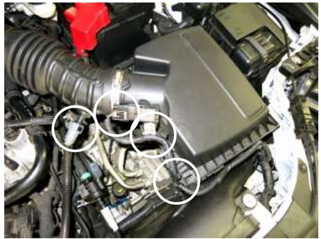
b. Disconnect the electrical connector, the two wiring harness connectors, and the vent tube on the stock intake.
