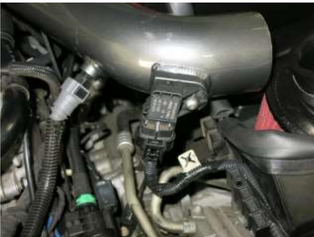
o. Install the electrical connector back onto the sensor that was removed in step 2b.
