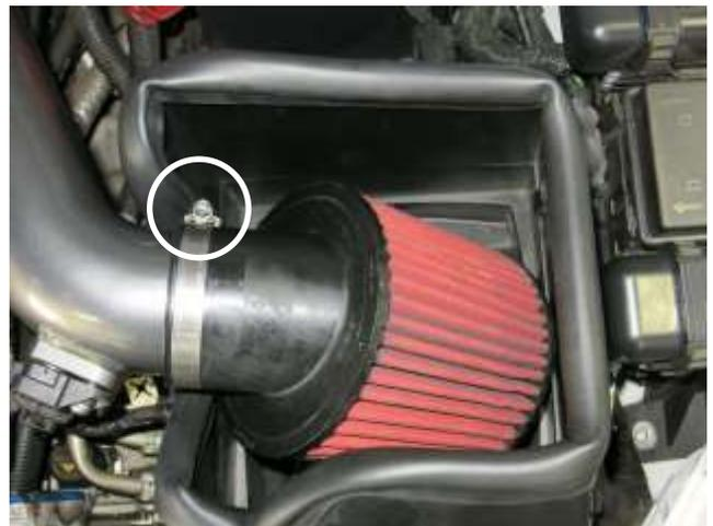
p. Attach the filter to the AEM intake tube and secure it with the hose clamp.
