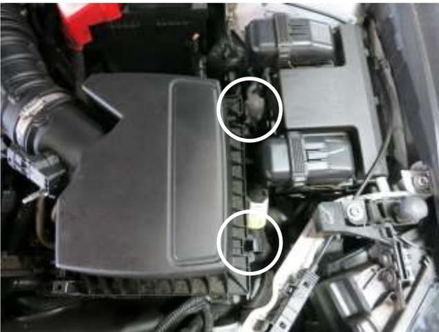
c. Unlatch the two clips that secure the upper to the lower air box.
