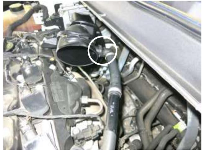
f. Squeeze to release the vent connector from the stock intake tube that leads to the turbo.
