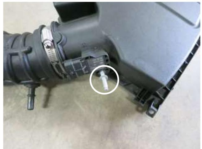
j. Using a E5 TORX socket remove the bolt securing the electrical sensor to the upper air box. This will be reused in step 3c.
