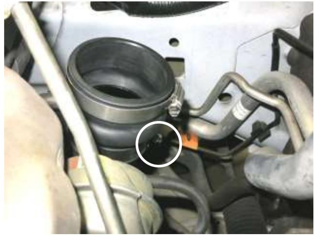
h. Install the hump hose onto the turbo compressor and tighten the clamp closest to the turbo at this time.
