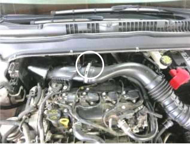
e. Loosen the hose clamp circled and remove the stock intake tube with the upper air box.
