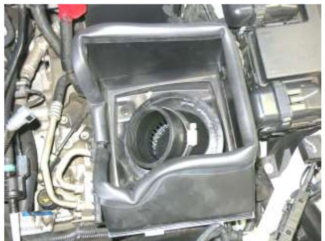
j. With the hose clamp on the filter loosely, lower the filter into the lower air box as shown.
