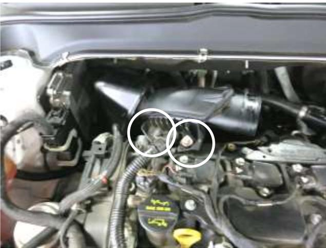
g. Loosen and remove the engine cover stand and the nut that are circled. The engine cover stand will be reinstalled in step 3r.
