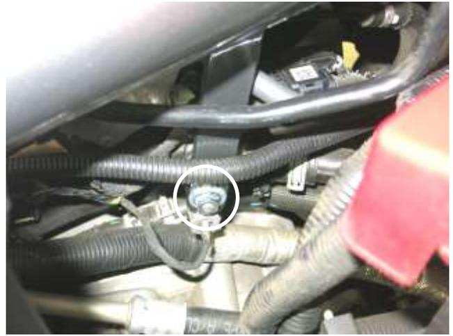
l. Once proper alignment is achieved, install and tighten the provided washer and nut onto the rubber bushing that was previously installed in step 3d.
