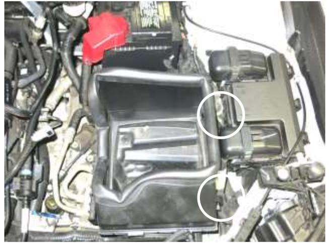
f. Place the assembled heat shield into the vehicles lower air box and secure with the clips that were unlatched in step 2c.
