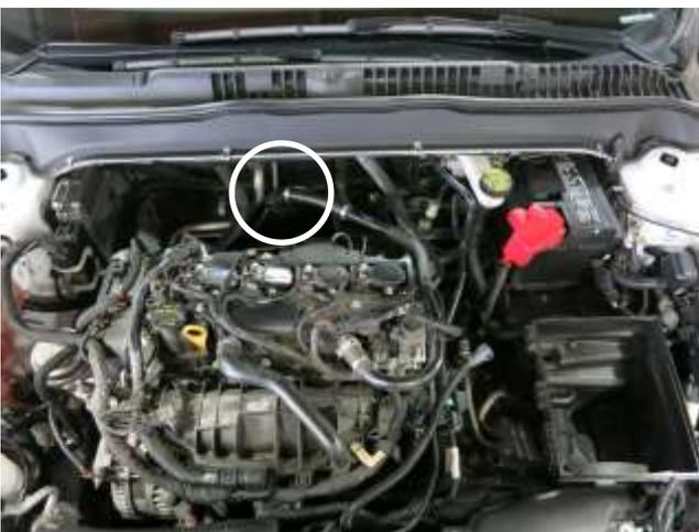
i. Using a pair of side cutters, cut the metal band that secures the fitting to the vent hose. Then, remove the fitting from the hose. The fitting will not be reused.
