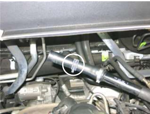
i. Install the provided spring clamp onto the vent line as shown.
