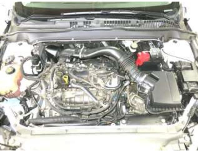
a. Remove the engine cover by pulling it up and out of the vehicle.
