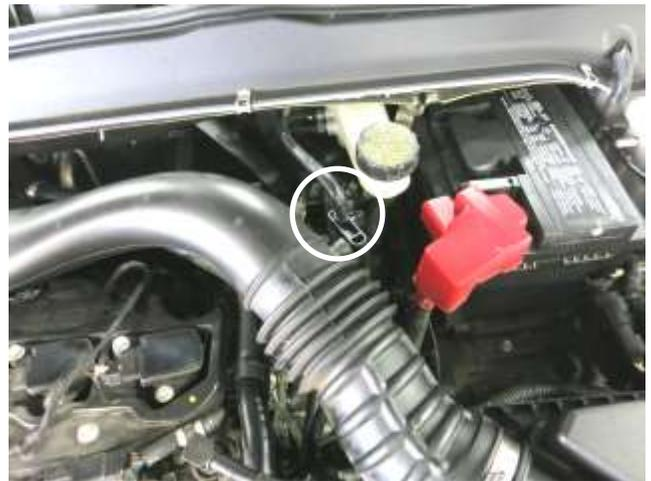
d. Unclip the vent line from the stock intake.
