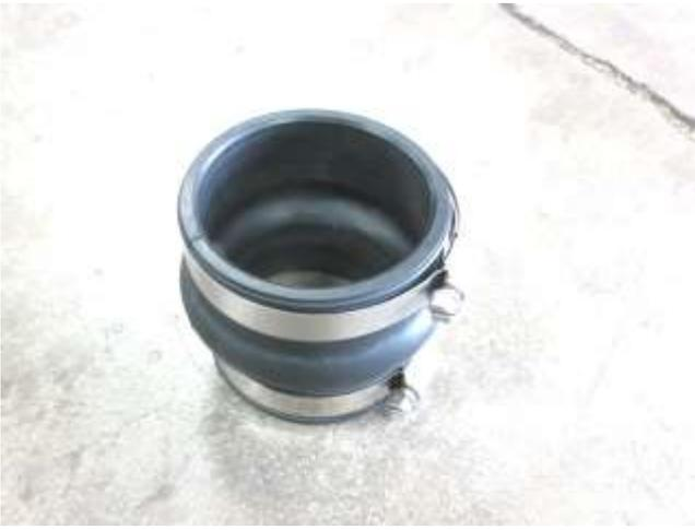
g. Place the two provided hose clamps onto the hump hose. Do not tighten them at this time.
