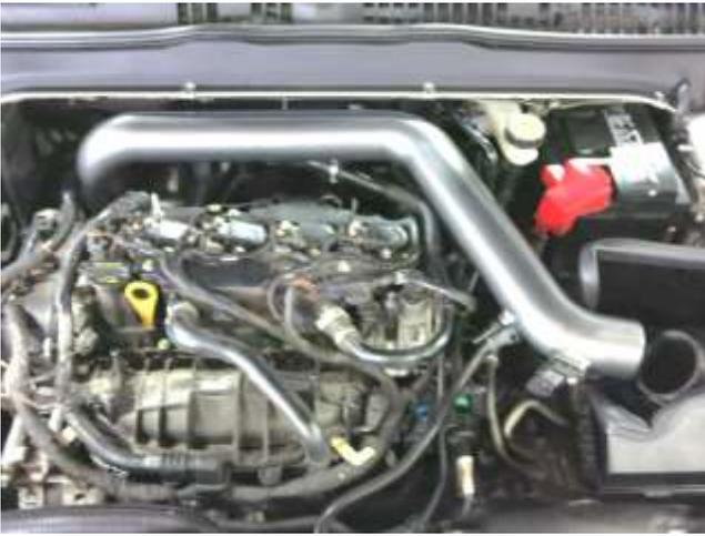
k. Install the AEM intake tube into the vehicle aligning the tube with the hump hose and the bracket to the rubber bushing.
