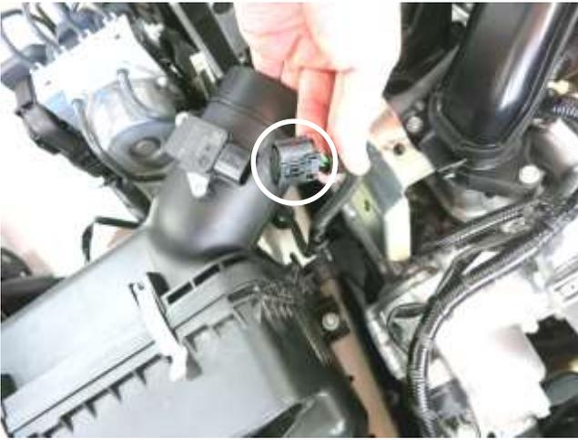
e. Depress the tab on the mass air sensor connector and disconnect it from the mass air sensor.
