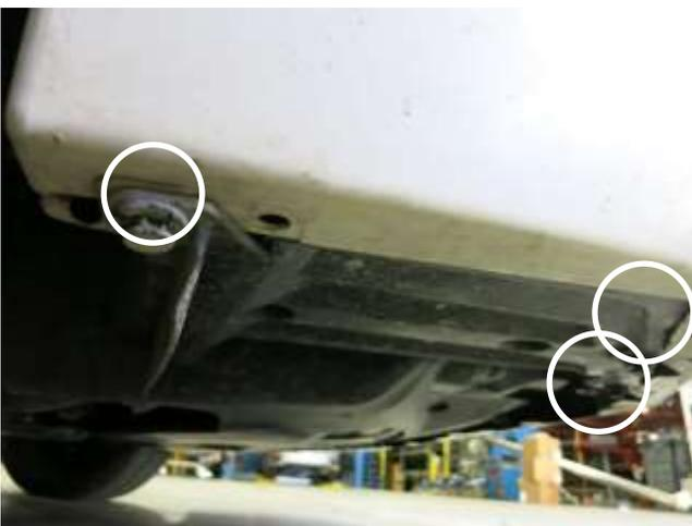
i. Remove the three clips securing the passenger side lower splash shield and pull the splash shield down.
