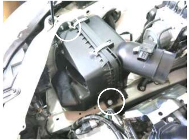
f. Remove the two nuts on the inner fender as well as the bolt on the lower air box. Then remove the air box from the vehicle. The nuts will be reused in step 3b. Note: Do not discard any of your stock equipment.
