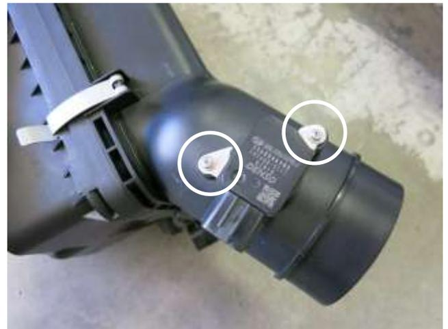
h. Remove the two screws securing the mass air sensor to the stock upper air box lid. Note: The screws will not be reused but the sensor will.
