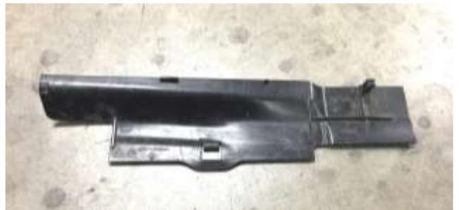
i. The inlet cover may now be removed through the emblem hole. It will look like the piece above. Replace the emblem at this time. Installation is reverse of removal.
