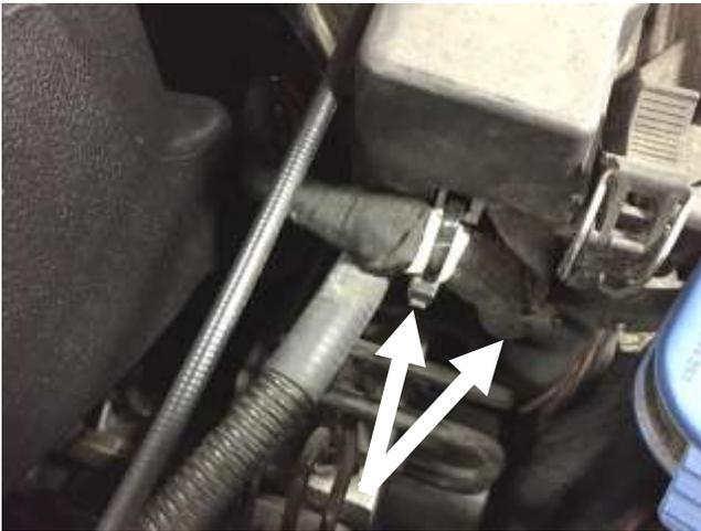
g. Cut the zip ties shown above to free the ECU harness. Take care to not cut the wiring.
