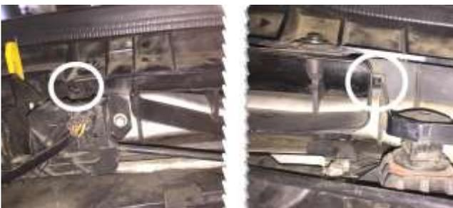
h. Release the inlet cover by squeezing and pushing the cover retainer tabs located on either side of the secondary inlet.
