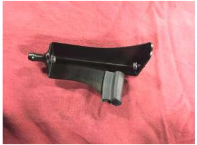
f. Install the 40mm trim piece on the airbox stand-off and assemble remaining components onto it as shown above.
