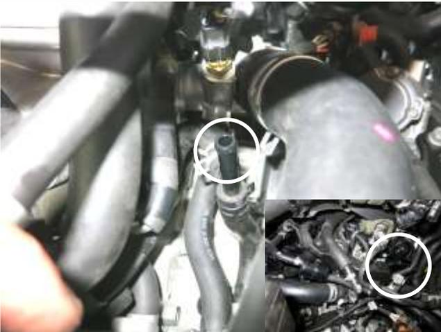
i. Route the previous hose above the "hard line" and too the "T" fitting. Connect the other end of the hose to the "T" fitting and secure with the spring clamp from step 2i. Then, with the two provided vacuum caps, cap the ends of the hard line.
