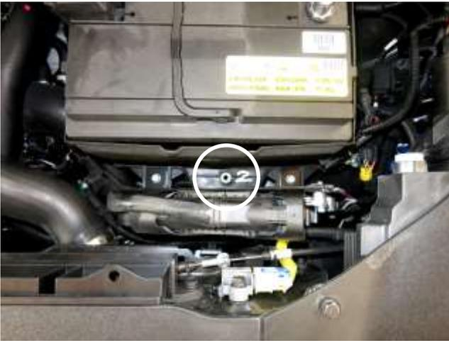
q. Re-center the battery in the tray and install the battery hold down with the bolt that was removed in step 2b.
