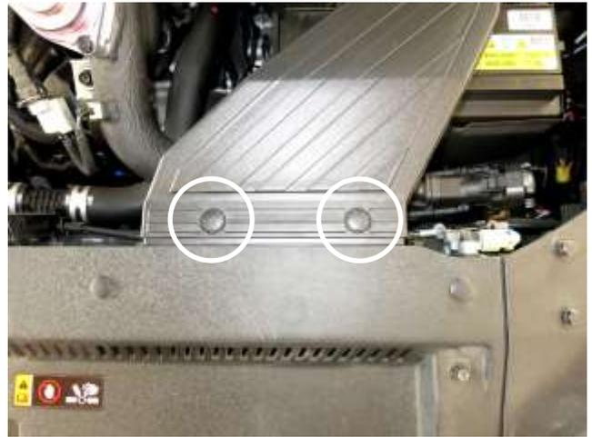
r. Install the stock scoop back into the vehicle with the clips that were removed in step 2a.
