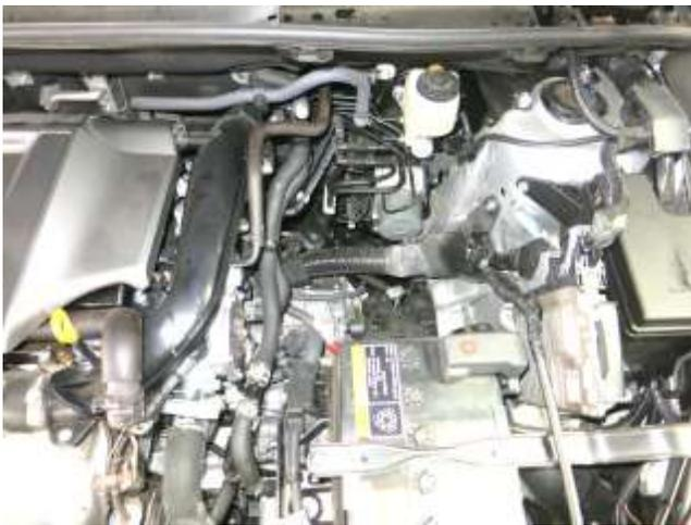
m. Remove the lower air box from the vehicle. **Note: Do not discard any of your stock equipment.**
