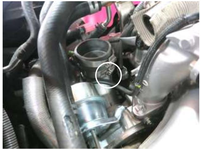
h. Install the hose and hose clamps onto the turbo compressor inlet. Tighten the hose clamp closest to the turbo at this time.
