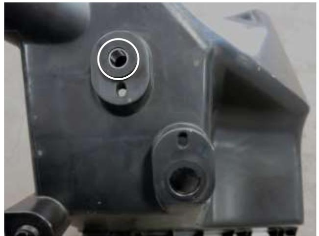
n. Turn the lower air box over and remove one of the metal sleeves and rubber grommet. The metal sleeve will be reused in step 3E.
