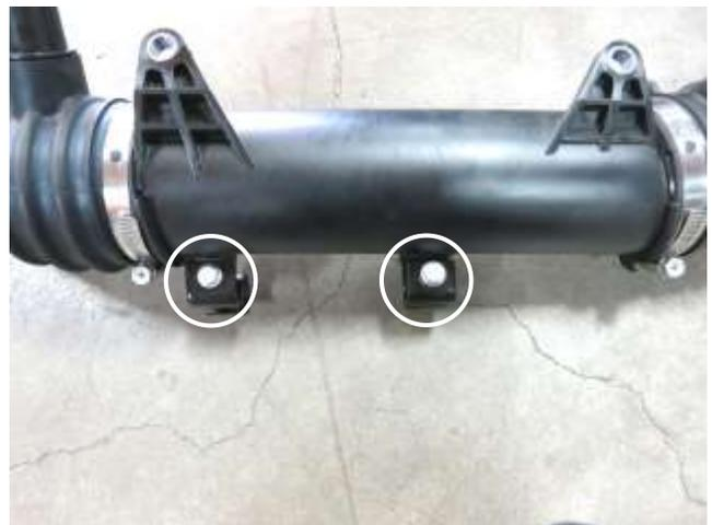
p. Remove the two bolts and stand offs. These will be reused in step 3c.
