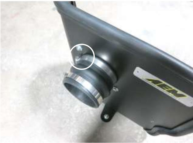
g. Install the hump hose onto the adapter with the provided hose clamps. Tighten the hose clamp closest to the heat shield at this time.
