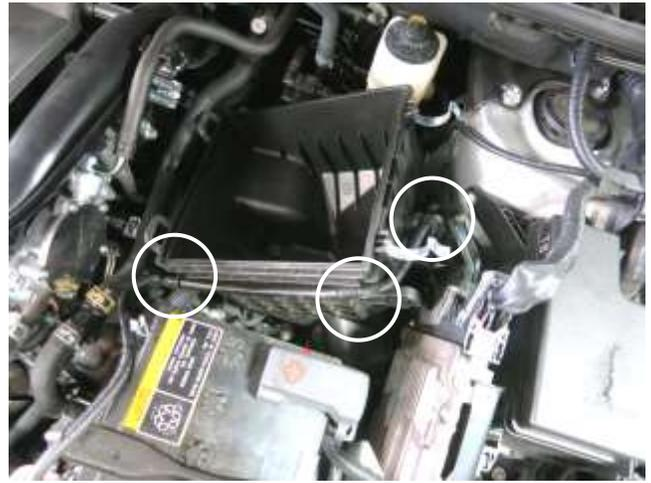
l. Maneuver the lower air box to access the three push-in wire harness clips and disconnect all of them.
