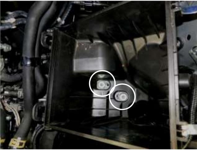
k. Remove the two bolts securing the lower air box to the vehicle. One bolt will be reused in step 3s.
