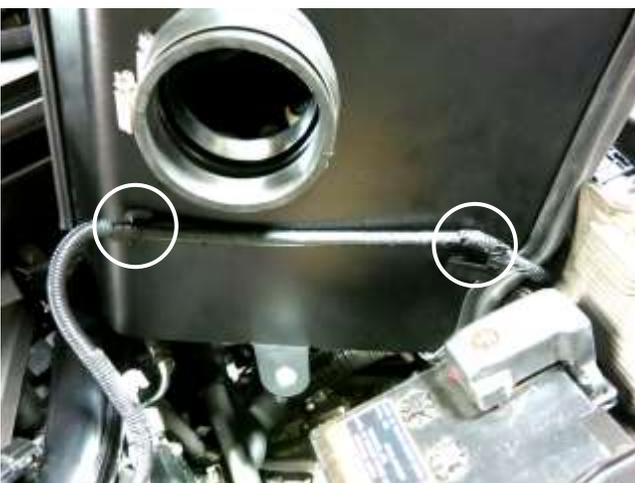
i. Secure the MAF sensor wiring harness onto the AEM heat shield via the stock clips. Then, lower the heat shield into the engine bay and press the air box mount into the stock grommet.
