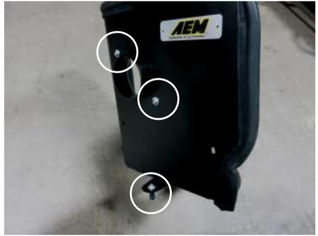
f. Assemble the adapter and air box mount with the provided hardware according to diagram on pg. 2.
