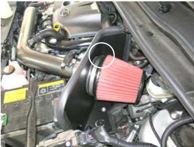
o. Install the AEM filter onto the filter adapter and tighten the hose clamp.
