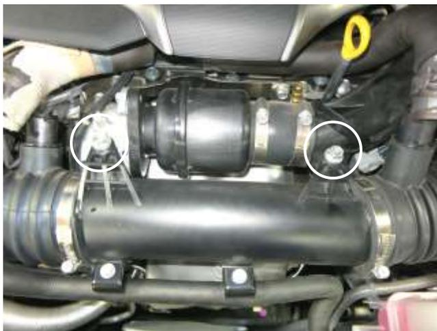
c. Loosen and remove the two bolts securing the stock intake tube to the vehicle.
