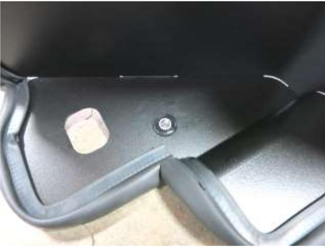
e. Take the sleeve that was removed in step 2n and install it into the grommet. **Note: A little soapy water will ease installation.**
