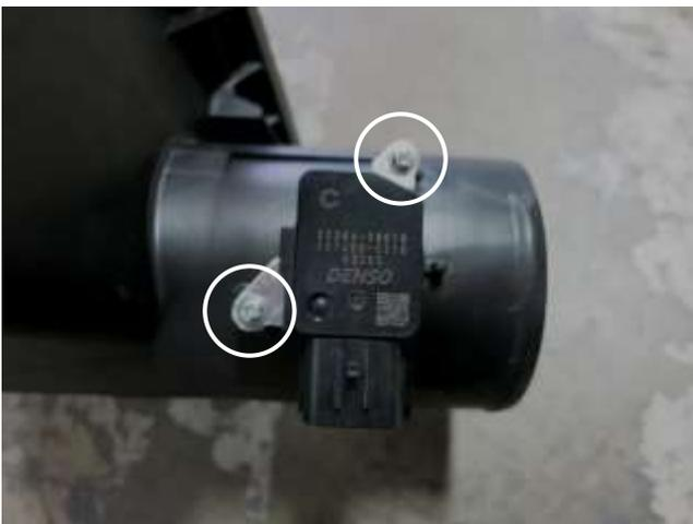
o. Remove the two screws that secure the MAF sensor to the upper air box. The MAF sensor will be reused in step 3b.
