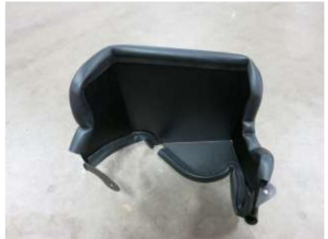
b. Install the edge trim onto the AEM heat shield as shown, trim to fit if desired.
