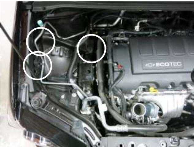
c. Remove the stock air intake. There are three push-in mounts securing the lower air box to the vehicle. Note: Do not discard any of your stock equipment.
