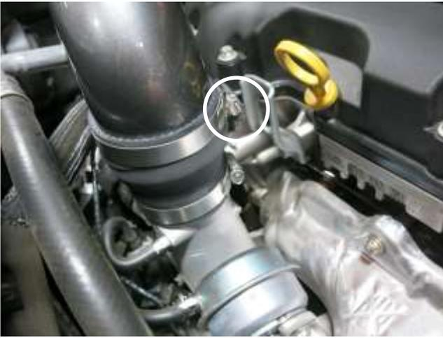
i. Install the AEM intake tube into the vehicle aligning the tube with the coupler. Tighten the hose clamp (circled above) at this time.
