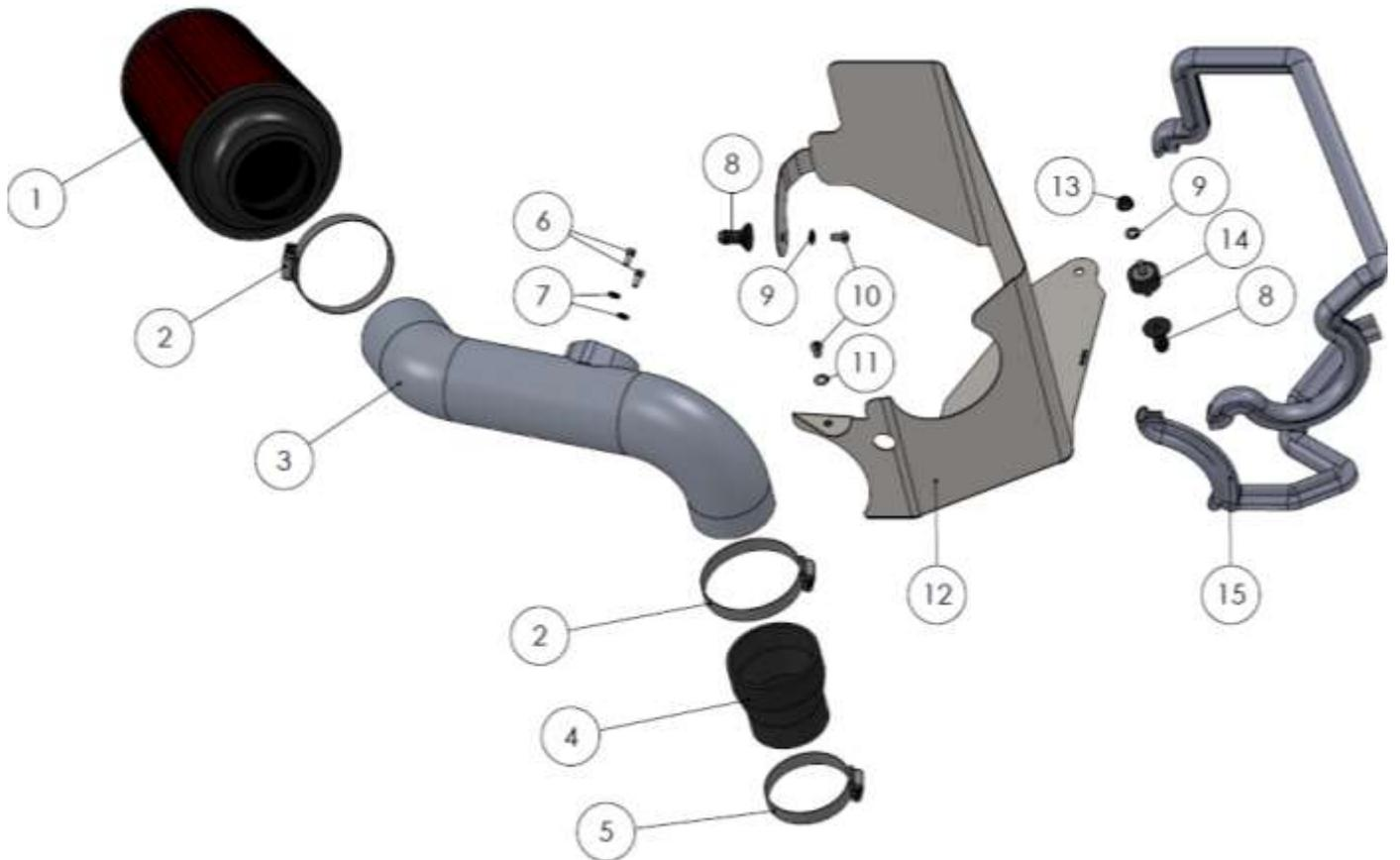
Read and understand these instructions **BEFORE** attempting to install this product. Failure to follow installation instructions and not using the provided hardware may damage the intake tube, throttle body and engine.
