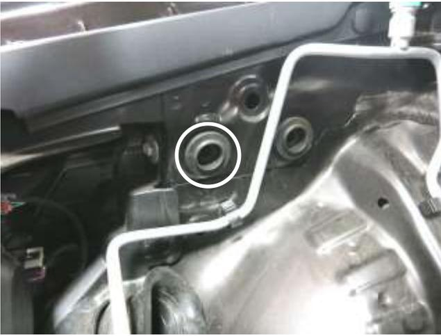
e. Remove the rubber grommet from the inner fender of the vehicle. This will be reused in step 3a.
