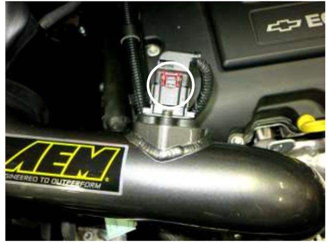
j. Reconnect the mass air sensor connector onto the mass air sensor. Engage the red locking tab.
