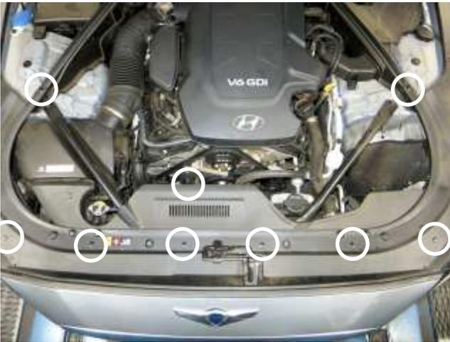
a. Remove the 13 plastic tabs that secure the engine bay cover by pushing down in the middle of the tabs, and then removing them. Note: Not all clips are shown in picture. Remove the cover.
