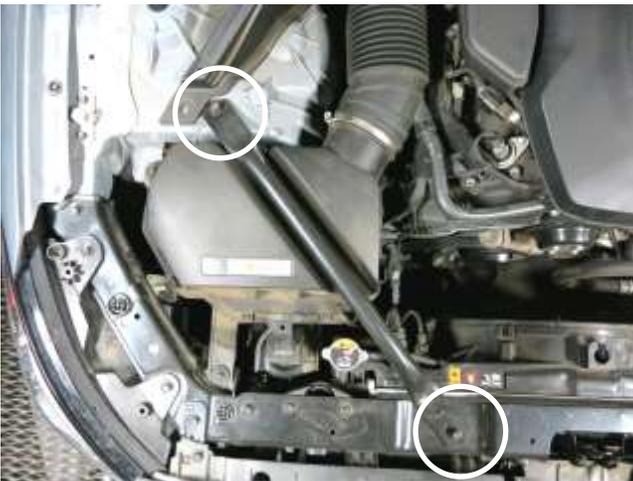
c. Remove the two bolts securing the brace to the vehicle. These will be reinstalled in step 3m.
