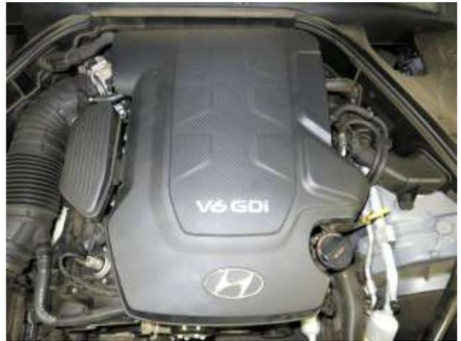
b. Remove the engine cover by pulling it up and out of the vehicle.
