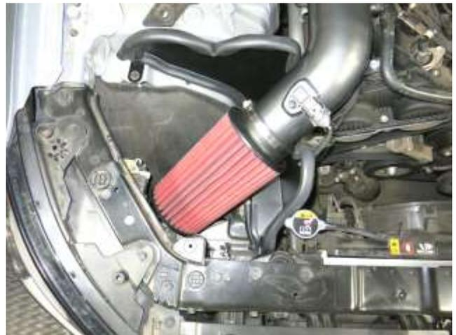
n. Install the AEM filter into the vehicle and onto the AEM intake tube. Tighten the provided hose clamp to 30 in-lbs.
