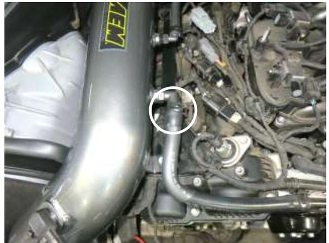
l. Install the vent line onto the AEM intake tube and secure with the spring clamp removed from step 2l.
