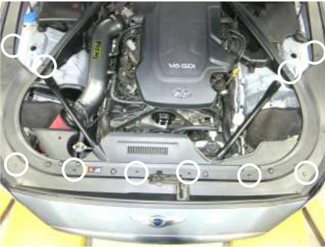
n. Reinstall the engine bay cover into the vehicle and secure with the clips removed in step 2a. Note: You will only use 12 of the clips (not all pictured)
