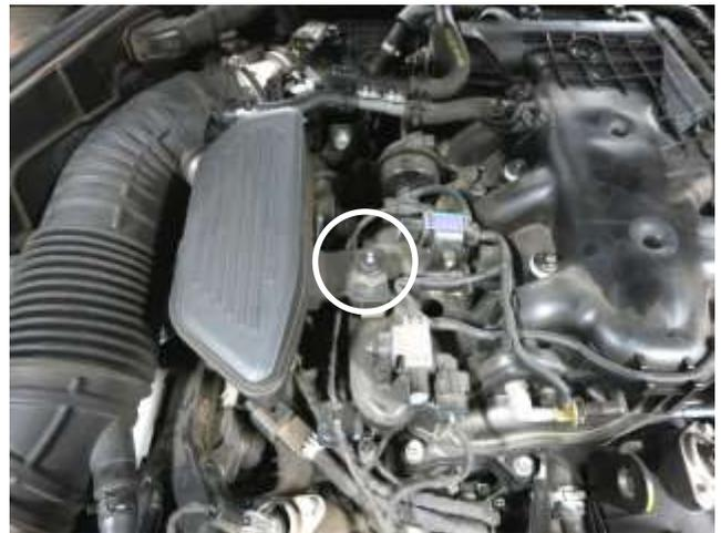
d. Remove the nut that secures the intake resonator to the engine. This nut will not be reused.
