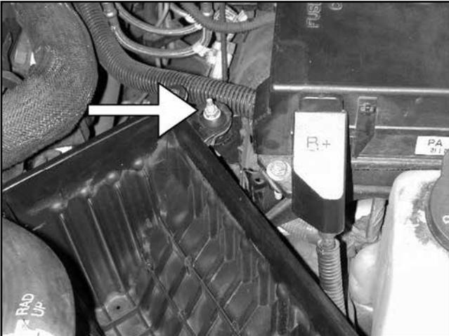
g. Remove the lower air box mounting nut. Remove the lower air box from the vehicle. Remove the lower air box mounting stud. This stud will be replaced with a rubber mount for the AEM® intake pipe later in the installation.
