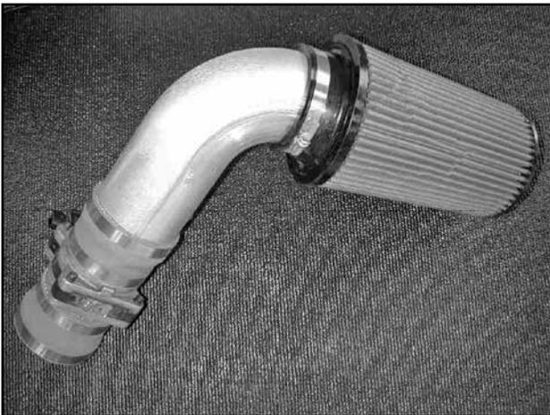
l. Install the AEM® air filter on to the end of the inlet pipe.
