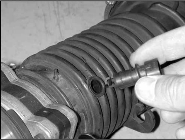
e. Remove the IAT sensor from the stock rubber intake tube. Set the sensor aside for use later in the installation.
