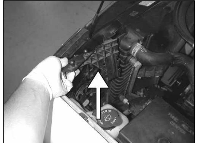
h. Remove the plastic air box mounting bracket located next to the radiator. The bracket is released by sliding it straight up.
