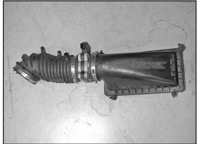
f. Loosen the hose clamps on either side of the MAF sensor. Remove the MAF sensor from the assembly and set aside in a safe place. Use care to avoid damaging the screen or any other part of the MAF sensor. The rubber gasket on the air box side of the MAF sensor will not be used with the AEM® intake.
