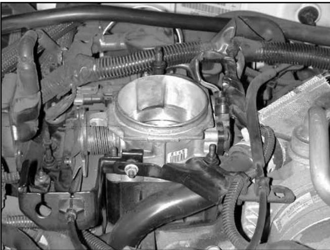
k. Remove the plastic throttle body adapter from the throttle body.
