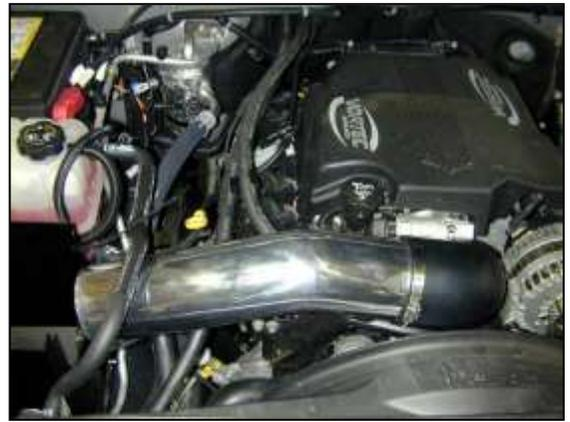
g. Slide the pipe into the rubber elbow and align the mounting bracket with the rubber mount previously installed on the heat shield.
