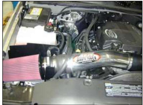
o. Tighten the hose clamps at the throttle body and silicone couplers. Tighten the nut on the mounting bracket. Re-adjust the intake pipe if necessary. Install rubber edge trim to the top of the heat shield and trim as necessary.
