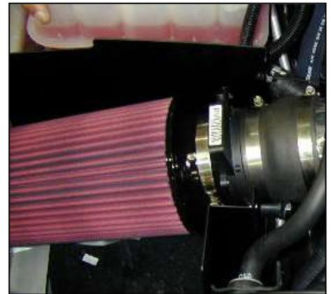
i. Securely attach the air filter to the MAF sensor using the supplied hose clamp (inlet side has the mesh screen). Securely attach the silicone coupler to the other side of the MAF sensor using the # 56 hose clamp.
