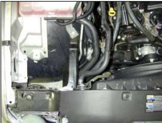
g. Stock airbox system removed from the vehicle.
