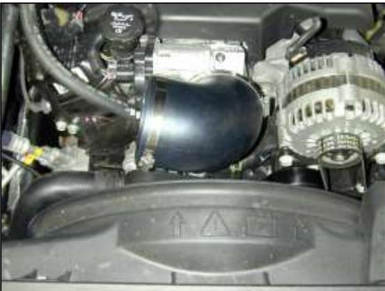
d. Install the supplied rubber elbow onto the throttle body using two #64 hose clamps. Do not fully tighten.
