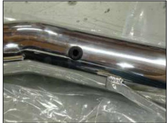
c. Install the rubber grommet into the hole in the intake pipe as shown.
