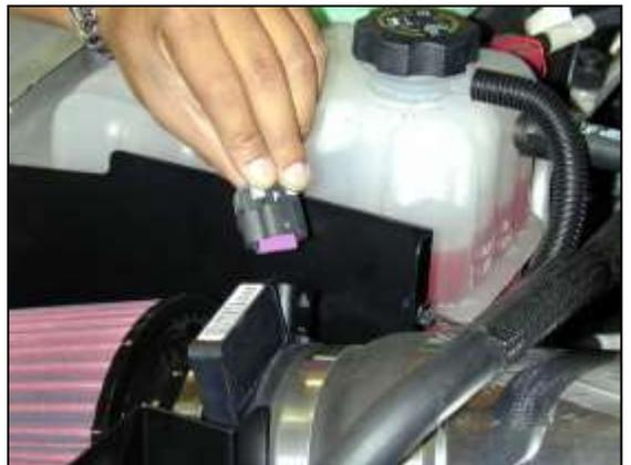
k. Rotate the MAF sensor so the plug is facing up as shown. Plug in the MAF sensor harness as shown. Use the zip tie to secure the harness out of the way and trim the excess.
