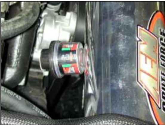
n. Install the air filter restriction gauge into the grommet installed in step 3c.
