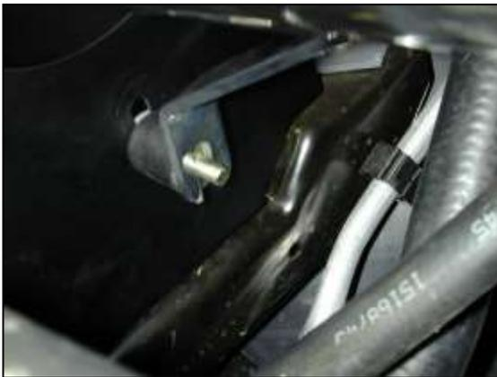
h. Attach the bracket to the rubber mount using the remaining washer and nylok nut. Do not tighten completely.
