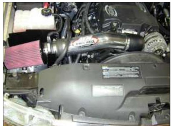
AEM® intake system installed
