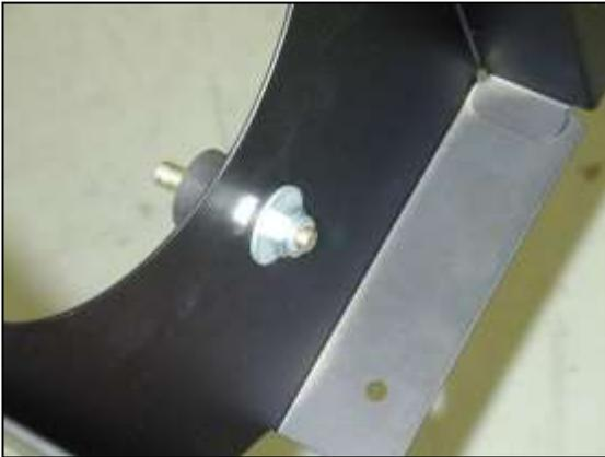
b. Install the supplied rubber mount onto the heat shield as shown using one washer and one nylok nut. Do not fully tighten. It is helpful to run both supplied nylok nuts down the threads once before assembly to make installation easier.
