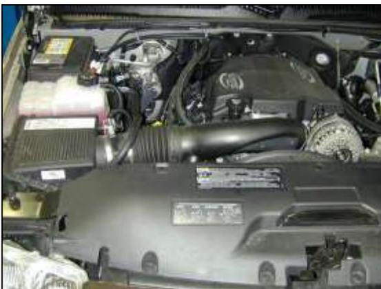
Factory airbox system installed.
