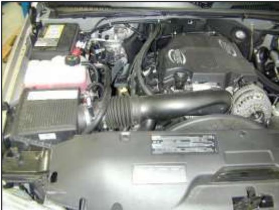
a. Factory airbox system installed.
