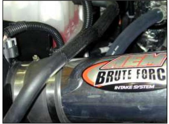
m. The reservoir hose should clear the intake pipe as shown.
