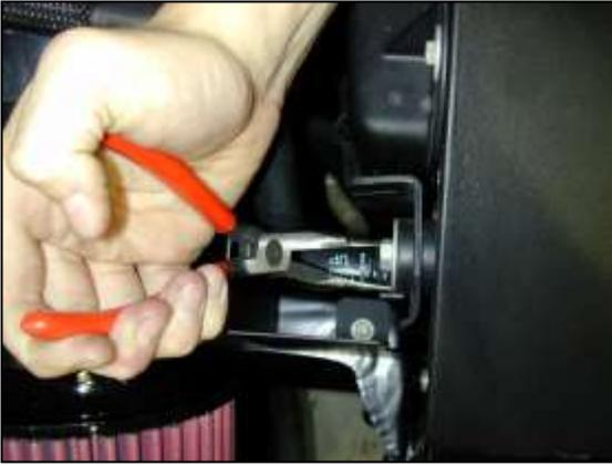
l. Use a pair of pliers and compress the clamp holding the coolant reservoir hose to the radiator. While compressed, rotate the hose up and away from the intake pipe.
