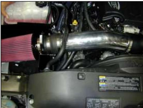
j. Attach the air filter assembly to the intake pipe by sliding the silicone coupler over the intake pipe end. Secure with a supplied #64 hose clamp. Ensure that the air filter does not make contact with any part of the vehicle.
