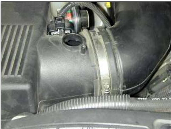
c. Loosen the hose clamp at the air box side of the air intake tube.
