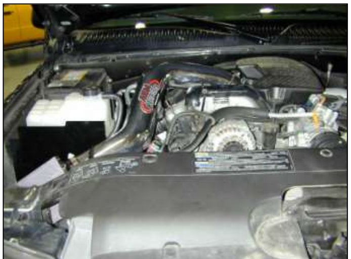
AEM® intake system installed
