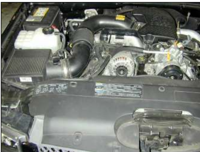
Factory air box system installed
