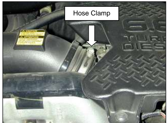
d. Loosen the hose clamp at the turbo inlet side of the air intake tube. Remove the air intake tube from the engine bay.
