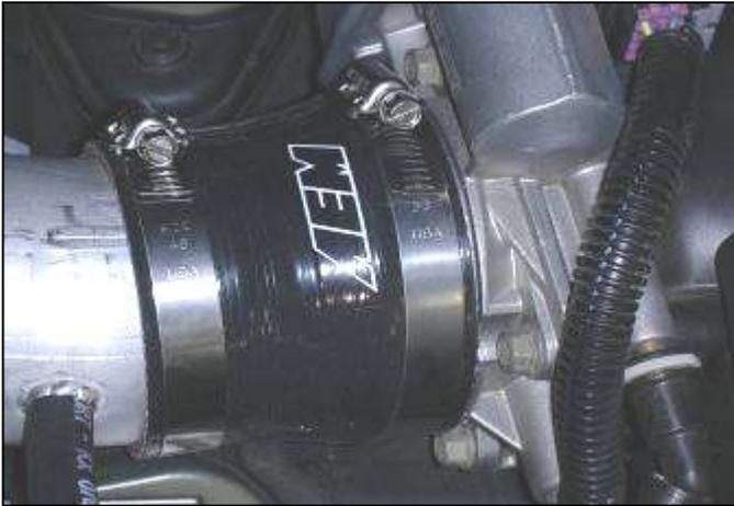
f. Slide the bracket side of the pipe through the heat shield hole. Align the coupler with the throttle body and secure using the #52 hose clamp.
