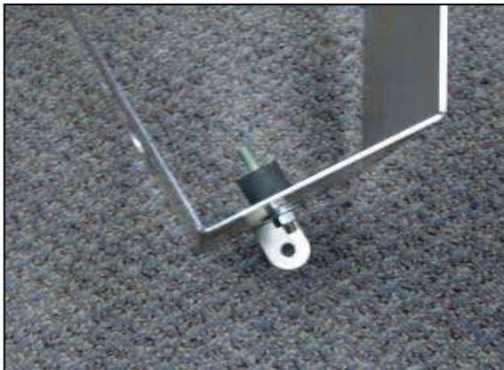
b. Install the supplied rubber mount on to the AEM® heat shield using one each of the supplied washers and locknuts.
