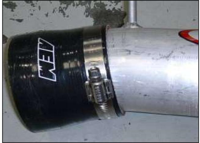
e. Install the reducing coupler on the end of the intake pipe using the #48 hose clamp.
