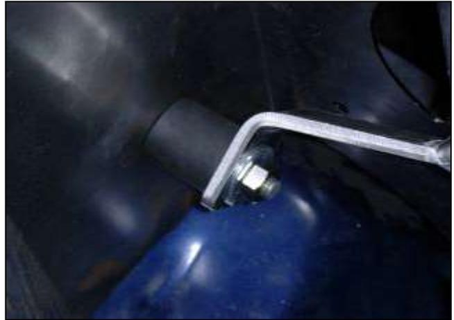
g. Align the intake pipe bracket with the rubber mount on the heat shield. Use the supplied washer and nylok nut to partially secure.
