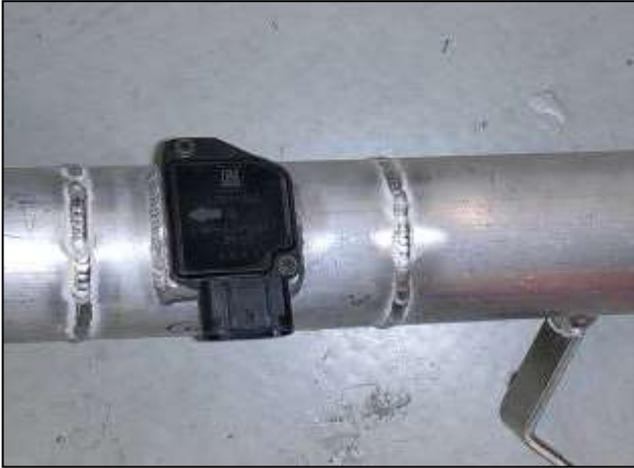
d. Install the MAF Sensor using the original mounting screws. Use caution to avoid damaging the o-ring.
