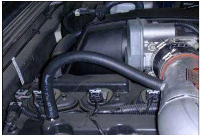
i. Attach the supplied 1/2" hose between the intake pipe and the valve cover as shown. Trim to fit and secure using the supplied hose clamps.
