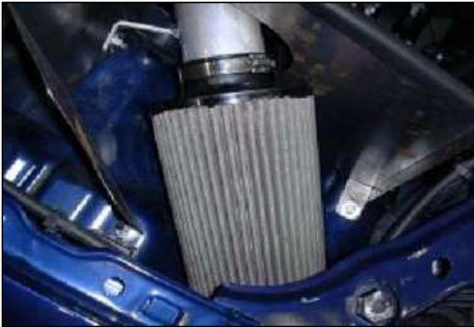
h. Check to be sure that the AEM<sup>®</sup> air filter is clear from and debris. Attach the air filter to the end of the AEM<sup>®</sup> intake pipe as shown.
