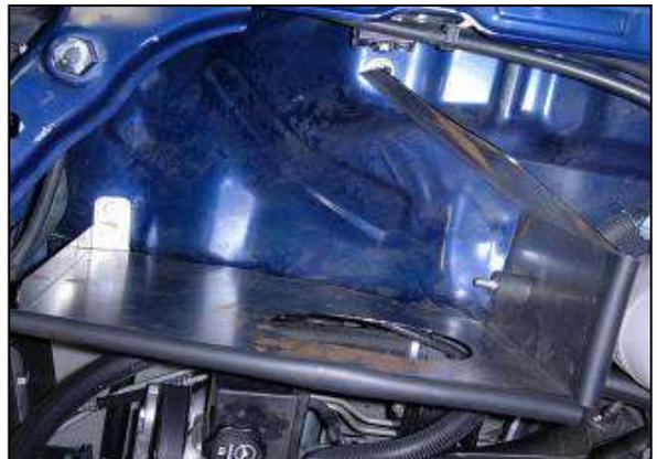
c. Install the AEM® heat shield using the two supplied bolts and washers and the original air box mounting nut. Install rubber edge trim to the top of the heat shield.
