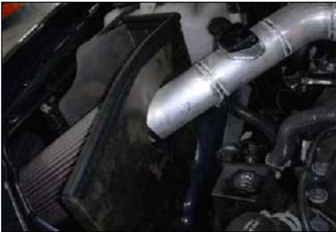
I. Position the AEM® intake for best fitment. Be sure that the pipe or any other component is not in contact with any part of the vehicle. Tighten the hose clamps at the throttle body. Tighten the nut on the mounting bracket. Re-adjust pipe if necessary. Re-connect the MAF wire harness.
