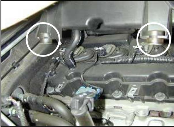
e. Remove the two bolts on the air resonator. Lift the resonator up and remove the breather hose from the valve cover. Remove the small breather hose from the front of the resonator and remove the resonator.
