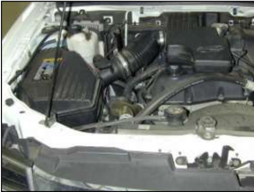
a. Factory airbox system installed.
