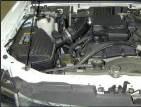
a. Factory airbox system installed.
