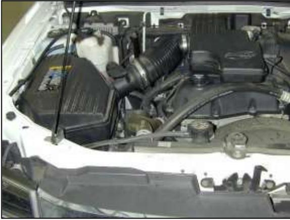
Factory airbox system installed.
