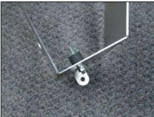
b. Install the supplied rubber mount onto the AEM<sup>®</sup> heat shield using a washer and locknut as shown.
