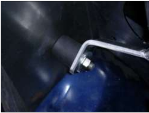
g. Align the intake pipe bracket with the rubber mount on the heat shield. Use the supplied washer and Nylock nut to secure (Do not tighten).
