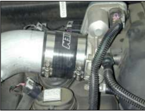
f. Slide the bracket side of the intake pipe through the heat shield hole. Insert the nipple side of the intake pipe into the 3" silicone hose on the throttle body.
