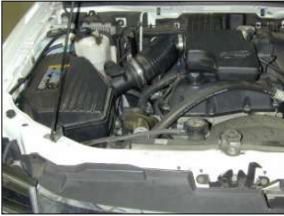
Factory airbox system installed.
