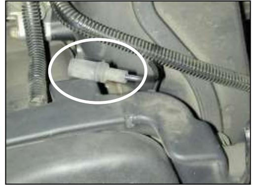
f. Remove the rubber breather hose adapter plug from the hard plastic breather hose by gently pulling it off while holding the hard plastic line.
