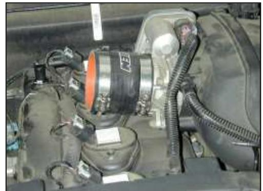
e. Install the 3" silicone hose onto the throttle body; secure using the #48 hose clamp. Install the remaining #48 hose clamp onto the opposite end.
