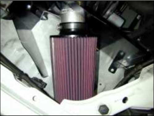
h. Ensure the AEM ® air filter is clear of debris. Attach the air filter onto the end of the AEM ® intake pipe and secure with a hose clamp as shown.
