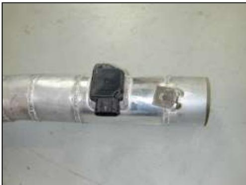
d. Install the MAF sensor using the stock mounting screws. Use caution to avoid damaging the o-ring.
