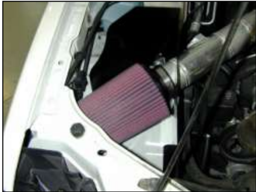
k. Tighten the hose clamps at the throttle body. Tighten the nut on the mounting bracket. Re-adjust the intake pipe if necessary. Plug the MAF sensor harness into the sensor.
