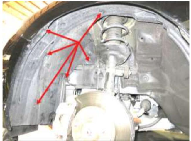
h. Using a flat screw driver, disconnect the six trim panel clips shown above. Disconnect by inserting screwdriver
