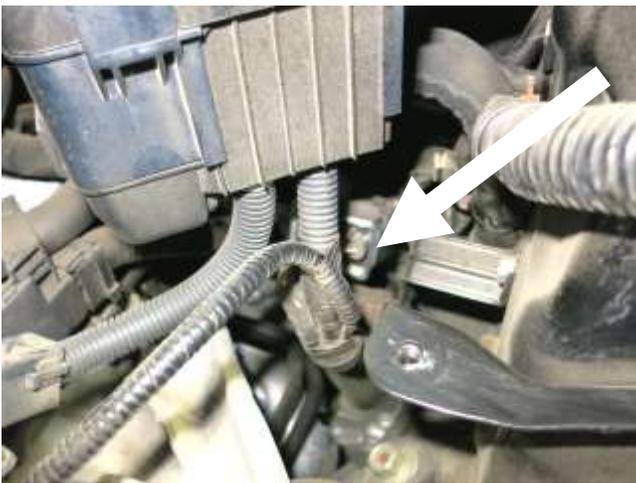
g. Remove the electrical tape that holds the MAF harness to the main wire harness.
