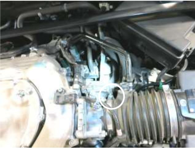
e. Loosen the hose clamp at the throttle body and remove the intake duct from the throttle body.
