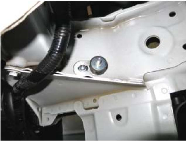
e. Install the rubber mount onto the provided bracket & install the bracket into the vehicle, then secure the screw to the wellnut. Align the AEM intake tube bracket with the mount & secure with provided washer & nut.
