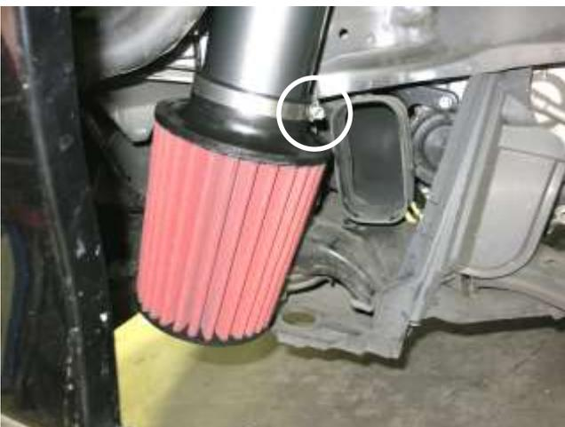
i. Install the AEM filter onto the AEM tube and secure with the provided hose clamp to 30 in-lbs.
