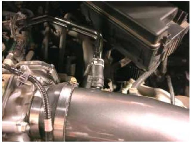
f. Install the provided hose and spring clamp onto the AEM intake tube. Install the vent line into the hose and secure the spring clamp that was removed in step 2c. Note: Trim hose to fit.
