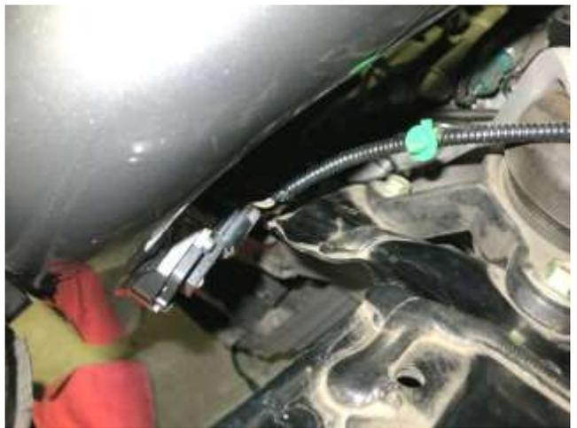
h. Plug the MAF connector back into the MAF sensor on the AEM intake tube.
