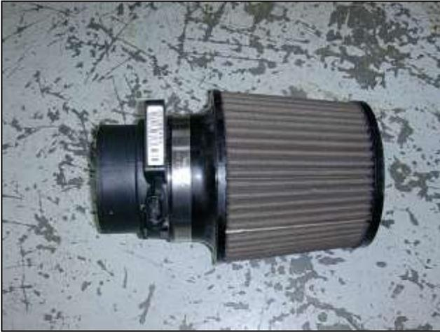
n. Install the AEM<sup>®</sup> air filter on to the end of the MAF Sensor housing. Push the air filter over the inlet pipe until the stop in the filter is reached; then install one hose clamp to secure the air filter.
