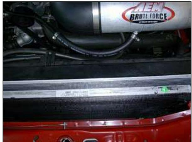
q. Install the supplied 3/8" hose between the plastic breather hose and the aluminum nipple on the intake pipe. Secure using two 3/4" hose clamps.
