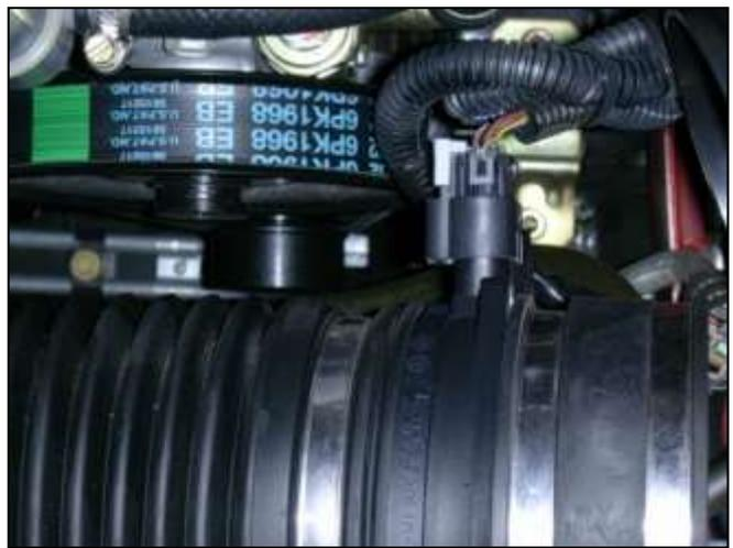
d. Unplug the MAF sensor harness from the MAF sensor and remove the stock inlet air hose and sensor.
