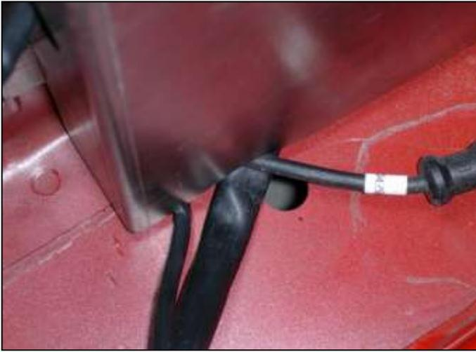
f. Be sure to have the wires run under the heat shield where the cut out on the bottom is located.
