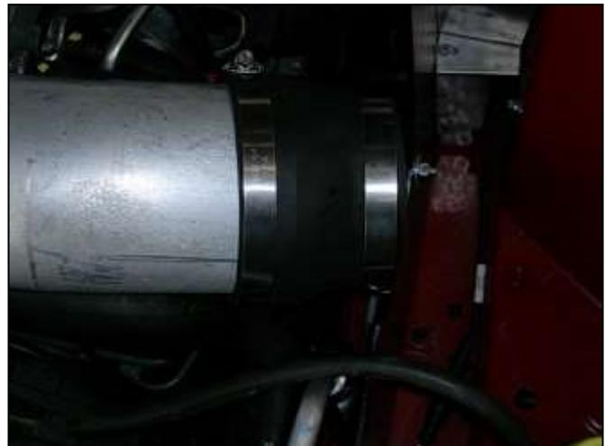
m. Install the reducer coupler onto the smaller side (black plastic) of the MAF sensor housing using a #64 hose clamp to secure.
