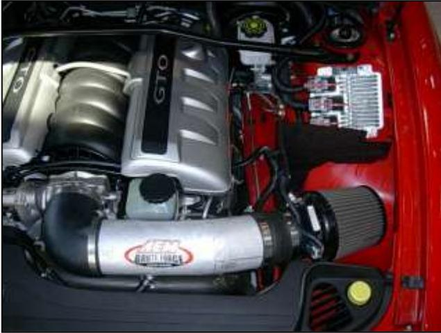
r. Reinstall the radiator shroud and check that the air filter is not touching any part of the vehicle.
