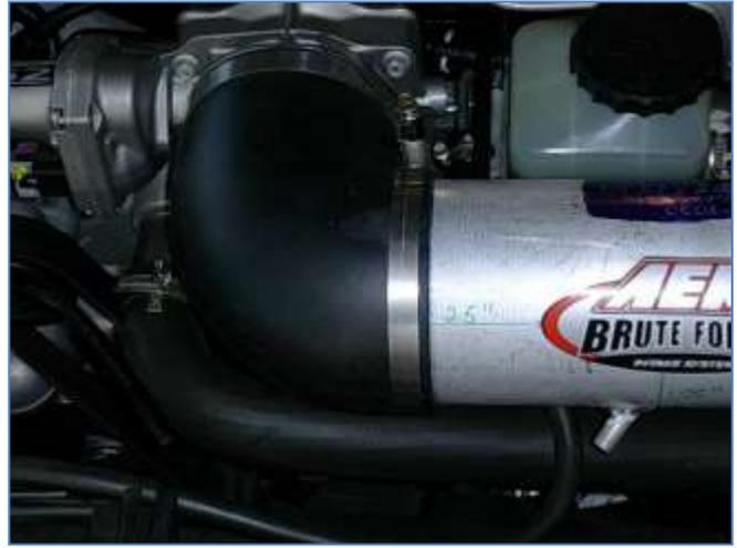
k. Check to be sure the upper intake pipe is clear of any debris. Install the intake pipe by sliding it into the coupler attached to the throttle body.
