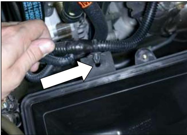
g. Detach the wiring harness air filter housing as shown.
