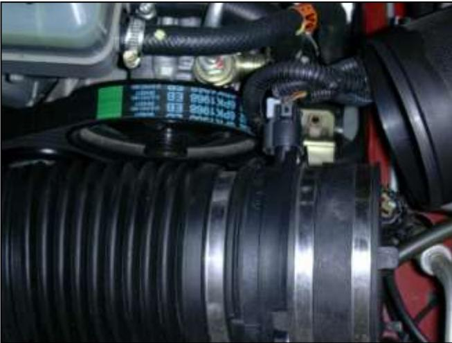
e. Remove the MAF sensor from the inlet hose and set aside. Be careful not to damage the MAF sensor.
