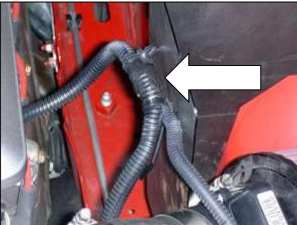
p. Install the supplied heat shield zip-tie into the hole and secure the MAF sensor wiring harness.
