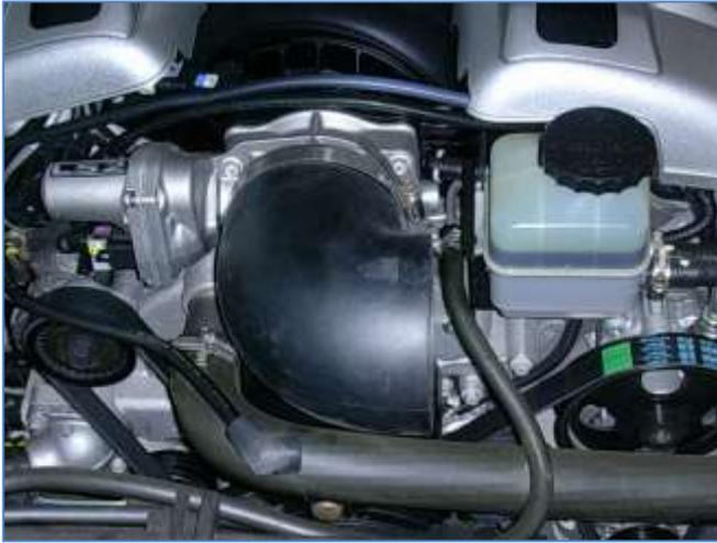
j. Install the long end of the rubber elbow over the throttle body using the supplied #64 hose clamps.
