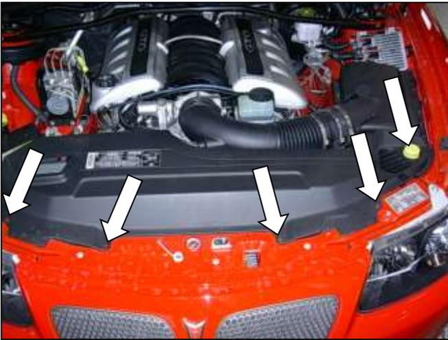
a. Remove the radiator shroud from the front of the vehicle by removing the 5 plastic connectors.
