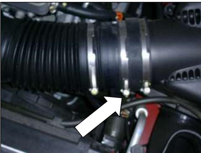
c. Loosen the hose clamp on the Mass Air Flow Sensor (MAF) and remove the inlet hose from the air filter housing. Rotate the inlet hose to expose the MAF sensor plug and harness.
