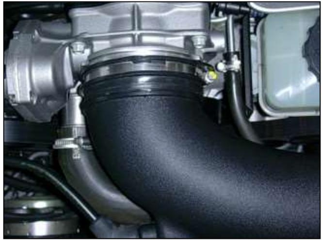
b. Loosen the hose clamp on the inlet hose elbow attached to the throttle body.
