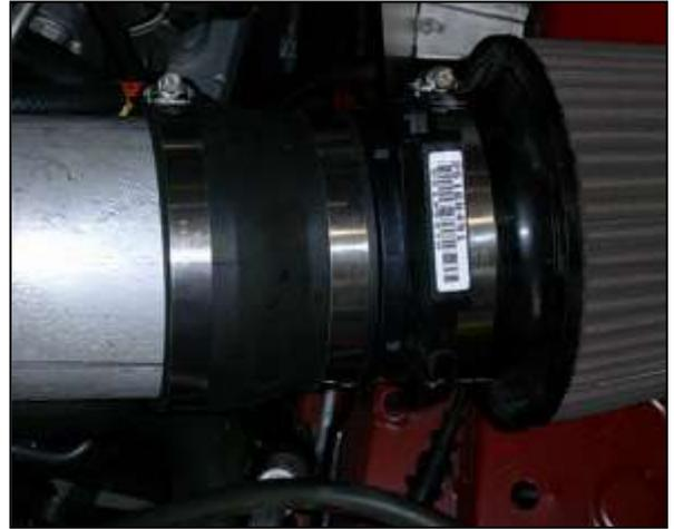
o. Install the MAF sensor and filter into the previously installed reducer coupler. Plug in the MAF sensor and secure the unit using the #56 hose clamp.
