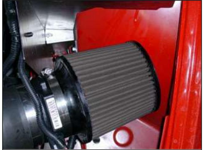
s. Position the AEM® intake for best fitment. Be sure that the pipe or any other component is not in contact with any part of the vehicle. Tighten the hose clamps at the throttle body and silicone coupling. Tighten the nut on the mounting bracket. Re-adjust pipe if necessary.
