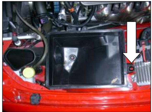
h. The lower air box is held in place with three grommets. To remove it, simply lift up on the box near the ECU.
