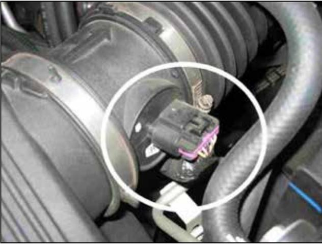
e. Disconnect the mass air flow sensor wire, and loosen the hose clamp securing the MAF housing to the stock inlet tube.
