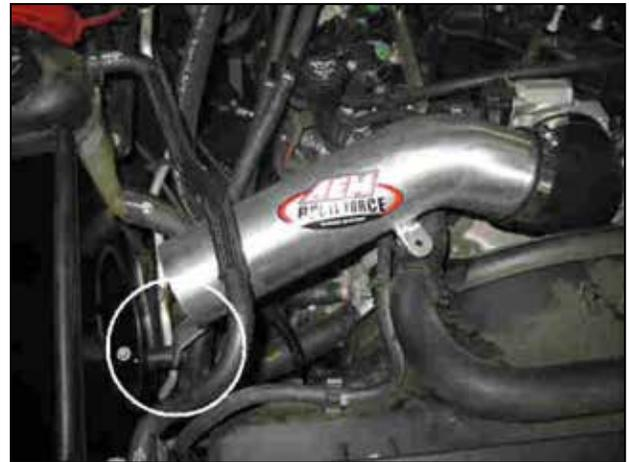
e. Insert intake pipe into elbow located at the throttle body. Secure the bracket to the rubber mount on the heatshield.
