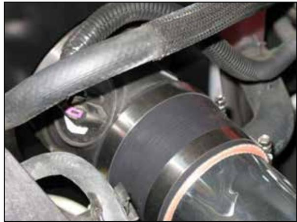
g. Then attach the assembly made in step 3g. to the end of the intake pipe. Reconnect the MAF sensor wire.
