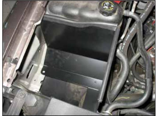
b. On the heat shield, install rubber mount using the supplied washer and nut. Install "8-3018" rubber edge trim around intake pipe opening. Install 8-4011 and 8-4012 edge trim to top edge of the heat shield.
