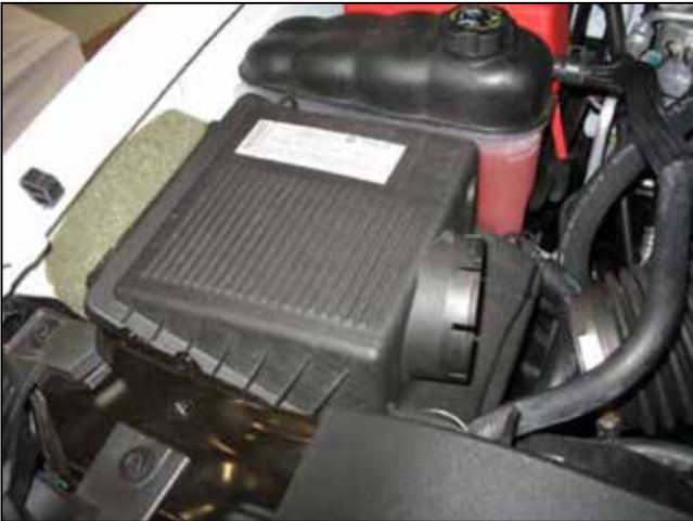
g. Pull the stock air filter housing straight up out of the vehicle.
