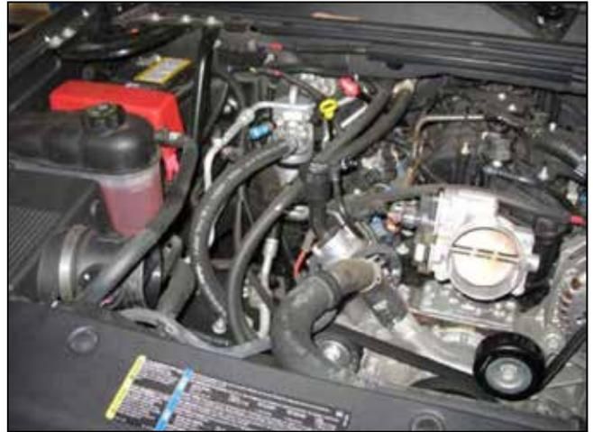
f. Pull the stock inlet tube out of the vehicle. Loosen the hose clamp securing the MAF housing to the air filter, remove MAF housing, keep for later reuse.
