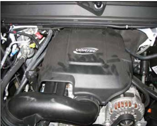
Factory air box system installed
