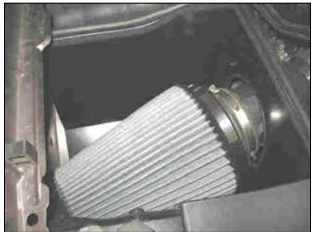
i. Install air filter assembly into the stock MAF rubber coupler.
