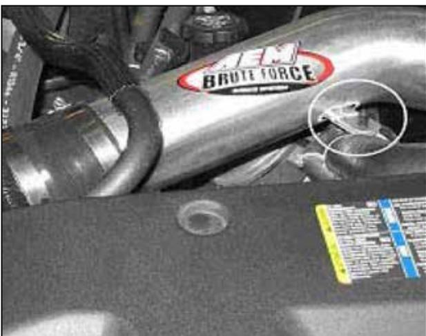
j. Use the stock plastic radiator clamp to secure the radiator hose away from the intake pipe. By inserting it into the bracket located on the pipe.
