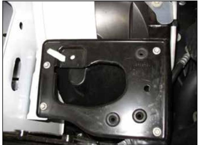
h. Remove the four bolts securing the stock air box mounting plate.
