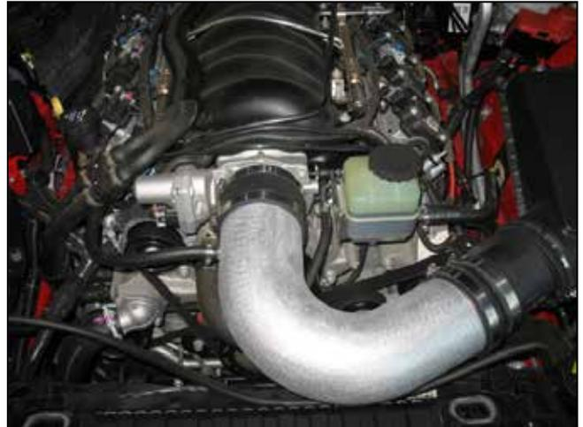
c. Slide coupler over MAF body, then the elbow over the throttle body, align inlet and secure the hose clamps.
