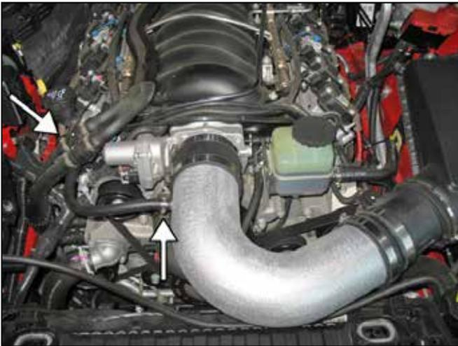
d. Route the breather hose around pulley and under AC lines.
