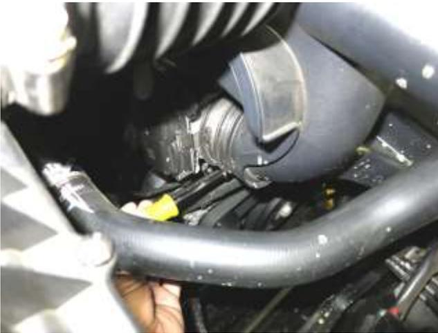
c. Loosen the hose clamp securing the upper resonator to the throttle.
