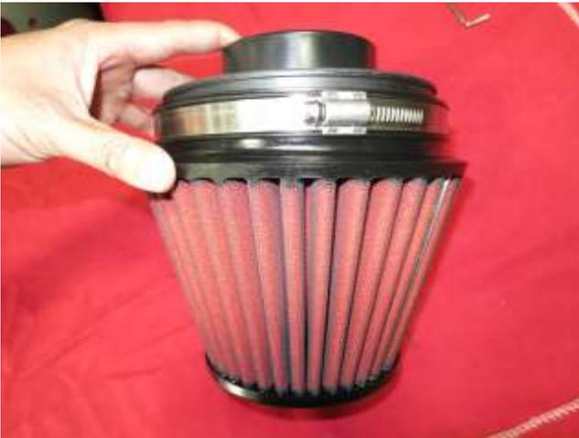
c. Insert the filter adapter(21512-1) into the filter(AEM-21-209D)and fasten with the hose clamp(AEM-94104) provided.
