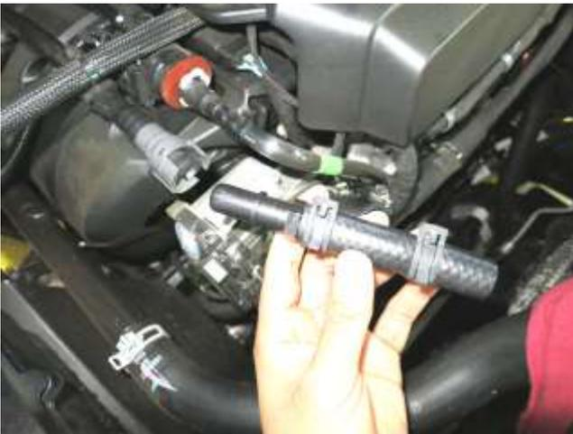
g. Assemble the hose(087028) with the spring clamps (08553) and quick disconnect nipple(082628) provided.
