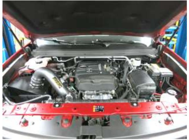
l. Finished installation of AEM Intake System.
