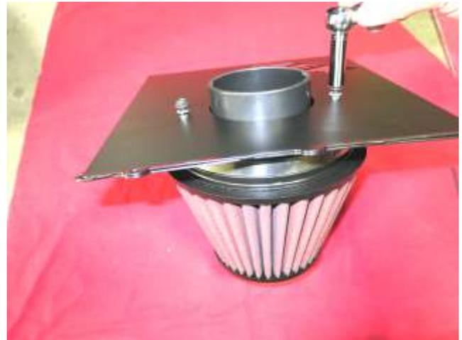
d. Fasten the adapter to the heat shield(AEM-20-8552) using the crush washers(AEM-1-3025) and m6 bolts (AEM-1-2110) provided.
