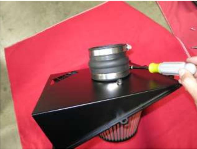
e. Install the hump hose(08657) and fasten it to the adapter using the hose clamp(AEM-9456). Slide hose clamp(AEM-9452) onto the other end.
