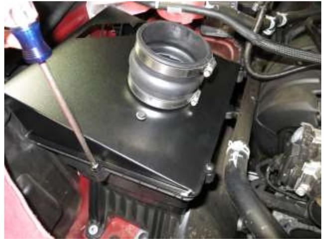
f. Fasten the heat shield to the stock lower airbox using the 4 screws(AEM-1-1020) provided.
