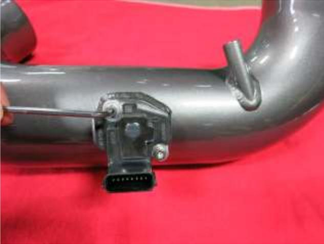
a. Use the provided bolts(07733) to install the MAF sensor into the AEM tube(AEM-2-1533C).
