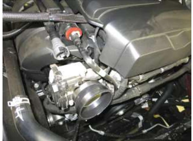
b. Install the coupler(084034) and hose clamps(AEM-9444 and AEM-9452) onto the throttle.
