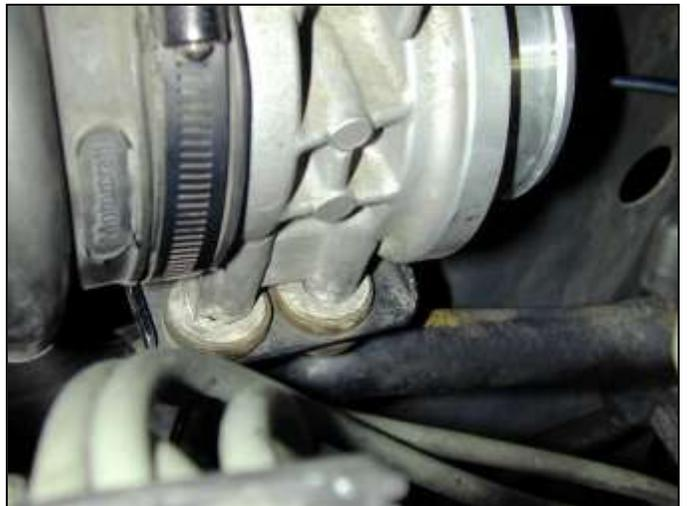
d. Loosen the two remaining bolts on the opposite side of the MAF sensor and remove.
