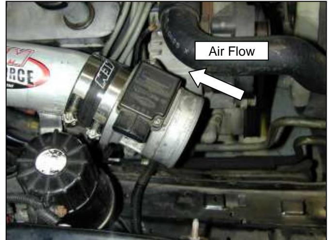
g. Attach the coupler to the inlet pipe and secure with hose clamps. Insert the MAF sensor.
