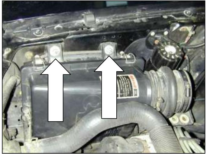
f. Loosen and remove the remaining two nuts on the air box. Remove the air box.
