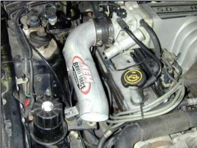
f. Insert inlet pipe and align with the rubber mount. Secure the inlet pipe onto the rubber mount with provided washer and nylok nut.
