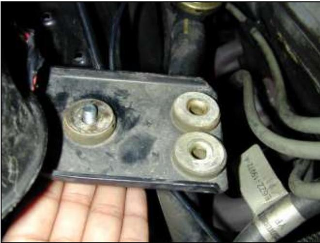
d. Insert the bolt and washer into the hole in the MAF sensor bracket.
