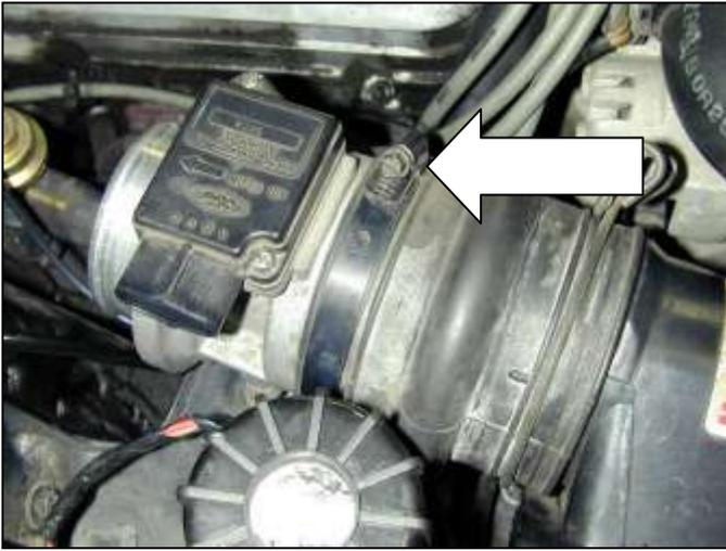
e. Loosen hose clamp and remove MAF sensor. Be careful not to damage sensor or screen.
