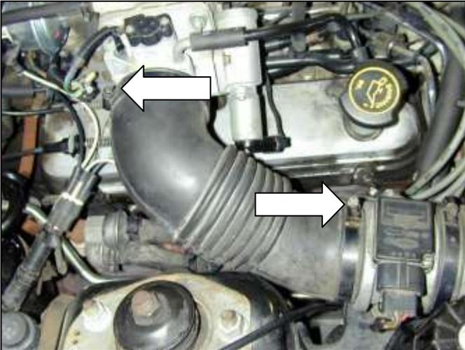
a. Loosen the hose clamp on the intake tube at the throttle body and also at the mass airflow sensor (MAF). Remove inlet tube.
