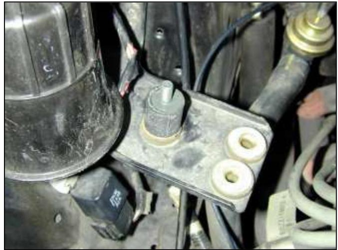
e. Tighten the female end of the rubber mount to the bolt in step 3c.
