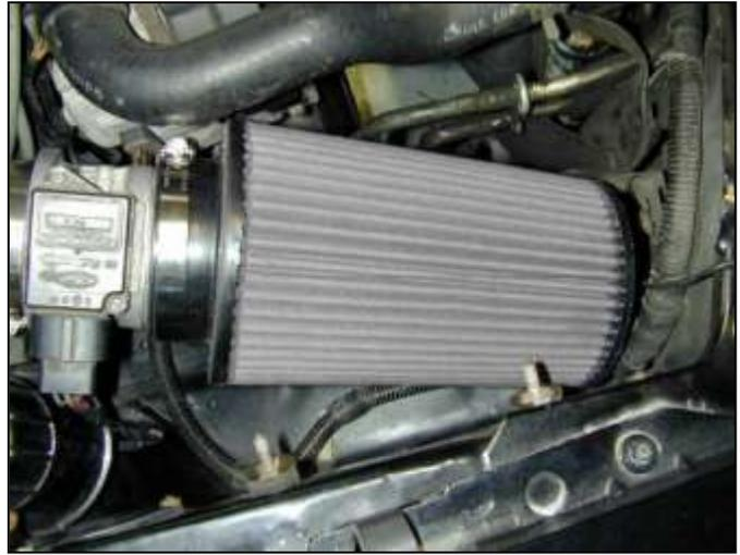
i. Attach the air filter element to the MAF sensor and secure. Check for clearance.
