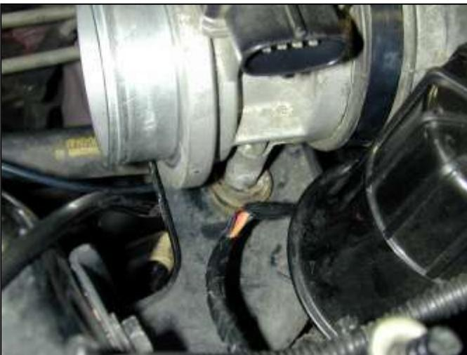
c. Loosen the bolt anchoring the MAF sensor and remove. The bolt head is located underneath the sensor.
