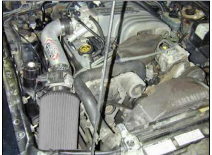
AEM® intake system installed
