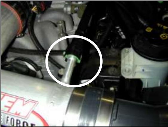
s. Re-attach breather hose. Make sure connector snaps onto the nipple.
