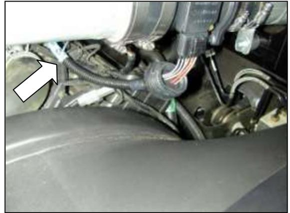
t. Secure MAF wire harness away from the fan with provided zip tie. **Failure to do so may damage harness and may result in engine failure.**
