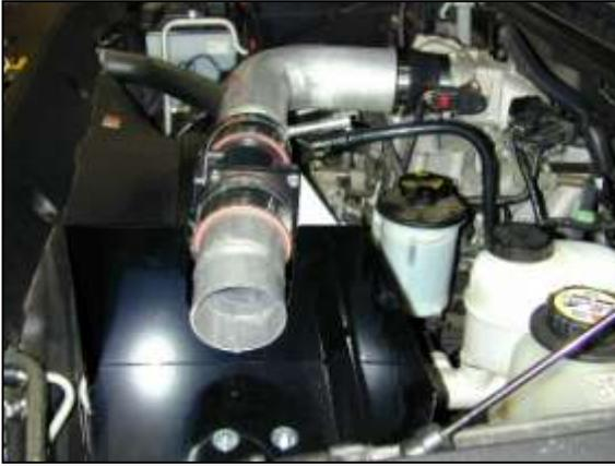
q. Align the both inlet pipes along with the MAF sensor assembly to the bracket on the heat shield.
