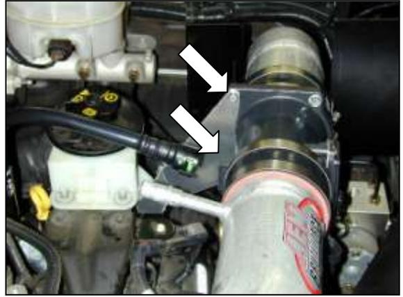
r. Secure the MAF sensor bracket to the remaining two holes on the assembly. Re-align to the rubber mount and secure rubber mount to the pipe bracket. Check clearance through the heat shield.
