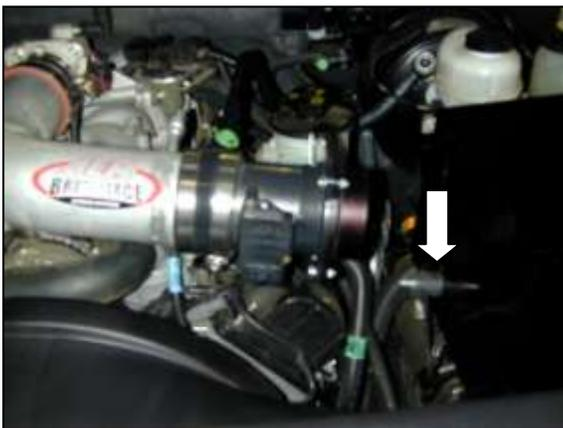
o. Insert rubber mount into the heat shield and secure with provided washer and nylok nut.
