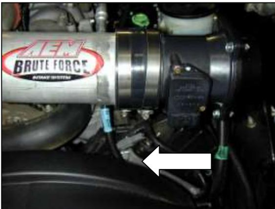
m. Insert the MAF sensor assembly into the coupler.
