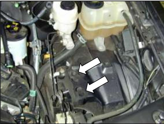
b. Remove rubber grommets left by the filter element housing.
