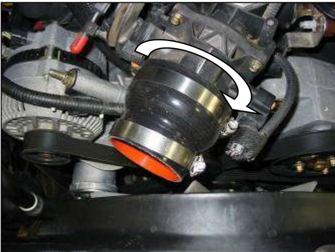
b. Place coupler over the throttle body as shown. Align the worm screw of the large hose clamp **AWAY** from the throttle body cable pulley. Tighten the large clamp.
