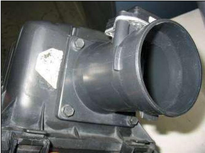
f. Remove the MAF sensor from the air box.
