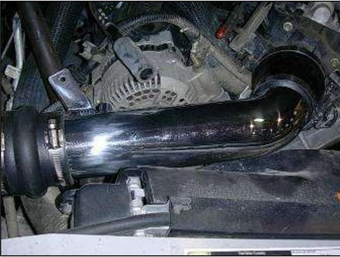
l. Place the inlet pipe in the engine bay as shown.
