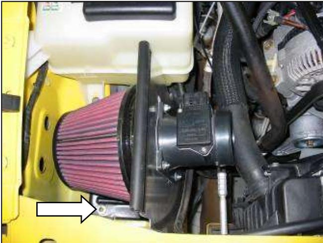
j. Place the heat shield/air filter/MAF sensor in the engine bay. Secure it to the chassis with the original bolts.
