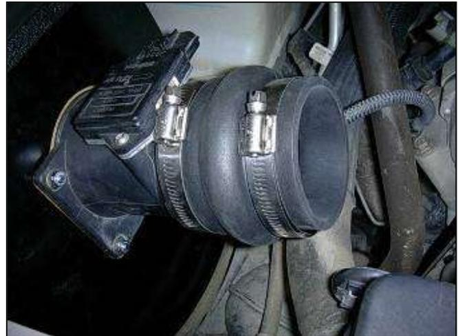
k. Install the large end of the hump hose over the MAF sensor housing as shown.
