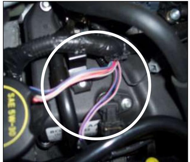
m. Pull MAF sensor plug towards MAF sensor.
