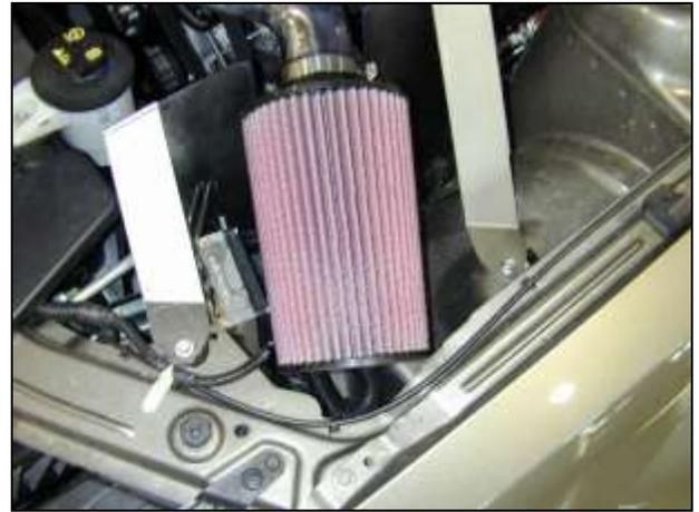
k. Install the AEM® air filter onto the end of the intake pipe. Push the air filter over the intake pipe until the stop in the air filter is reached. Secure the air filter onto the intake pipe with the supplied hose clamp.
