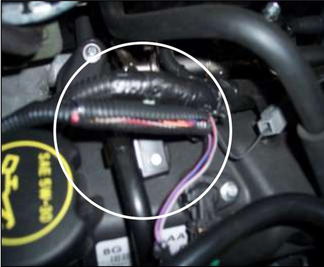
n. Place the factory convoluted slit covering over the wires as indicated in the picture above.
