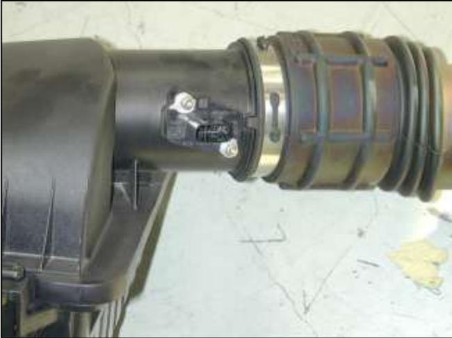
e. Remove the two screws retaining the MAF sensor with the supplied Torx tool and then carefully remove the MAF sensor.
