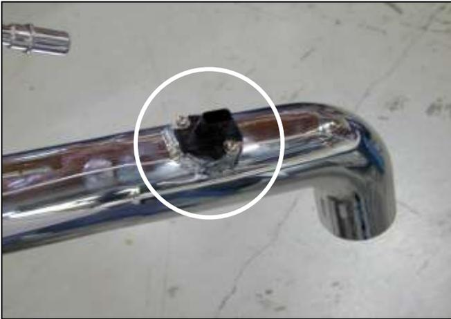
f. Ensure that the AEM<sup>®</sup> intake pipe is clear of debris. Install the MAF sensor using the supplied mounting screws. Use caution to avoid damaging the o-ring.
