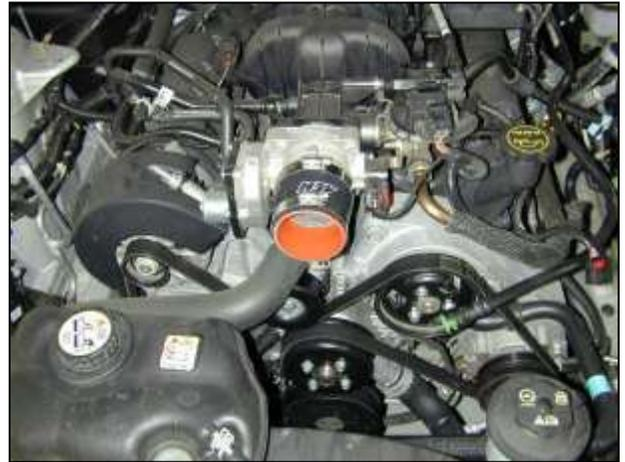
g. Install the supplied adapter hose onto the throttle body as shown using the #48 hose clamp.
