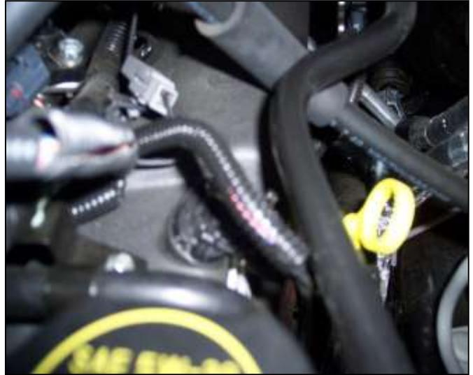
o. Place supplied convoluted slit covering over the remaining two wires as indicated in the picture above.
