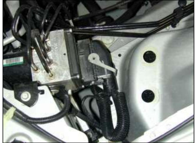
f. If your vehicle is not equipped with ABS, proceed to Step 3. Remove the ABS wire harness from the ABS control unit. This is done by pushing in on the locking button and rotating the latch mechanism toward the engine.
