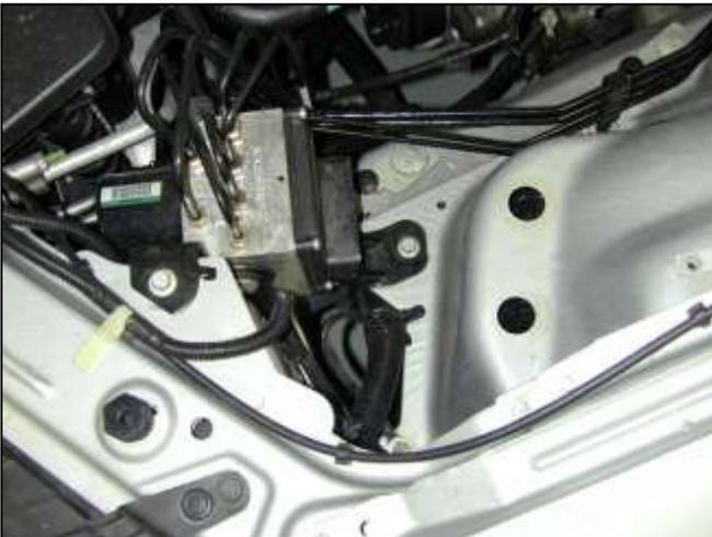
g. Move the harness out of the way and remove the upper and lower bolts securing the ABS unit to the chassis as shown. Set these bolts aside for now, they will be used during the AEM<sup>®</sup> intake system installation.
