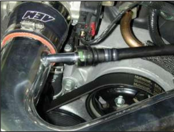
j. Attach the stock plastic breather hose by pushing it over the aluminum nipple on the AEM® intake pipe until it snaps into place.
