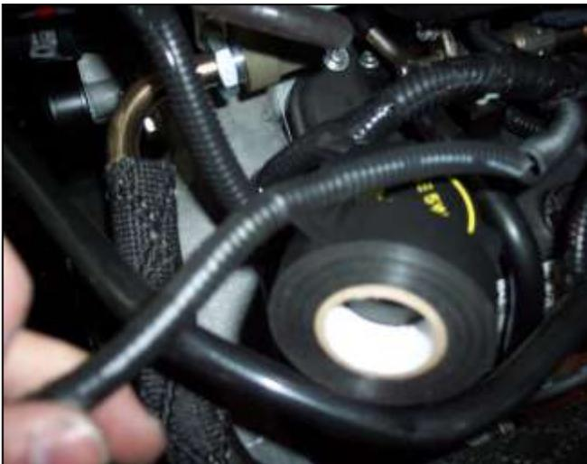
p. Wrap the factory convoluted slit covering with electrical tape to secure the wiring from potential damage.
