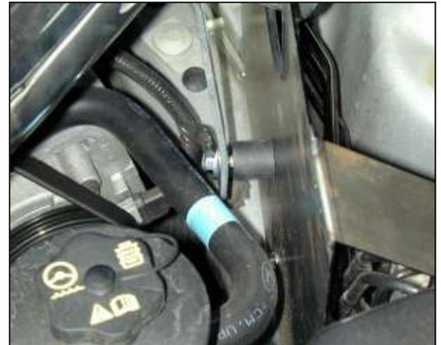
i. Align the mounting bracket with the rubber mount on the heat shield. Install the M8 washer and serrated nut onto the rubber mount. Leave slightly loose for adjustment.
