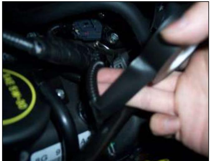
q. Wrap the supplied convoluted slit covering with electrical tape to secure the second group of wires.
