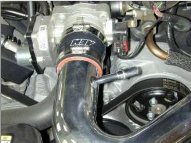
h. Insert the inlet pipe into the coupler installed on the throttle body as shown.
