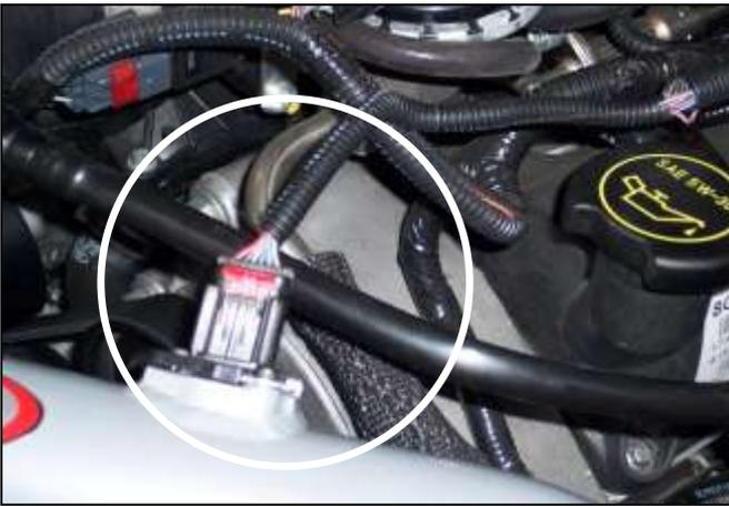
r. Plug in the wire harness into the MAF sensor.
