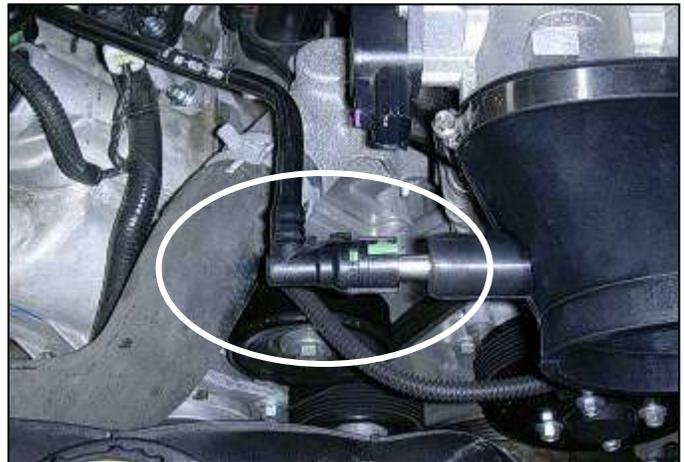
k. Attach the stock plastic breather hose by pushing it over the aluminum nipple until it snaps into place.
