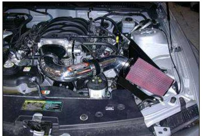
AEM<sup>®</sup> intake system installed
