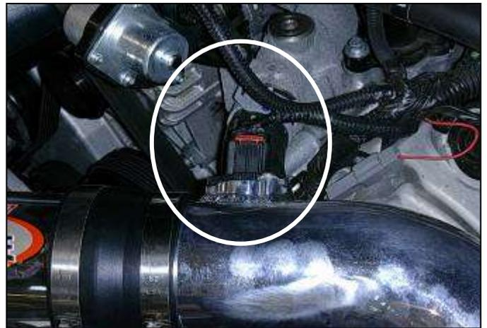
s. Plug in the MAF sensor on the pipe, the throttle position sensor and the throttle plate control motor on the throttle body. Zip tie TPC motor harness to MAF sensor harness.
