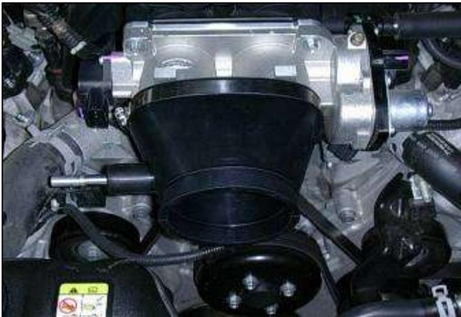
j. Install the adapter coupler onto the throttle body using the #72 hose clamp.
