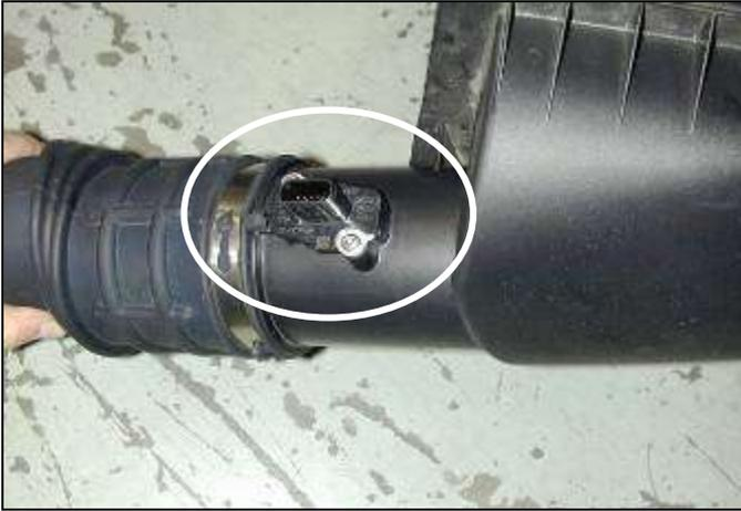
e. Remove the two screws retaining the MAF sensor and carefully remove the MAF sensor.
