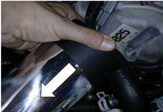
n. Slide the carbon trap into the end of the upper intake pipe until it reaches the flange on the rubber isolator.
