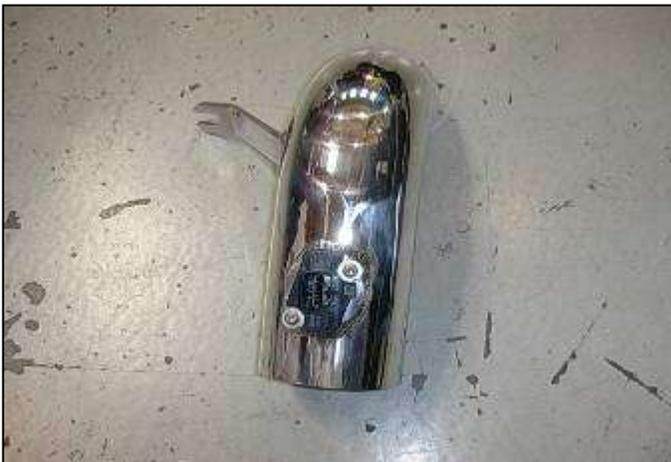
h. Check to be sure that the AEM® intake pipe is clear from debris. Install the MAF sensor using the original mounting screws. Use caution to avoid damaging the o-ring.
