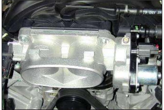
c. Install the throttle body spacer onto the two studs on the intake manifold with the two o-rings facing outward. Install the throttle body using the two previously removed nuts and bolts. Tighten to 84 inch pounds (7.0 ft-lbs).
