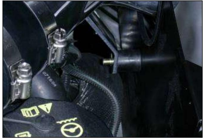
q. Install the M8 washer and nylok nut onto the rubber mount. Leave slightly loose for adjustment.
