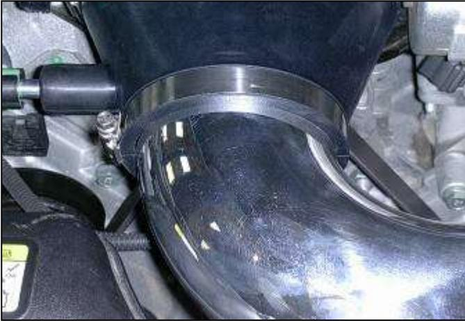
l. Check the inside of the AEM® upper intake pipe to ensure it is clear of any debris. Install the pipe with the bend side into to the previously installed coupler. Secure using a # 56 hose clamp as shown.
