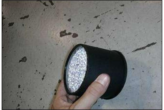
m. Vehicles not equipped with the carbon trap proceed to step 3o. Vehicles equipped with a carbon trap: Install the carbon trap into the supplied rubber isolator. The carbon trap is non-directional and can be installed in the isolator freely.
