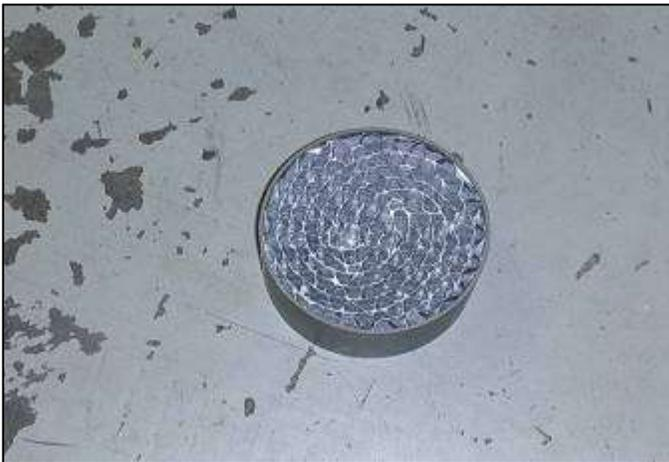
k. This carbon trap is on 2005 model year Mustangs with air induction system part numbers 4-R33-9C662-BJ (4.6L3V M/T) and 4R33-9C662-CF (4.6L 3v A/T) Remove the carbon trap by using a flat head screwdriver and gently prying it out of the stock intake tube.
