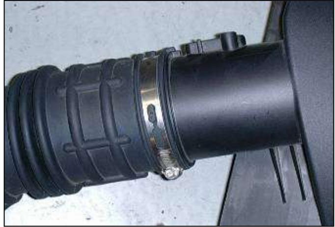
j. Separate the stock intake tube from the air box by loosening the hose clamp securing them. Look inside of the air intake tube to see if there is a carbon trap present and if so proceed to next step. Otherwise proceed to step 21.
