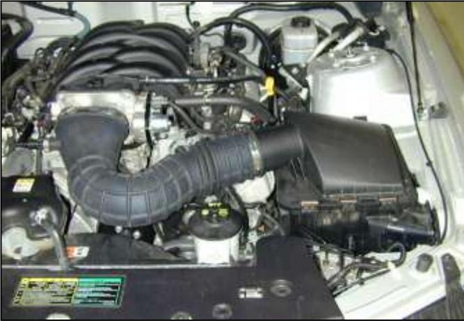
a. Factory air box system installed.
