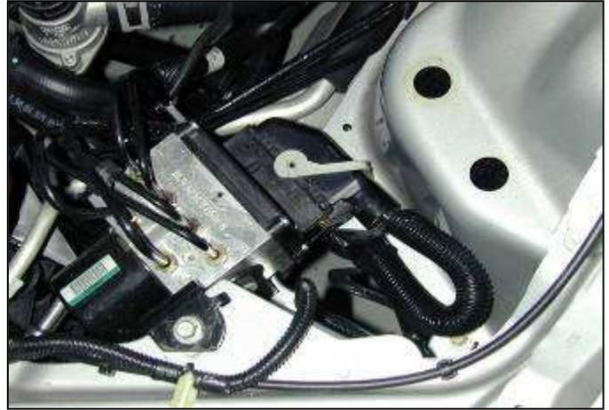
f. Remove the ABS wire harness from the ABS control unit. This is done by pushing in on the locking button and rotating the latch mechanism toward the engine.
