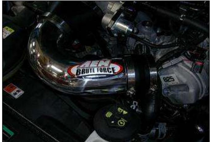
o. Install the rubber reducing coupler onto the upper intake pipe. Secure using the supplied #56 hose clamp.
