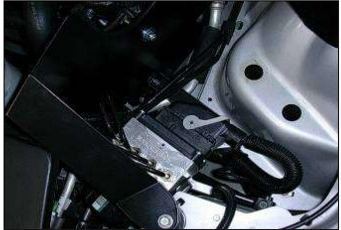
g. Plug the ABS wiring harness back into the ABS control module.
