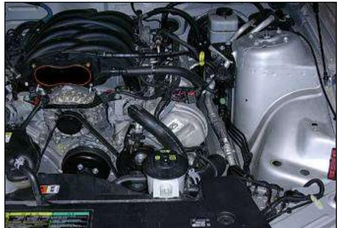
l. Factory air box system removed.
