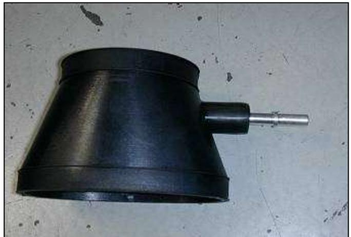
i. Install the aluminum nipple into the EPDM throttle body adapter coupler. This is done by pushing the nipple into the bung from inside the coupler. Next, pull the nipple through until it locks into place.
