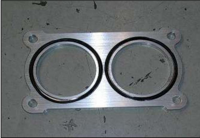
b. Install the two supplied o-rings into the throttle body spacer. Dab a small amount of grease into the groove to hold the o-rings in place during assembly.
