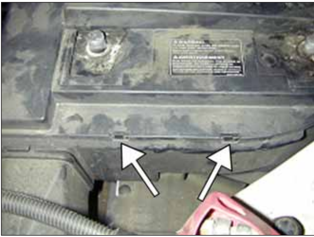
e. Unclip the front side of the battery box cover as shown.
