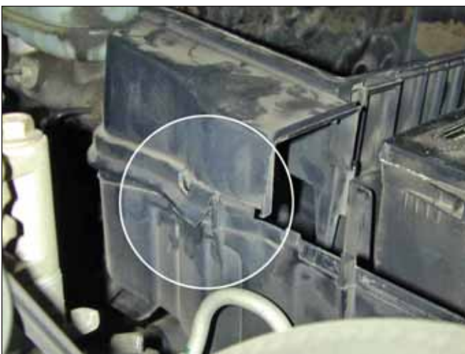
i. Unclip the passenger's side snap of the lower air filter housing. Remove the lower air filter housing.
