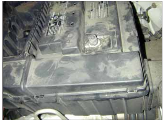
f. Unclip the passenger side of the battery box cover. Remove the battery box cover by gently lifting it straight up and out of the engine bay.
