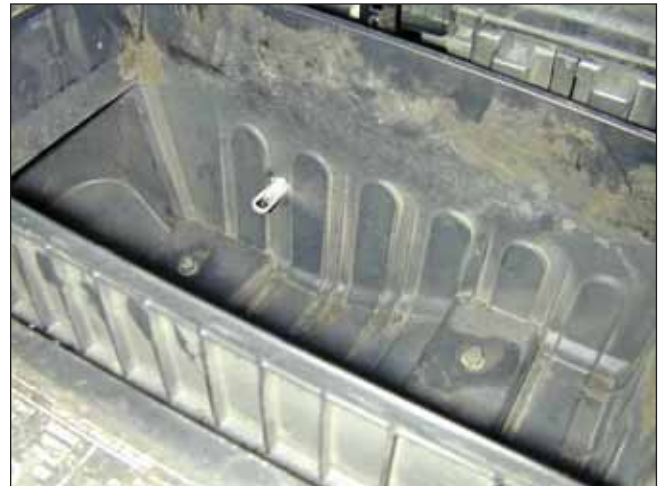
h. Remove the Inlet Air Temperature (IAT) sensor from the air filter housing by rotating it 90 degrees and gently pulling it out.
