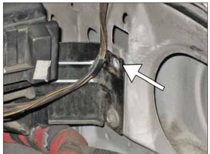
j. With the air filter housing removed, locate the upper bolt securing the fuse block mount to the driver's side fender as shown. Remove the bolt.
