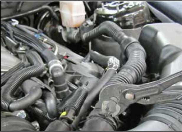
e. Release the spring clamp on the sound tube using a pair of pliers.
