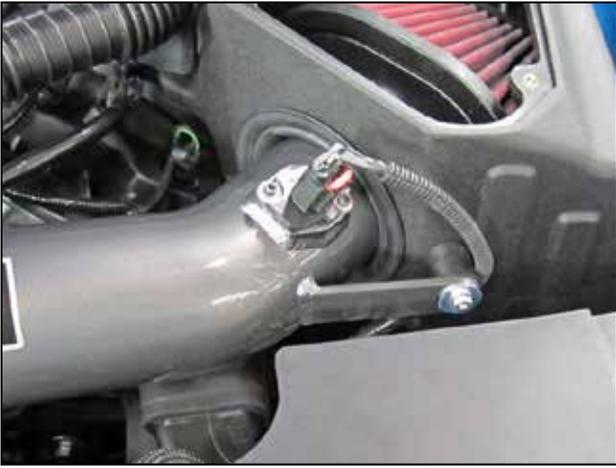
x. Attach the MAF sensor harness connector to the MAF sensor. Adjust the intake pipe for best fitment, then tighten the M6 nut and remaining hose clamp.
