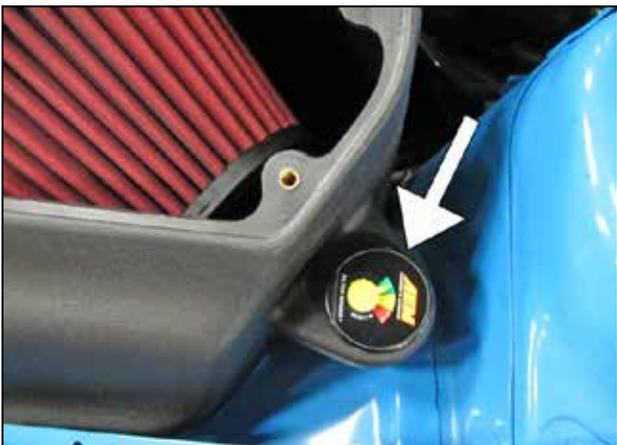
v. Install the filter minder by pressing it into the grommet installed in step 3f.
