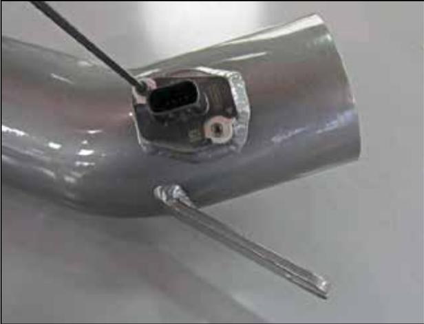
b. Install the MAF sensor into the AEM® intake pipe using the two supplied M4 bolts (#1-2105).
