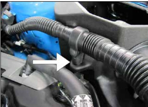
p. Plug the rubber support into the hole of the AEM® airbox as shown.
