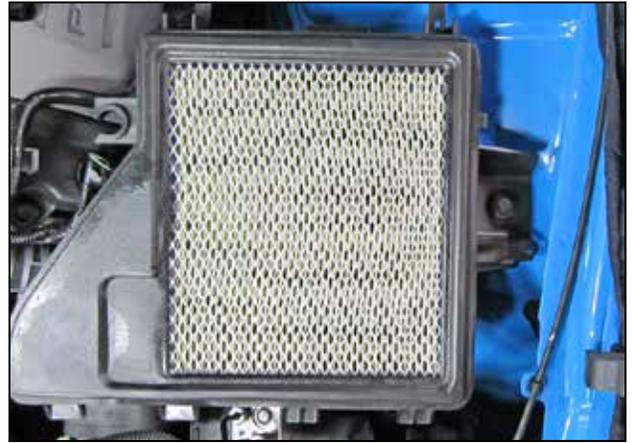
l. Remove the inlet tube from the throttle body and lift the airbox lid off of the lower airbox. Remove the airbox and inlet tube assembly.
