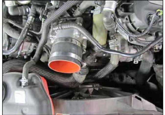
c. Install the 3.5" coupler and two (#9456) hose clamps onto the throttle body. Slide the coupler all the way onto the throttle body, position the hose clamps as shown, and tighten the throttle body-side hose clamp.
