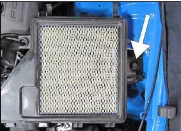
m. Remove the M6 bolt securing the lower airbox, then remove the lower airbox.
