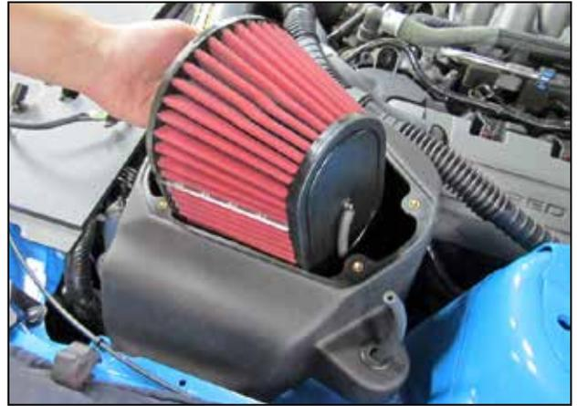
s. Attach a (#9456) hose clamp onto the air filter and lower it into the airbox as shown. Feed the 5/32" hose up through the grommet from inside the airbox.
