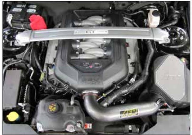
aa. Reinstall the strut brace and tighten all 4 nuts.
