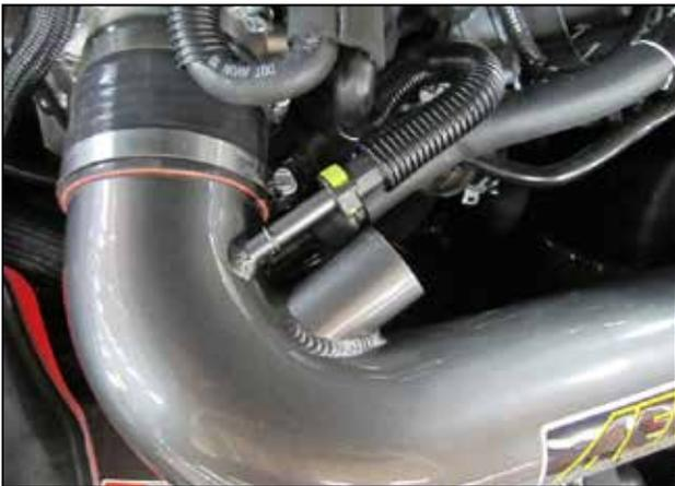
n. Connect the OEM vent tube(s) to the AEM® intake pipe by firmly pressing the connector onto the respective nipple until it 'clicks' into place. On manual trans. vehicles, cap the smaller nipple with the supplied vac. cap. (#8-101).
