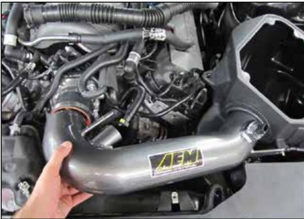
l. Install the AEM® intake pipe as shown. Make sure that the bracket engages the stud on the rubber mount.
