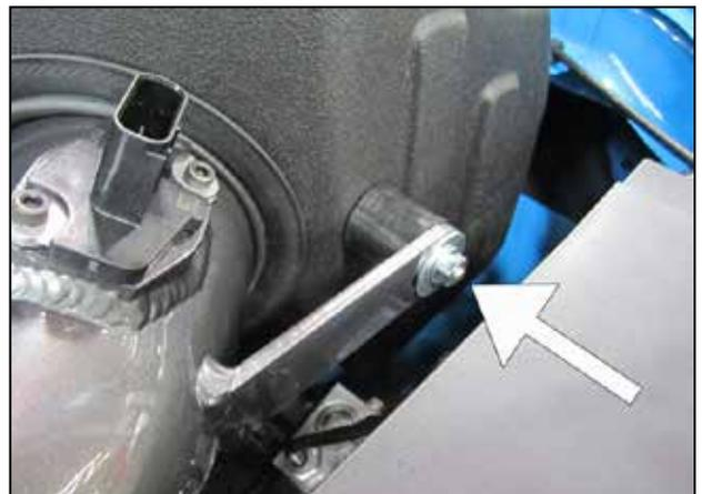
w. Secure the pipe bracket to the rubber mount with a supplied M6 nut (# 444.460.04) and washer (#08160).
