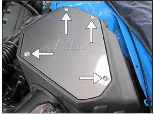
y. Install the AEM® airbox lid using the 4 supplied M6 button head bolts (# 1-112) and nylon washers (#1-3001).
