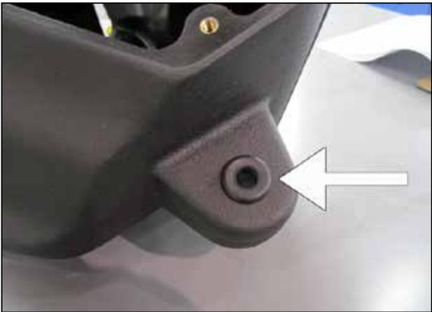
f. Install the supplied grommet (#784642) into the hole in the airbox as shown.
