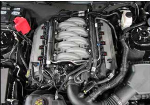
c. Remove the engine cover by lifting up on it from the front and releasing the 4 snap clips.
