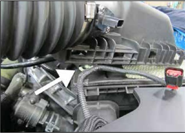
k. Unclip the MAF sensor wire harness from the airbox lid.
