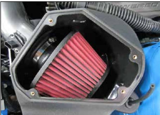
t. Install the air filter onto the end of the AEM® intake pipe and position the filter as shown. Make sure that the pipe is bottomed out on the stops within the air filter. Once proper fitment of the air filter is achieved, secure the (#9456) hose clamp.
