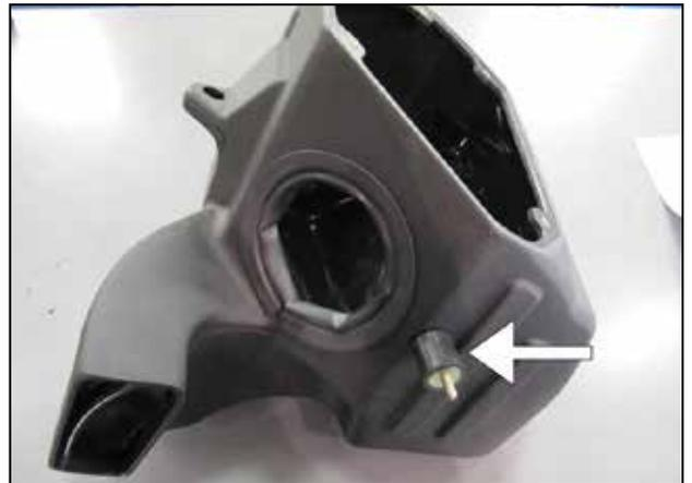
e. Install the rubber mount into the AEM® airbox as shown. Thread the short stud of the rubber mount into the airbox's threaded hole; hand tighten.
