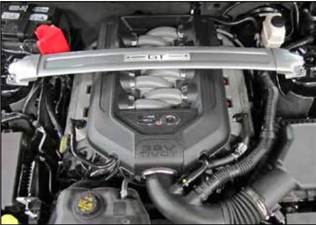
a. Loosen and remove the 4 nuts securing the strut brace.
