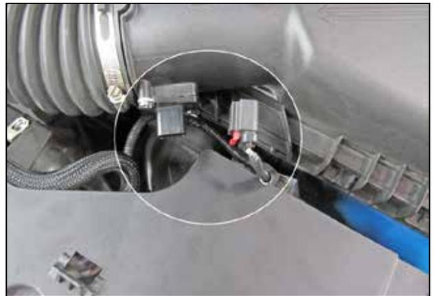
d. Unplug the MAF sensor. First pull back on the red latch, then squeeze to release the connector.
