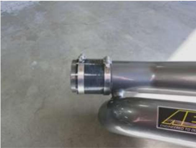
i. Install the straight coupler with hose clamps onto the AEM tube. Note: Use soap and water to allow the coupler to slide on the intake tube.
