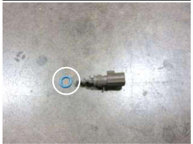
h. Remove the O-ring from air temperature sensor.
