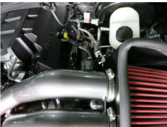
m. Connect the air temperature sensor connector onto the air temperature sensor that was removed in step 2b.
