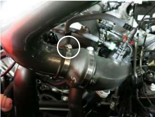
k. Align the AEM intake tube with the step coupler that was previously installed in step 3h. Tighten the hose clamp circled at this time.
