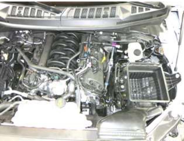
c. Remove intake tube by lifting top half of air box and moving the whole assembly out, from left to right. Remove factory panel air filter. **Retain all stock components.**
