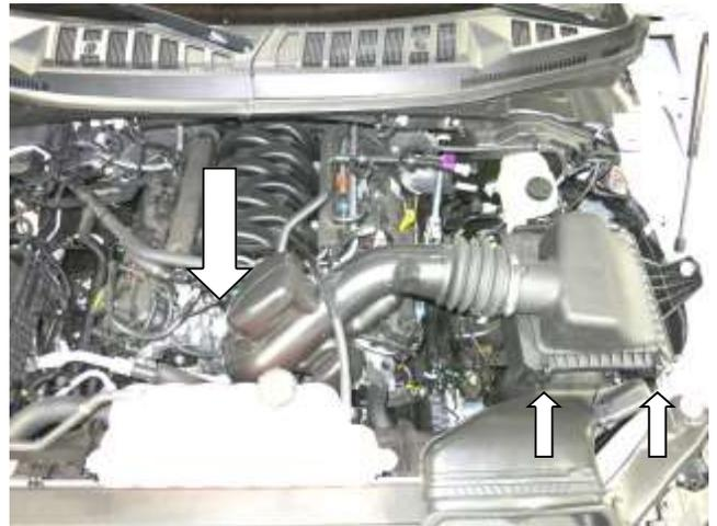
b. Loosen hose clamp at throttle body and release the two clips securing top half of air box.
