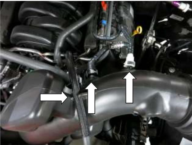
a. Disconnect EVAP vent and crack case vent connectors from factory intake. Pop coolant hose out of notch.
