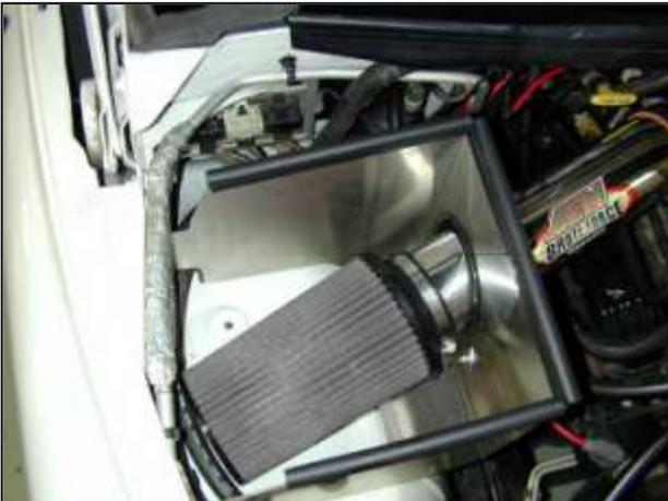
k. Install the AEM® air filter onto the end of the inlet pipe. Push the air filter onto the inlet pipe up to the stop molded in to the air filter neck.
