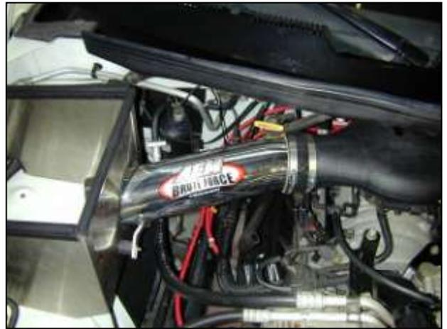
j. Install the AEM® inlet pipe. The mounting bracket should line up with the rubber mount on the heat shield.
