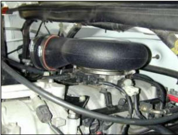
i. Secure the AEM® intake plenum to the throttle body using the original clamp and gasket. Do not tighten the clamp completely to allow for rotation and adjustment of the intake pipe during installation.
