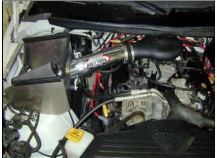
AEM<sup>®</sup> intake system installed
