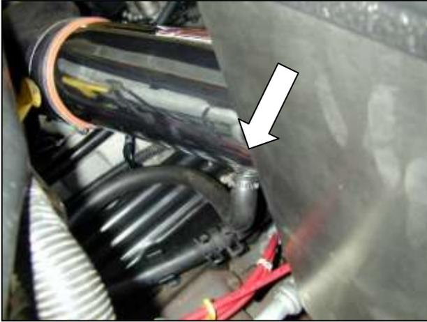
m. If the breather hose was originally on the passenger side of the air box, attach the stock crankcase breather hose to the nipple on the backside of the AEM<sup>®</sup> inlet pipe and secure with the supplied 1" hose clamp. If breather hose was originally on the driver's side, install supplied length of 1/2" hose between valve cover and breather nipple on AEM<sup>®</sup> inlet pipe and secure with the two supplied hose clamps.
