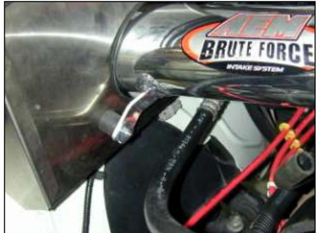
l. Secure the inlet pipe bracket to the rubber mount using the remaining M6 fender washer and locknut. Refer to the diagram below for proper rubber mount installation.
