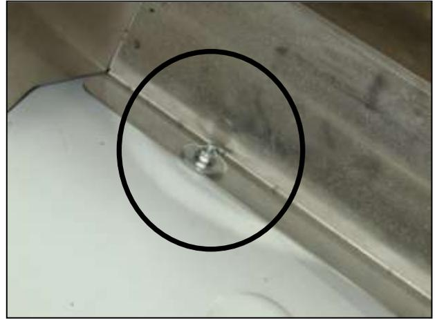
f. Secure the third heat shield mounting point using the supplied M6 bolt, washer, fender washer, and locknut. Install the bolt and small washer through from the tire side of the fender. Secure with the larger fender washer and locknut from the engine bay side.
