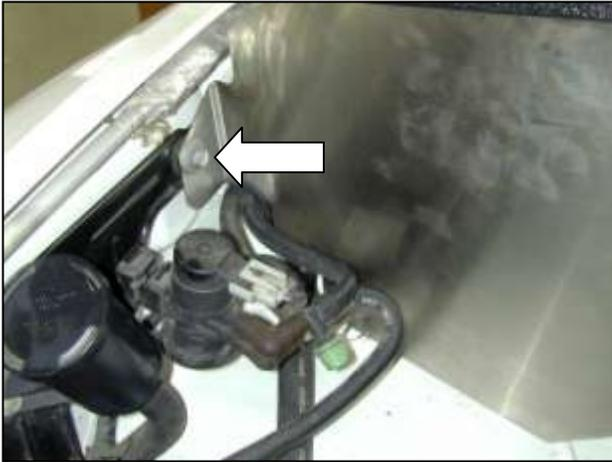
d. Install the heat shield into the engine bay. Secure the front mounting tab using the bolt removed in step 2e.
