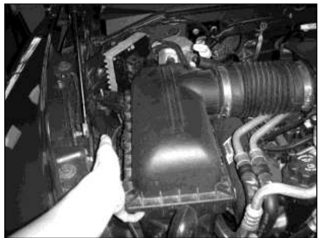
h. Gently pull the airbox out of the rubber grommets and remove the entire intake system from the engine bay.
