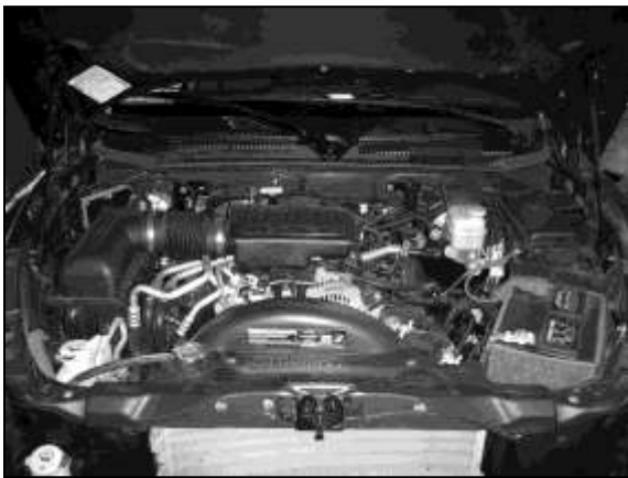
a. Stock air box system installed.
