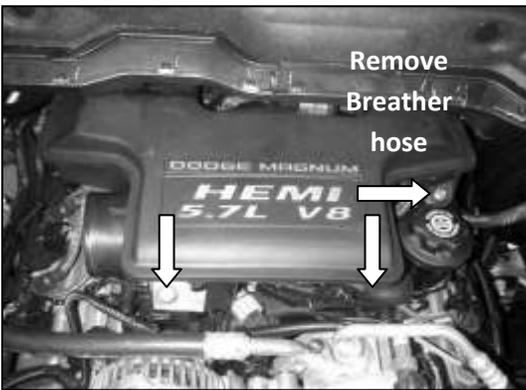
g. Remove the two bolts retaining the intake air resonator. Remove breather hose.
