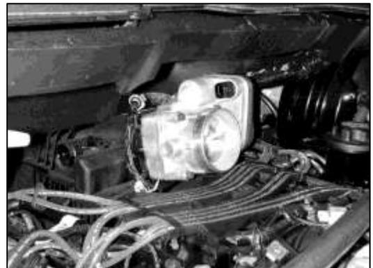
e. Install the throttle body using the supplied M6 bolts and washers. Align the dowel pins on the throttle body spacer with the holes in the throttle body. Before installing the throttle body spacer, make sure the o-ring is seated. Reconnect the electrical connector.
