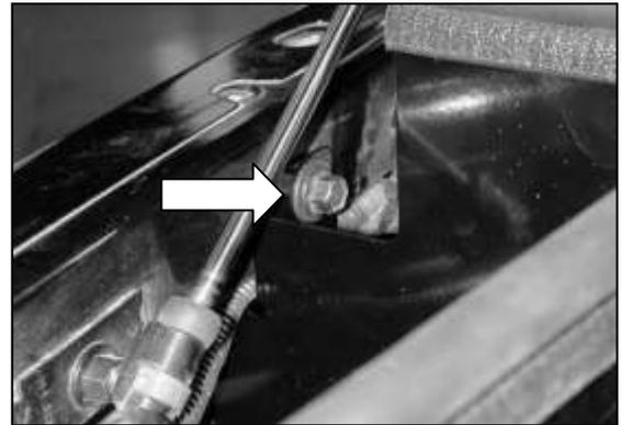
k. The rear mounting tab on the heat shield will line up with one of the lower air box mounting holes. Install one of the original bolts. Adjust the heat shield for best fitment then tighten the three mounting bolts.
