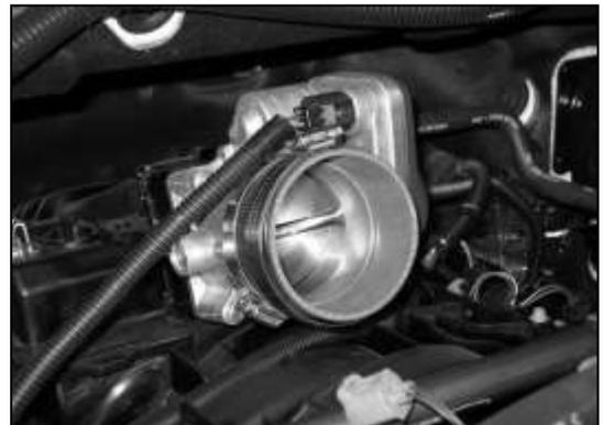
m. Loosely install the coupler and hose clamps onto the throttle body. Secure with provided hose clamps.
