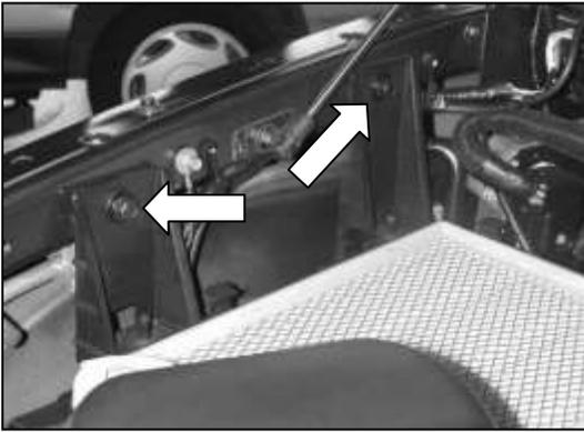
e. From inside the engine bay, remove the two remaining bolts securing the bottom half of the air box. Remove the bottom half of the air box and the air filter element.
