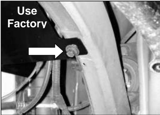
j. The lower heat shield mounting tab will line up with the lower air box mounting hole. Loosely secure the mounting tab with one of the original bolts.
