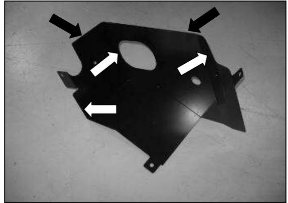
g. Install the rubber edge trim (PN: 8-4022) on the edges indicated with the white arrows. Install the sponge rubber gasket (PN: 8-3034) along the top of the heat shield indicated with black arrows.
