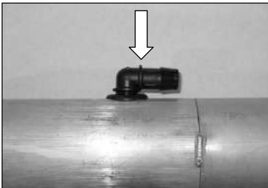
n. Insert the 1" grommet into the pipe. Insert the 90 degree plastic connector into the grommet. Be careful not to push the grommet through the pipe.
