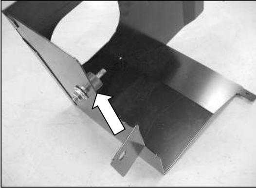
b. Install the supplied rubber mount into the heat shield as shown, place a M8 washer on the stud and a M8 nut to secure.
