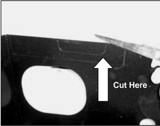
f. Trucks equipped with the optional under hood light on the **passenger side**, cut the corners on the small section of the top notch in the heat shield using a hacksaw or other suitable tool. Bend the tab back and forth until it breaks free. Clean up any sharp edges with a file. Vehicles not equipped with the under hood light, proceed to next step.
