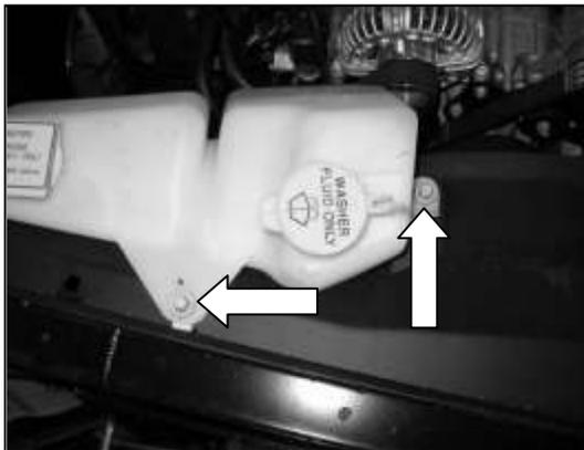
h. Loosen and remove the overflow reservoir mounting bolts.
