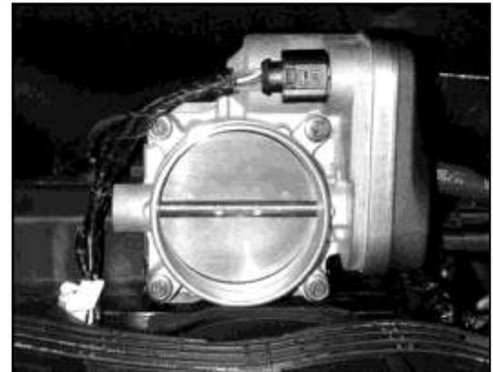
j. Remove the four bolts securing the throttle body. Unplug the electrical connector and remove the throttle body from the intake manifold.
