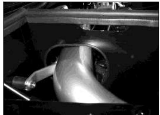
o. Insert the pipe as shown. Line up the support bracket to the rubber mount and secure. See diagram on next page.
