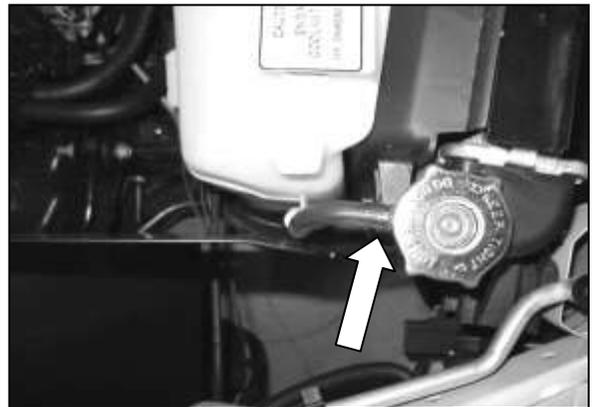
i. Disconnect the overflow tube to gain access to the upper radiator fan shroud bolt. Install the heat shield from inside the fender well. Place the front heat shield tab between the fan shroud and radiator end tank. Replace the factory bolt and overflow bottle.
