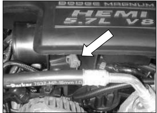
f. Unplug the inlet air temperature (IAT) sensor located on the front side of the intake air resonator.
