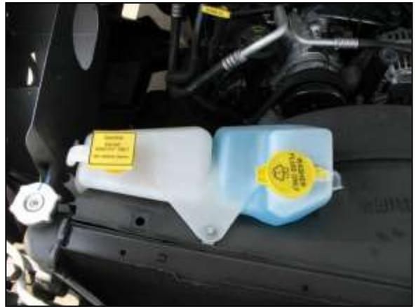
g. Reinstall the washer/coolant overflow reservoir.
