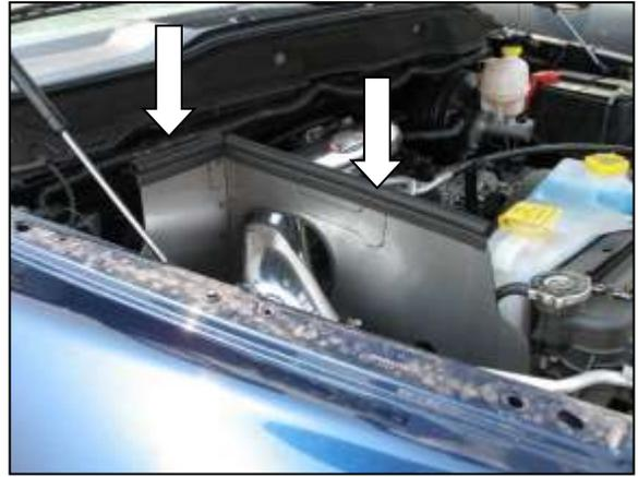
q. Attach the sponge gasket to the top of the heat shield.
