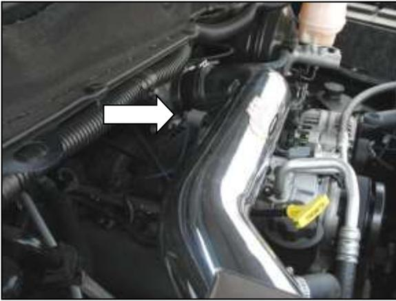
p. Reattach the IAT sensor harness connector to the IAT sensor.
