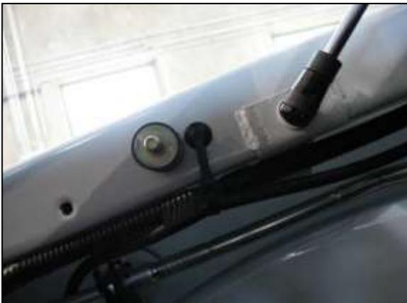
b. Install the supplied rubber mount into the passenger side fender.
