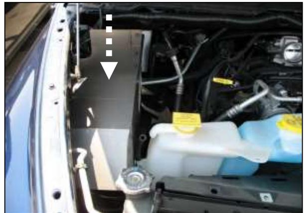
c. Insert the heat shield as shown.
