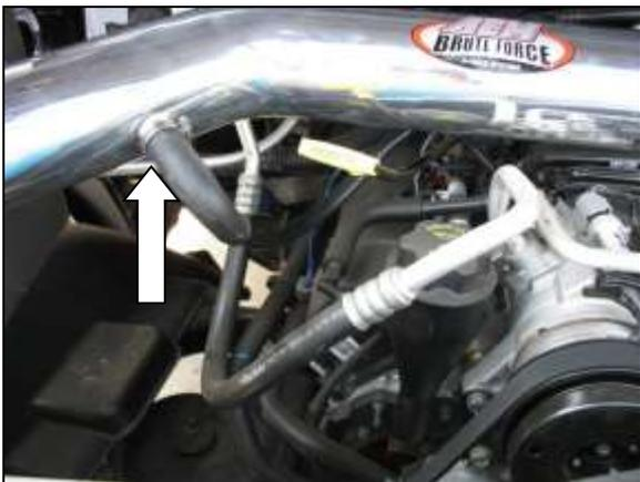
n. Attach the breather hose to the inlet pipe as shown. Secure with the provided hose clamp. Make sure that the rubber elbow is not kinked for air flow.
