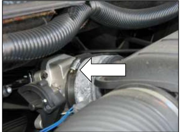
b. Loosen the hose clamp securing the throttle body coupler.
