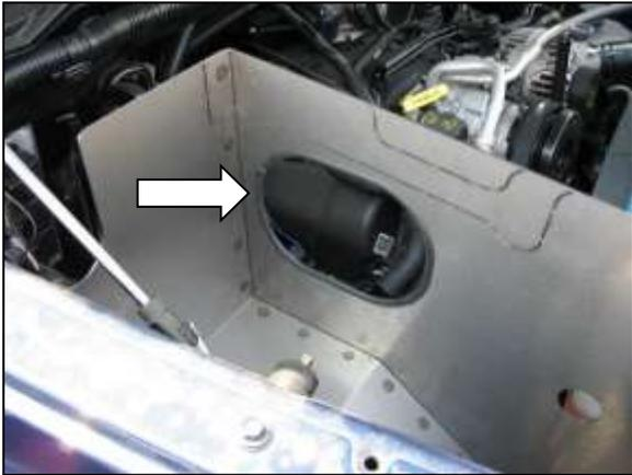
l. Attach the rubber edge trim to the heat shield opening.
