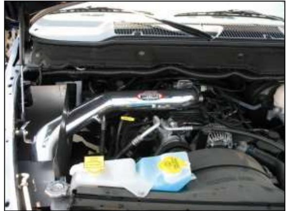
m. Insert the inlet pipe as shown. Secure at the throttle body with a #60 hose clamp. Align the bracket with the rubber mount. See diagram for proper assembly.
