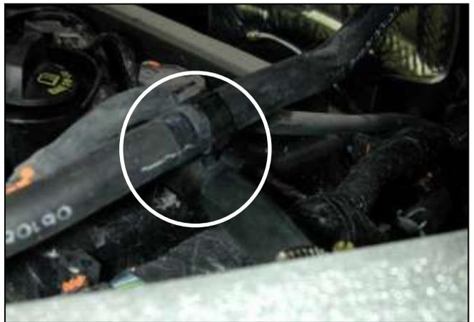
m. Secure both breather hoses with the factory clip (if equipped). Reinstall the engine cover.
