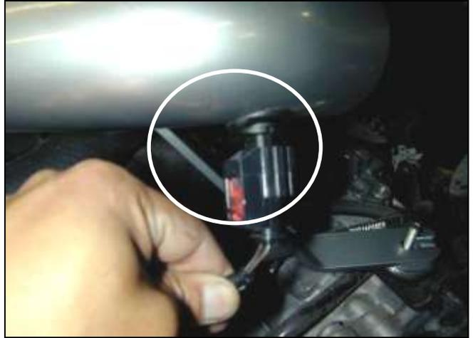
k. Reattach the IAT sensor wire harness connector. Check for clearance around the negative battery terminal.
