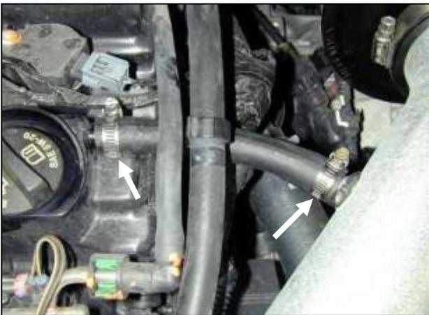
l. Attach the breather hose as shown to the inlet pipe and to the crank case vent. Secure with hose clamps.
