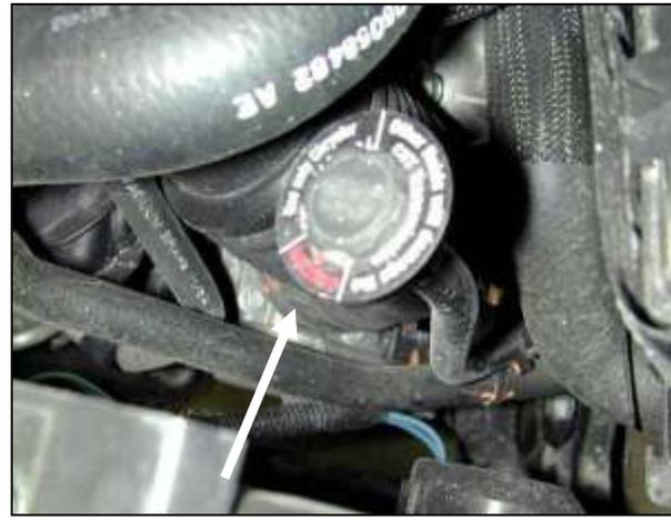
d. Loosen the inlet tube's hose clamp at the throttle body. Loosen the inlet resonator tube mounting bolt; this is located near the throttle body.
