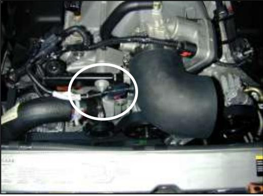
j. Attach the smaller end of the coupler to the throttle body and secure with provided hose clamp as shown. Reconnect the IAT sensor wire harness connector and lock in place.
