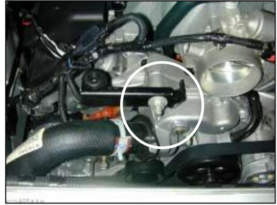
f. Loosen and remove the nut. Remove bracket and reinstall the nut.
