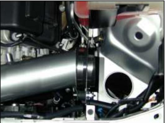
m. Attach the coupler and hose clamps to intake pipe and then secure.
