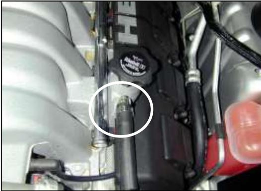
p. Attach the new crank case breather hose to the intake manifold. Tighten provided hose clamp to secure.
