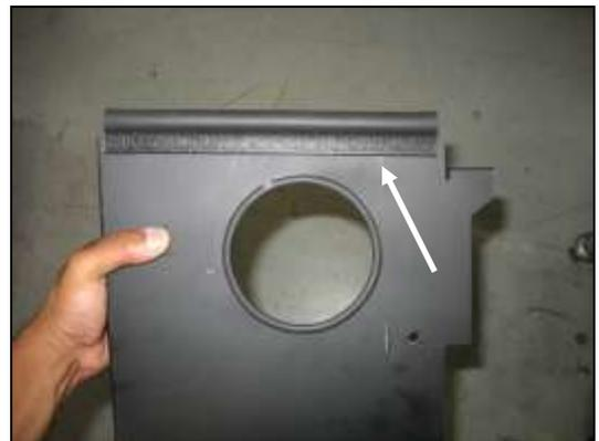
c. Attach the foam gasket onto the top of the heat shield. Trim excess.
