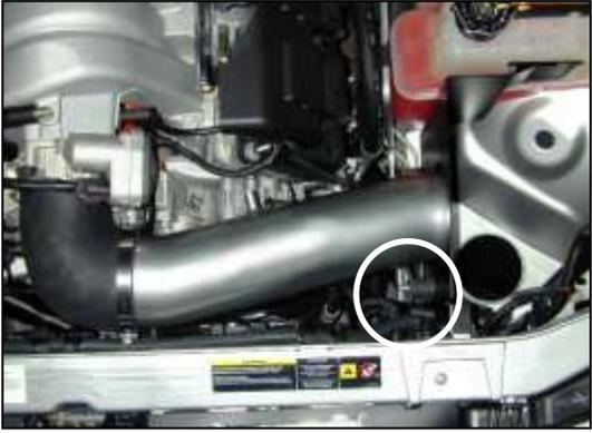
k. Insert inlet pipe as shown. Align the bracket to the rubber mount.
