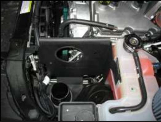
d. Insert the heat shield as shown. The vertical tab slides into the coolant reservoir. The bottom tab slides underneath the coolant and vacuum lines.
