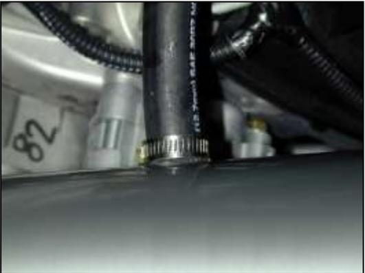
o. Attach the new crank case breather hose to the inlet pipe. Tighten provided hose clamp to secure.
