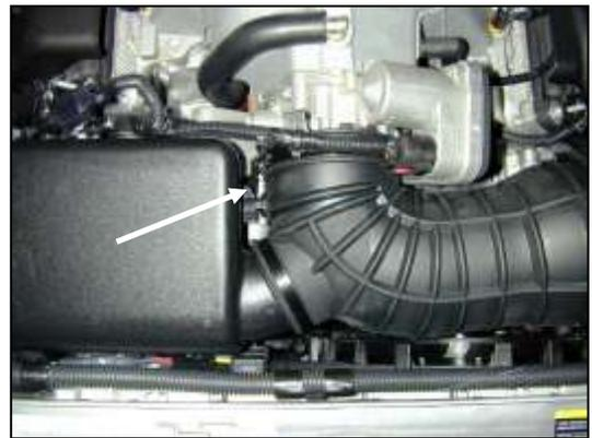
b. Loosen the throttle body hose clamp.
