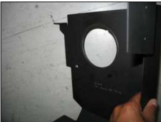
b. Attach the rubber edge trim to the inlet pipe opening on the heat shield. Trim excess.
