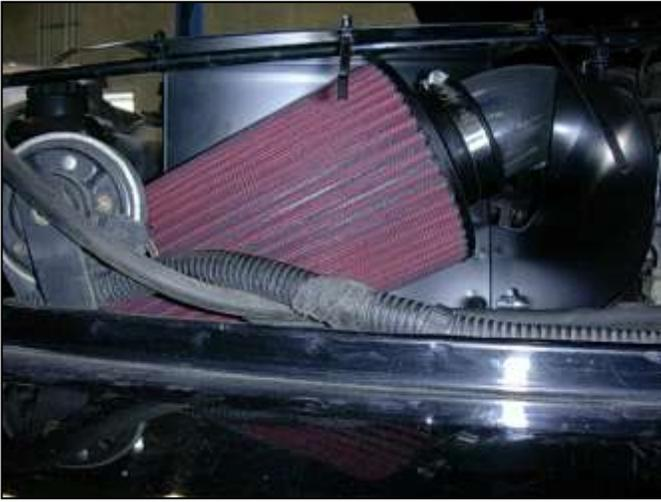
n. Ensure that the air filter is not touching any part of the vehicle. Position the AEM<sup>®</sup> intake system for best fitment. Be sure that the pipe or any other component is not in contact with any part of the vehicle. Tighten the hose clamps at the throttle body. Tighten the nut on the mounting bracket. Re-adjust pipe if necessary. Install rubber edge trim to the top of the heat shield
