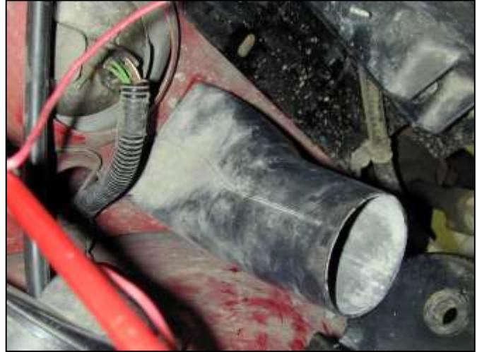
f. Remove the inlet air duct from below the headlight housing.
