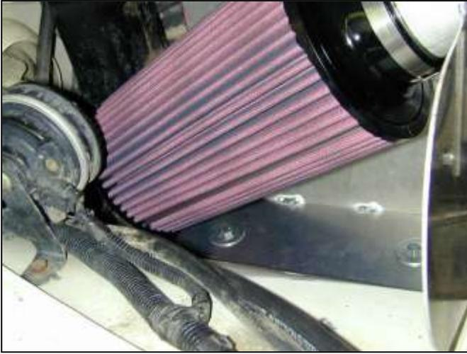
j. Install the AEM<sup>®</sup> air filter into the space behind the headlight. Push the filter over the inlet pipe until the stop in the filter is reached, and then install one hose clamp to secure the filter onto the inlet pipe.
