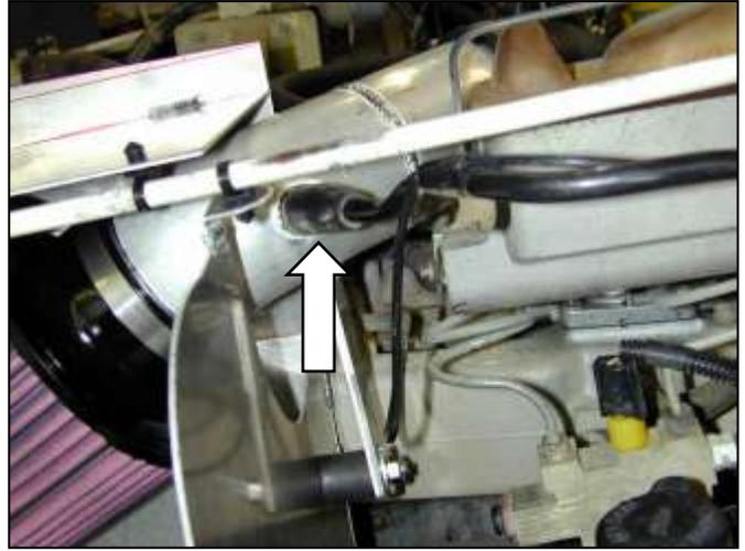
k. Attach the factor charcoal box breather line to the lower intake pipe by sliding it over the nipple.
