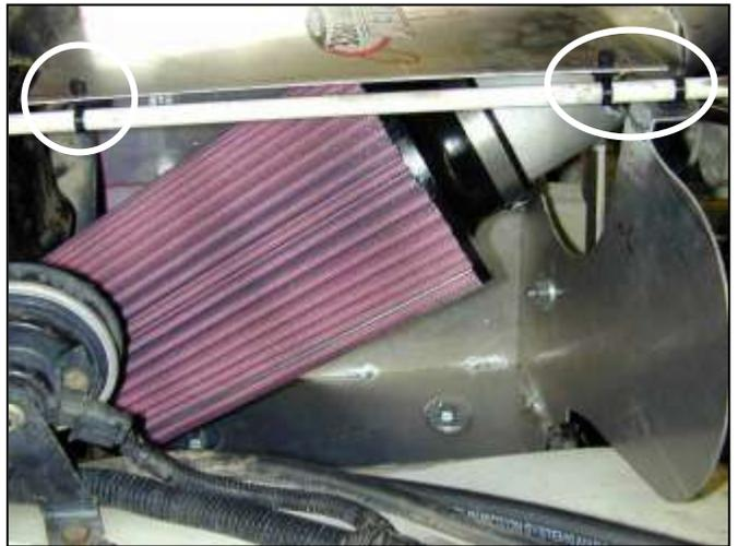
m. Swing the radiator support brace back to its stock location and secure. Wrap the heat shield zip-tie mounts around the brace and secure the heat shield to the brace.
