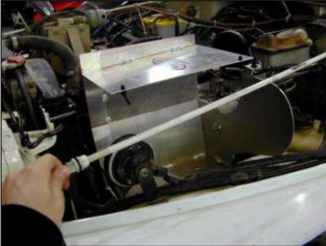
f. Install the heat shield by moving the radiator support bracket out of the way and aligning the holes in the bottom of the heat shield and stock air box bracket.
