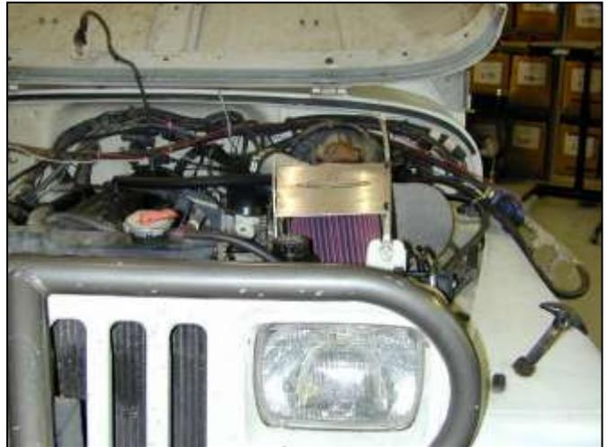
AEM<sup>®</sup> intake system installed
