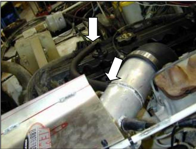
l. Install the supplied 1/2" breather hose between the intake pipe nipple and the valve cover elbow using two 1-1/16" hose clamps.
