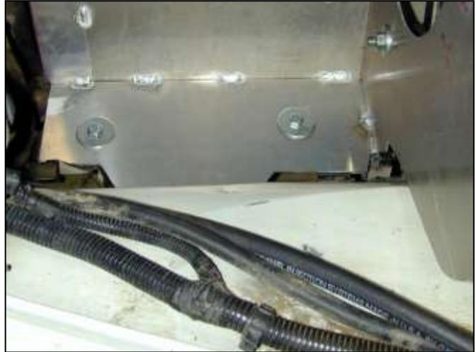
g. Install the two bolts, two nuts, and four washers to secure the bottom of the heat shield. Tighten until nut is snug but do not over tighten.
