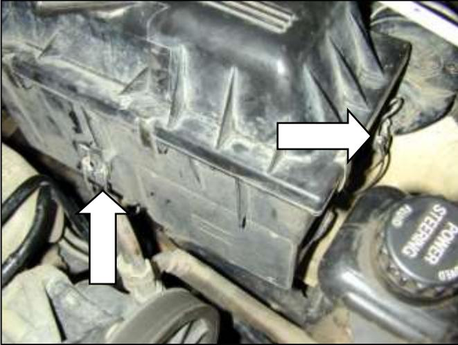
e. Un-clip the three hooks holding the air filter housing to the chassis. Lift the air filter housing and intake tube from the vehicle.
