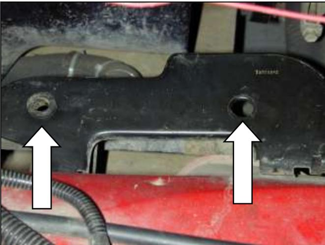
g. Remove the two rubber grommets from the air filter housing mount.
