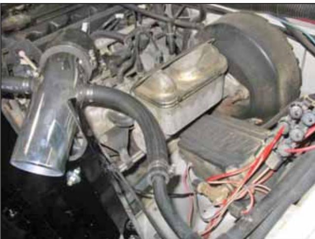
j. Install the supplied breather hose between the hard plastic charcoal canister hose and the nipple on the driver side of the intake pipe. Secure using the remaining 1" hose clamps. Trim hose to fit.
