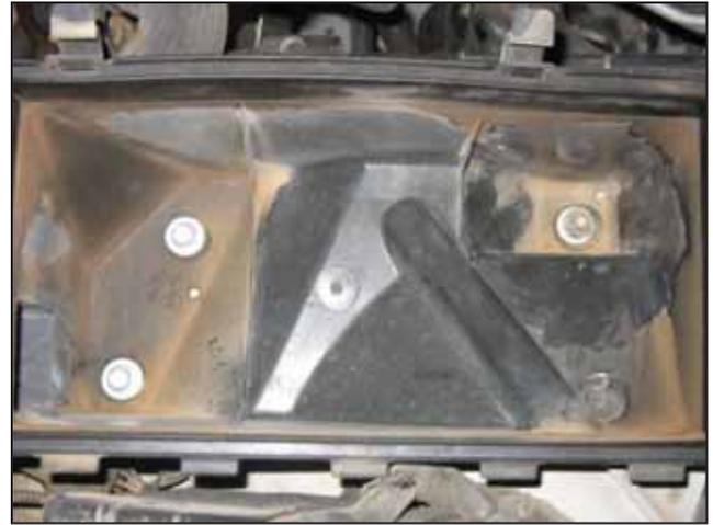
f. Remove the air filter from the housing. Remove the two bolts and the one nut from inside the filter housing. Lift up and remove the air filter housing base.
