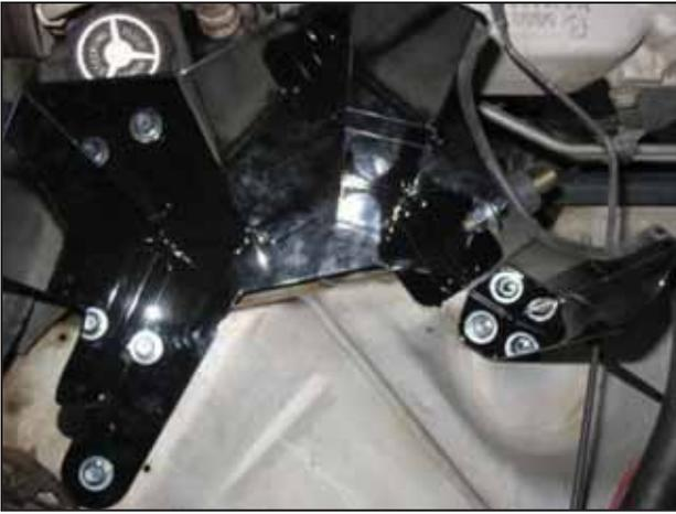
f. Install the heat shield by aligning the stud in the inner fender with the corresponding hole on the heat shield. Secure using the supplied M8 nut, two M8 bolts, and three washers.
