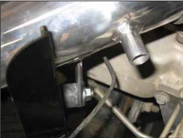
h. Slide the intake pipe into the elbow until the mounting bracket aligns with the rubber mount on the heat shield. Secure the pipe to the rubber mount using the remaining M8 washer and nut.
