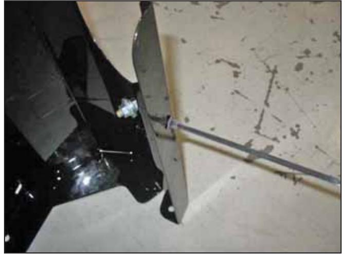
c. Install the tree mount zip-tie into the hole on the side of the heat shield as shown.
