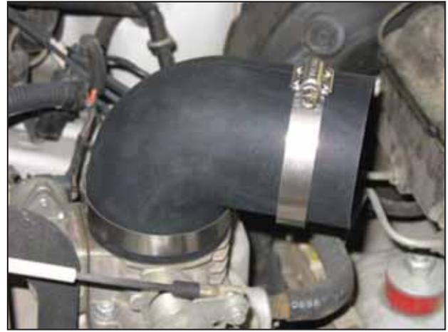
g. Install the 90 degree coupler onto the throttle body and secure using the supplied #48 hose clamps.
