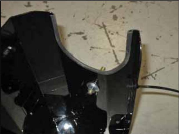
d. Install the rubber edge trim onto the top edge of the heat shield where the pipe passes through.
