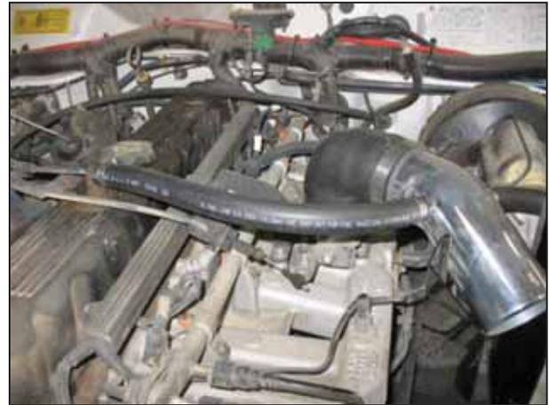
i. Install the hose between the valve cover breather nipple and the breather nipple on the engine side of the intake pipe. Secure using two of the supplied 1" hose clamps. Trim hose to fit.
