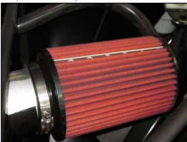
v. Attach the filter to the AEM air intake tube and attach the vent hose to the vent fitting on the heat shield.
