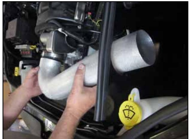
q. Install the AEM air intake tube (A) to the throttle body and through the heat shield opening.
