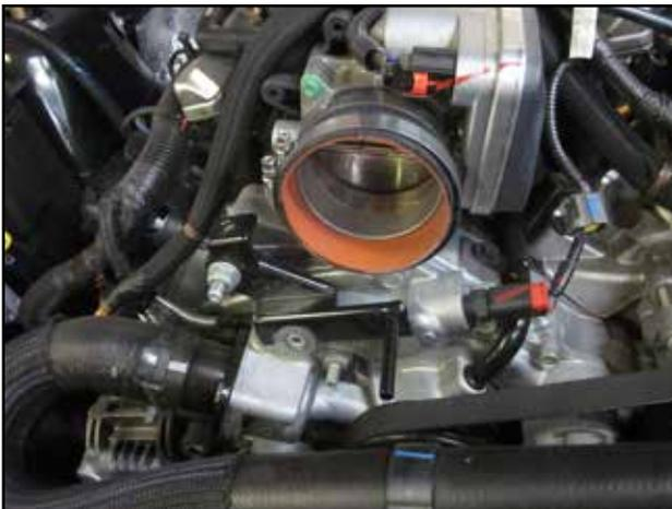
p. Install the supplied coupler (N) on the throttle body along with the supplied hose clamps (O).
