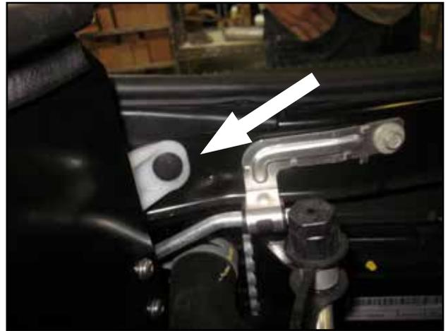
i. Place the windshield washer reservoir back in its place and reinstall the plastic clip removed from step 2-l).
