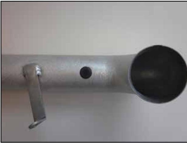
l. Install the supplied grommet (m) into the hole on the AEM intake tube.
