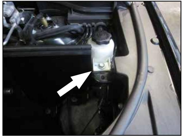
g. Place the power steering reservoir tab over the AEM heatshield bracket and install the factory M8 bolt. Do not tighten completely at this time.
