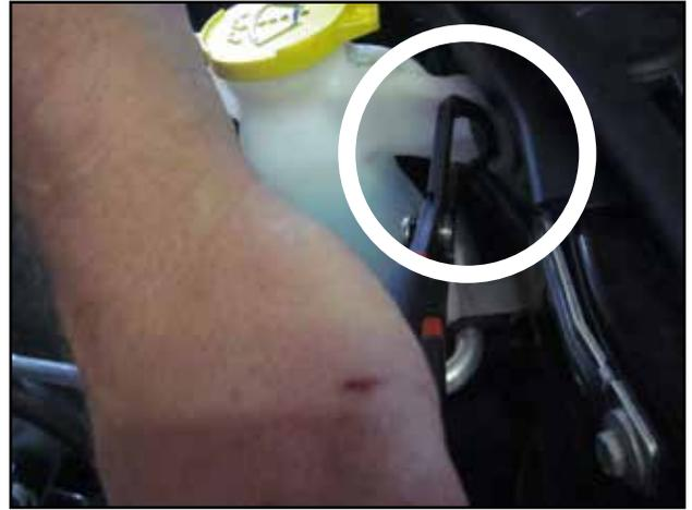
l. Remove the plastic clip securing the windshield washer fluid reservoir to the core support.
