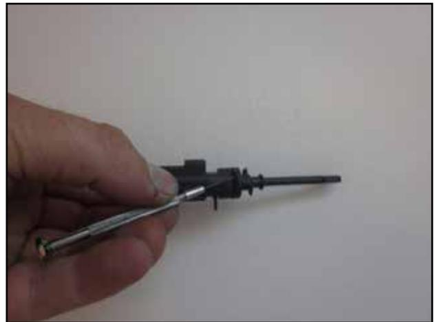
k. Once the IAT sensor is removed, use a suitable tool or pick to remove the small o-ring from the IAT sensor.
