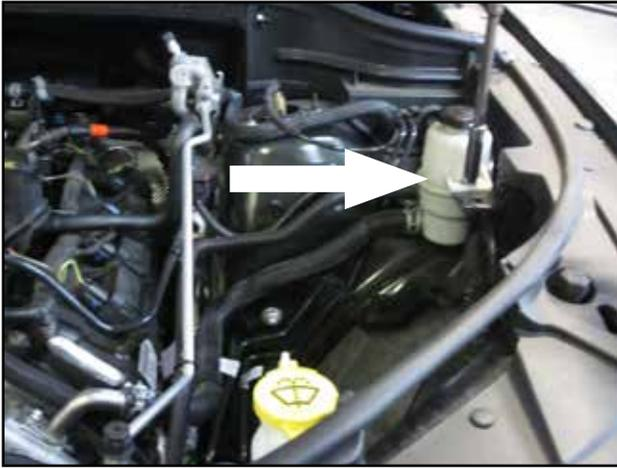
k. Loosen and remove the M8 bolt securing the power steering fluid reservoir. The bolt will be reused later.
