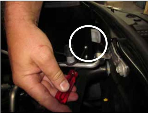
h. Attach the heat shield to the bracket installed in step 3-e) with supplied M6 bolts (L).
