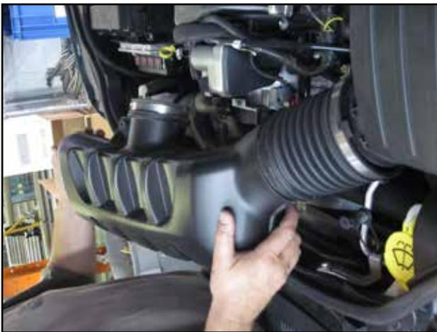
g. Remove the air inlet hose from the engine bay.
