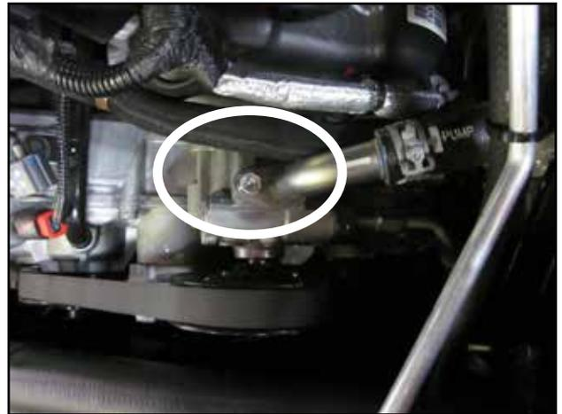
o. Loosen and remove the M8 bolt from the power steering pump housing. This bolt will not be re-used.
