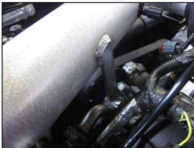
s. This is how the bracket should look when properly installed.
