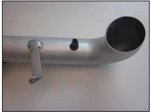
m. Insert the IAT sensor into the AEM air intake tube as shown.
