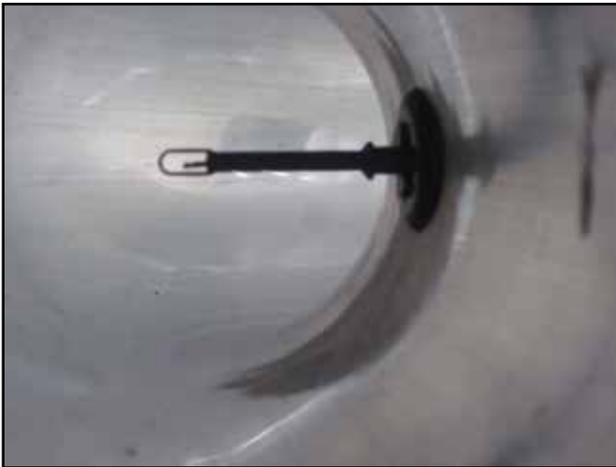
n. This is what the IAT sensor probe looks like inside the tube when sensor is properly inserted.
