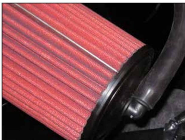
u. Install the elbow vent fitting (E) to the AEM air filter (D) top and attach the supplied 5/8" id hose (F) to the fitting.
