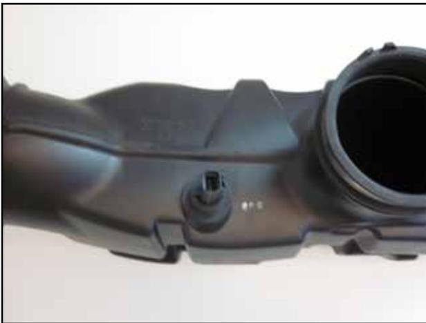
j. From the factory air inlet tube, twist and remove the IAT sensor.
