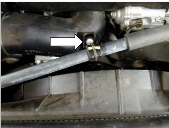
c. Remove the bolt retaining the stock AC line.
