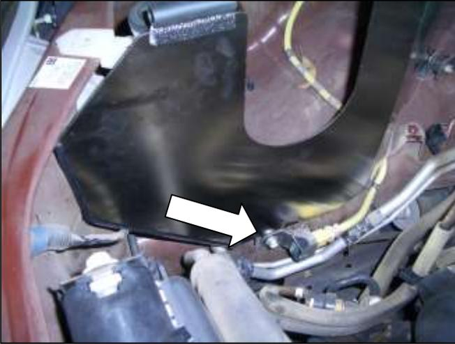
d. Remove the bolt securing the stock mounting tab. Insert the heat shield in place and use the stock bolt to secure in place.
