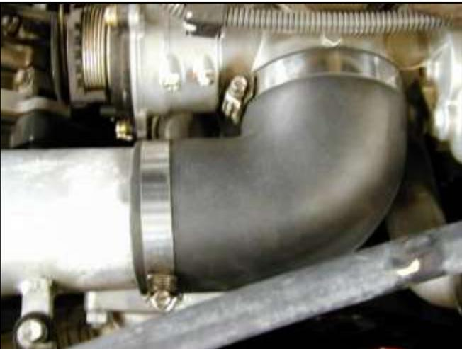
f. Install the rubber coupler on the throttle body and use the supplied #52 hose clamp to secure in place. Install the intake pipe in the other end of the rubber connector and secure in place using the supplied #48 hose clamp.
