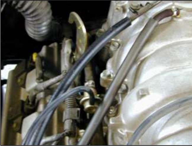
h. Install the 5/32" new hose on the fuel pressure regulator. Install the new 3/8" hose on the end of the exposed tube from the removal of the stock intake system if applicable. Use the 3/4 hose clamp to secure in place.
