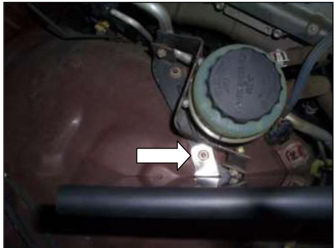
c. Install the heat shield mounting tab and use the stock nut to secure in place.
