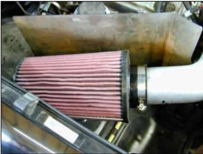
l. Install the air filter onto the end of the intake pipe and secure in place using the supplied hose clamp.
