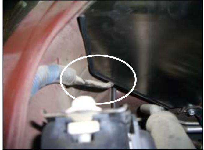
e. Relocate the stock wiring harness to the lower portion of the heat shield making sure it is free and clear.
