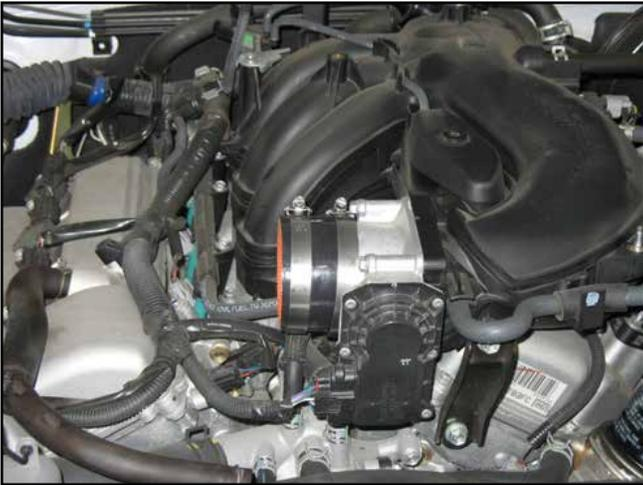
l. Install the coupler loosely at the throttle body using the supplied #48 hose clamps.
