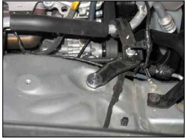
g. Place the supplied spacer on top of the A/C line bracket. Lining it up with the hole beneath it.
