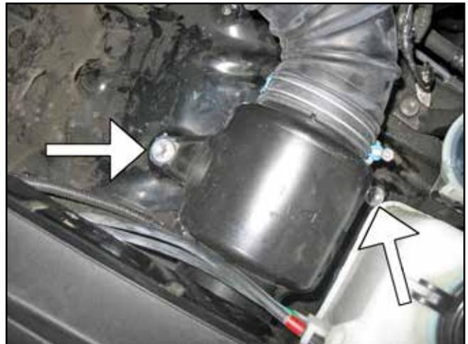
h. Remove the two bolts that secure the intake tube to the fender well.
