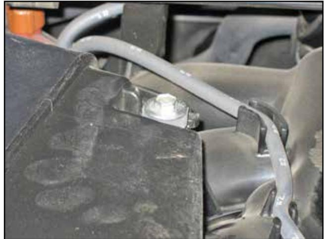
f. Remove the bolt securing the stock intake system to the intake manifold.
