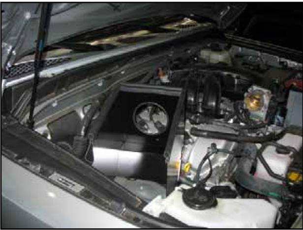
h. Prepare the heat shield with edge trim and rubber gasket then place in the engine bay as shown.
