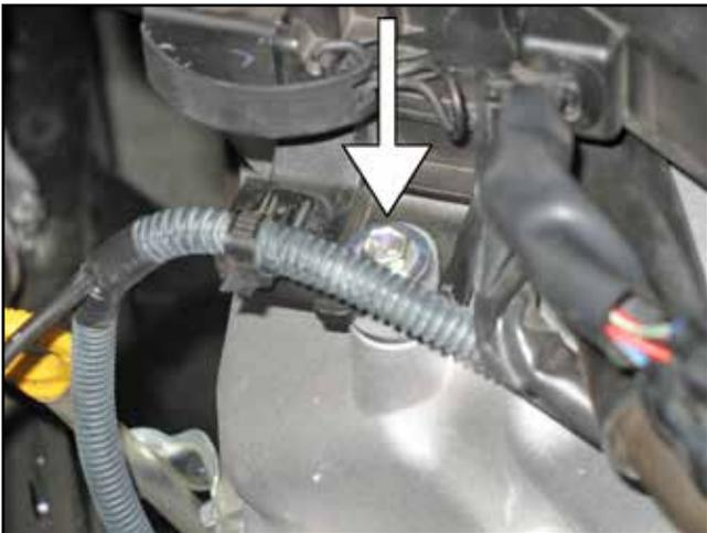
g. Remove the bolt securing the stock air box to the valve cover. Keep this bolt as it will be reused later. Also, disconnect the zip ties connected to the stock air box.
