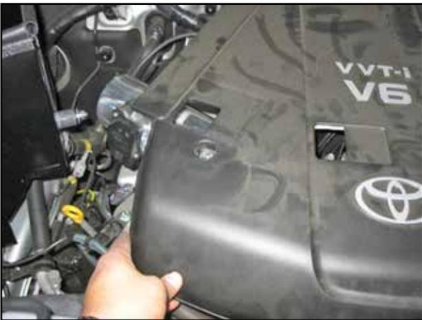
n. Line up the bolt that is attached to your upper intake pipe with the hole on the engine cover, then remove the engine cover again.
