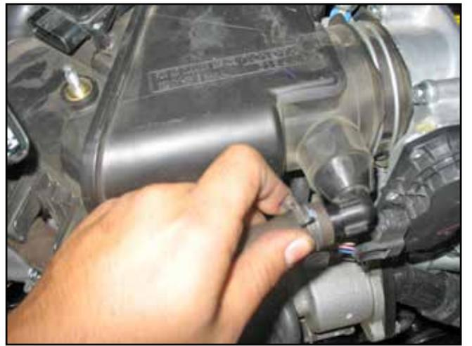
d. Disconnect the breather hose located in the front of the intake system.
