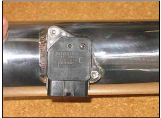
c. Install mass air flow sensor in pipe using supplied bolts.
