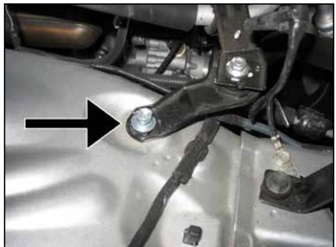
j. Remove the bolt securing the A/C line bracket.
