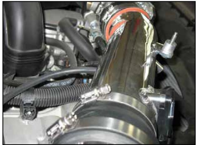
q. Attach the hose installed in step 3f. to the small nipple located on the back of the intake pipe.
