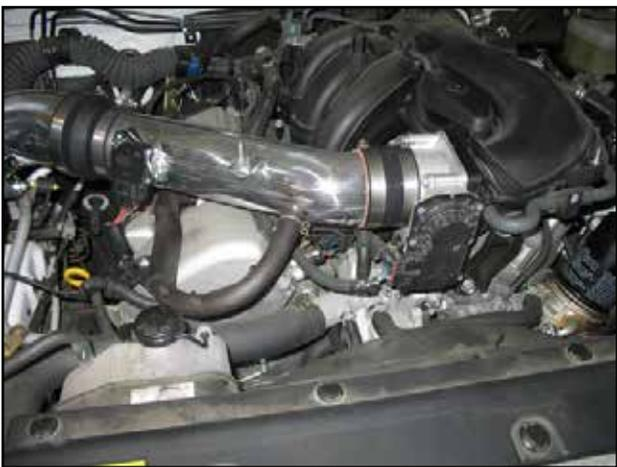
r. Reattach the PCV hose to the nipple on the upper pipe using the stock hose clamp. Also plug the MAF sensor back in.
