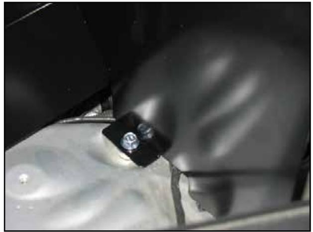
i. Line up the hole that is nearest to the front of the vehicle first. Then, run the supplied bolt through the heat shield and the spacer.
