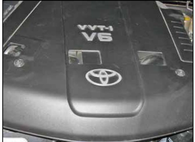
b. Remove two nuts securing the engine cover to the intake system and engine.
