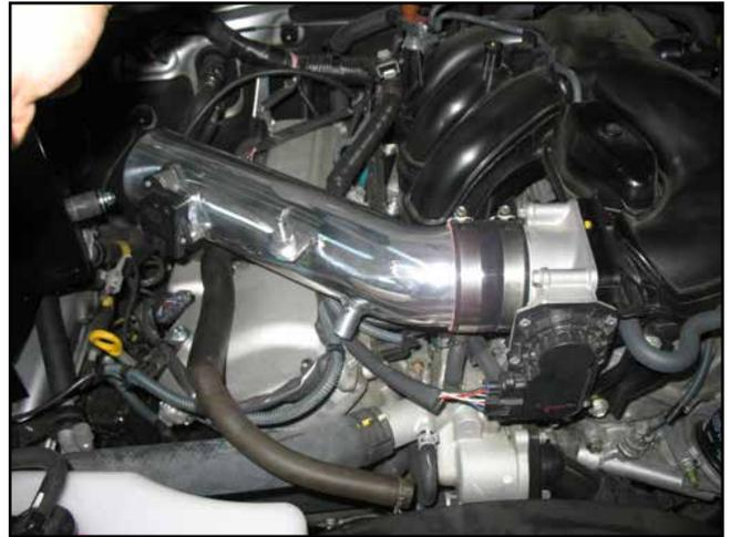
m. Insert the upper pipe into the coupler at the throttle body.
