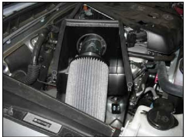
s. Install filter on the end of the lower pipe.
