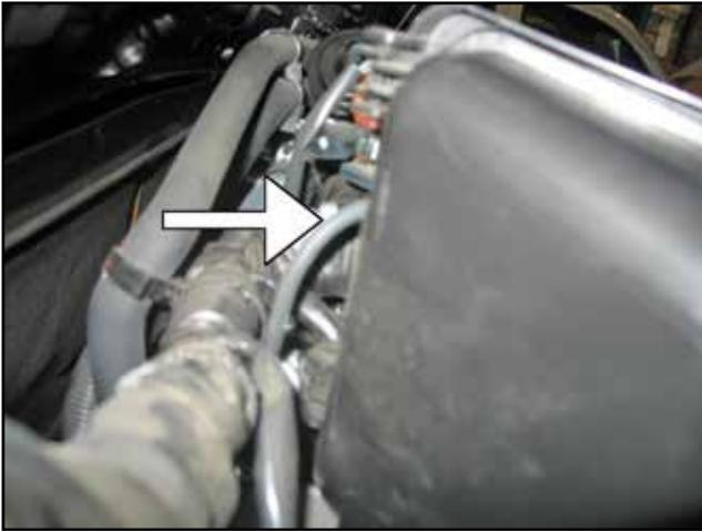
e. Disconnect the breather hose located in the back of the stock intake system connected to the fuel pressure regulator.
