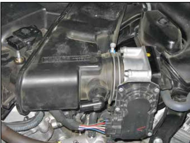
i. Loosen the hose clamp securing the stock air box to the throttle body.
