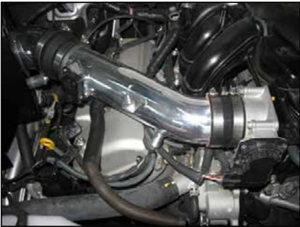
p. Use the supplied 8mm washer and serrated nut to secure the lower pipe to the rubber mount.
