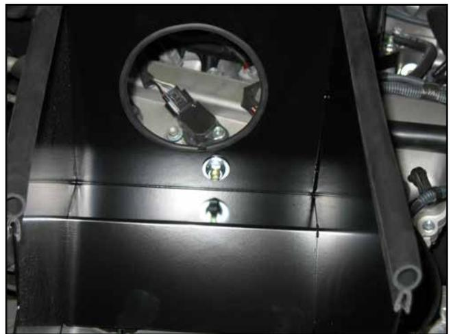
k. Install the rubber mount in the heat shield with the supplied 8mm washer and serrated nut.
