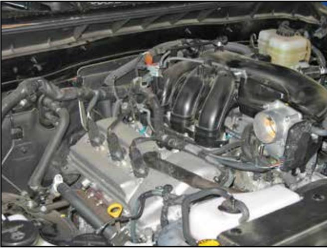
k. Factory air box completely removed from vehicle.
