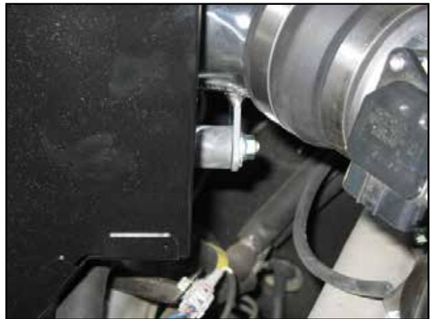
o. Install the screened hose adapter to the end of the upper pipe and guide the lower pipe through the heat shield, while lining up the bracket with the rubber mount as well.
