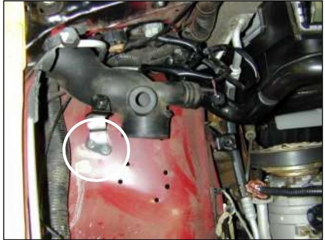
h. Remove the two bolts and the bracket circled in the picture.
