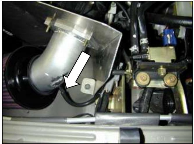
p. Install the included 3/16" hose between the connector on the pipe and the vacuum solenoid.
