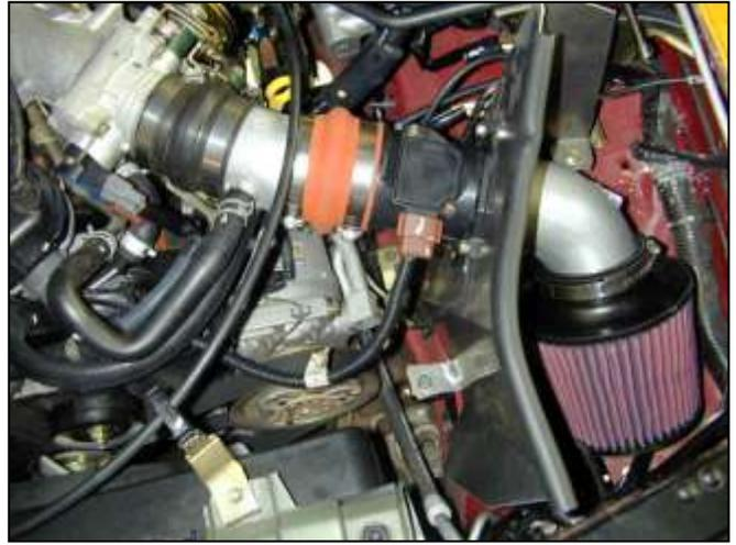
t. Check final fitment of the intake system and heat shield. Make sure no part of the intake system makes contact with the vehicle. After adjusting the position of the system, tighten down the mounting nuts on the heat shield and all of the hose clamps.
