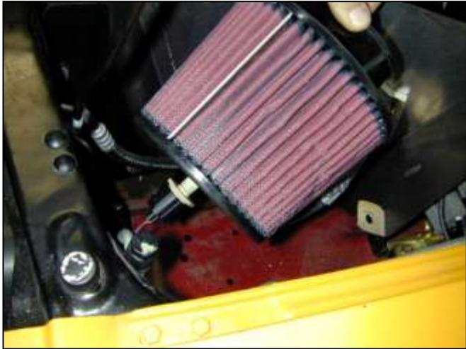
i. Insert the IAT sensor into the end of the air filter and plug in the sensor. Place the air filter and hose clamp on to the end of the intake pipe inside the heat shield. Make sure the air filter is fully inserted on the pipe and tighten hose clamp.
