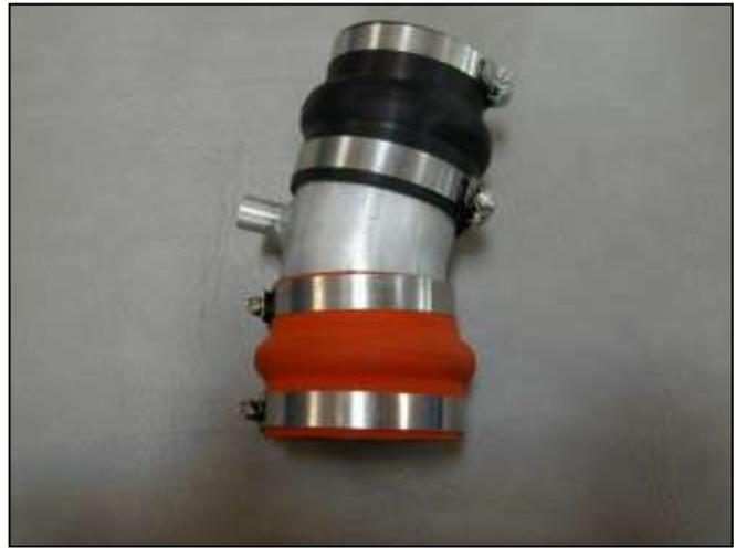
l. Place the 3" hump hose and #48 hose clamps around the other end of the pipe as shown.
