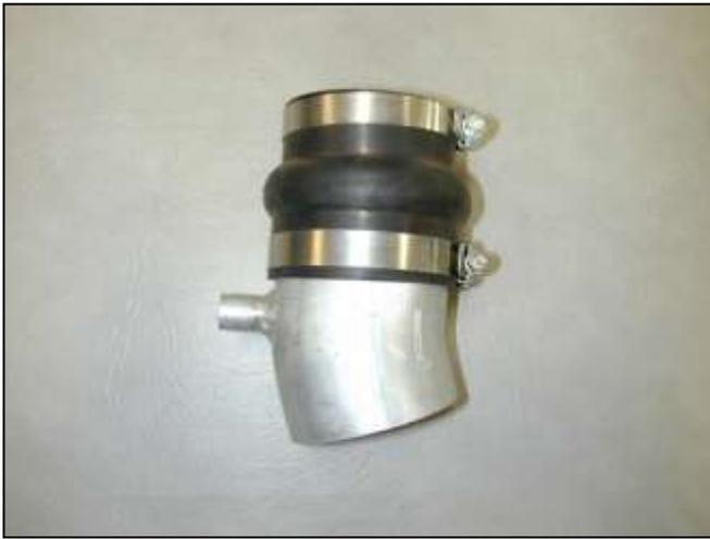
k. Insert the 2.75"-3.0" hump hose reducer on to the throttle body end of the pipe with the 3.0" end around the pipe. Use a #48 hose clamp for the 3" end and a #44 hose clamp around the 2.75" end.
