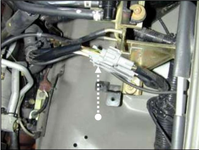
m. Bend the wire plug holders as shown in the picture, this will allow additional clearance for the heat shield.
