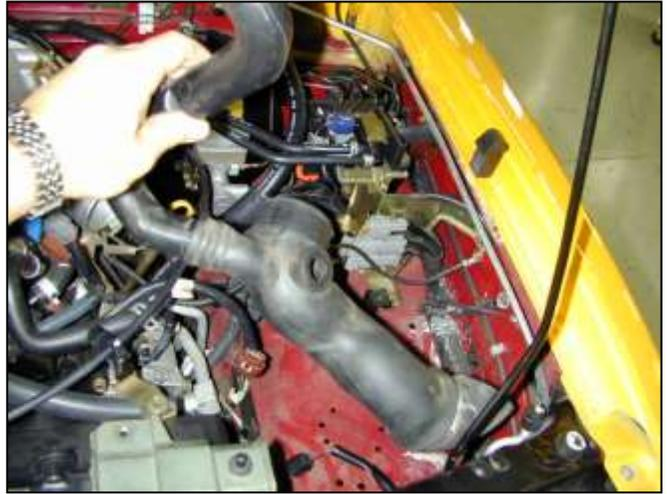
j. Unsnap the ducting assembly from the inner fender and remove it from the engine bay.
