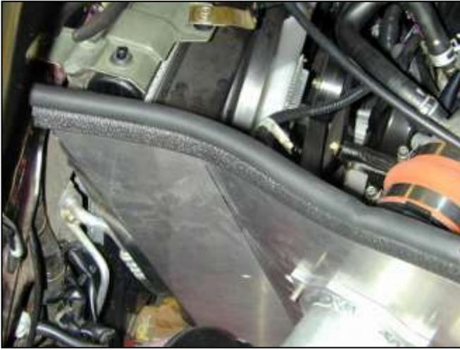
s. Push the molding onto the upper edge of the heat shield as shown in the picture.
