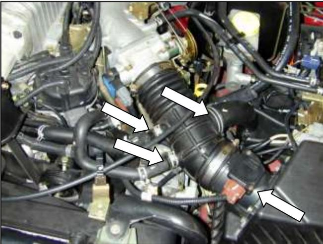
a. Disconnect the three hoses, pictured above, from the factory air inlet system. Unplug the Mass Air Flow (MAF) sensor and loosen the hose clamps around the throttle body and MAF sensor.
