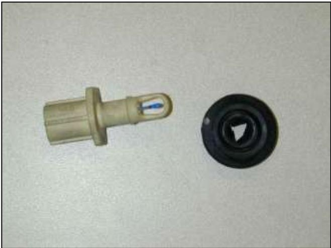
h. Remove the rubber grommet from the IAT sensor.
