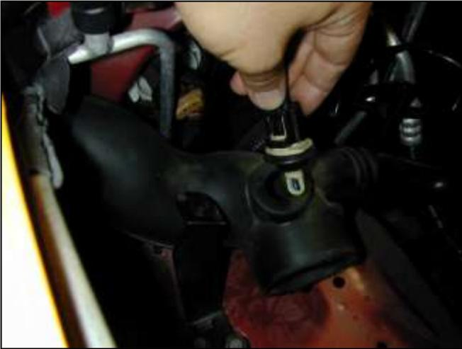
g. Remove the Intake Air Temperature (IAT) sensor from the plastic ducting as shown in the picture.
