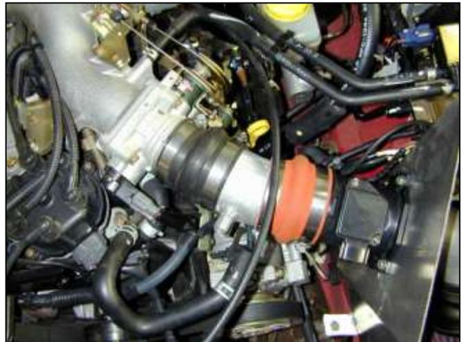
n. Place the assembly from the previous step into the vehicle with the 2.75" hose around the throttle body and the 3" end around the MAF sensor. Make sure the nipples are facing toward the front of the vehicle.
