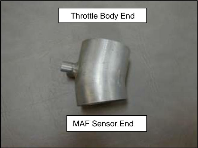
j. Orient the upper intake pipe as shown. The straight section is the end that will connect to the throttle body.
