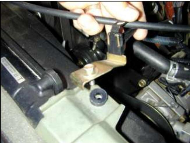
b. Place the supplied round spacer underneath the throttle cable bracket as shown. Secure the bracket in place by reusing one of the fasteners from step 2(i). Skip this step for normally aspirated vehicles.
