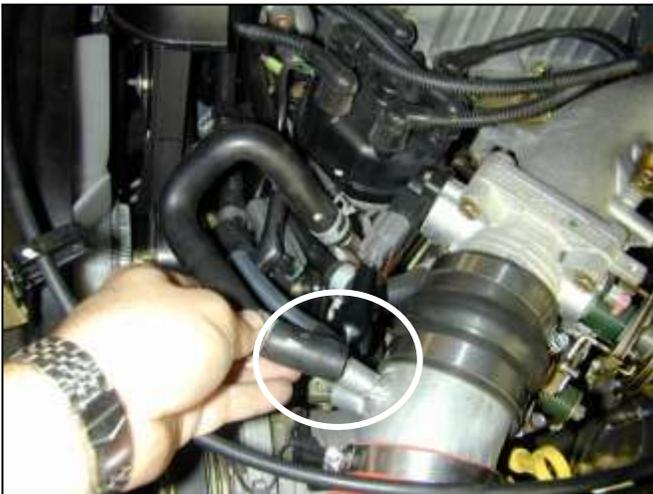
q. Plug the factory idle air hose onto the upper nipple and secure it in place by reusing the factory hose clamp.
