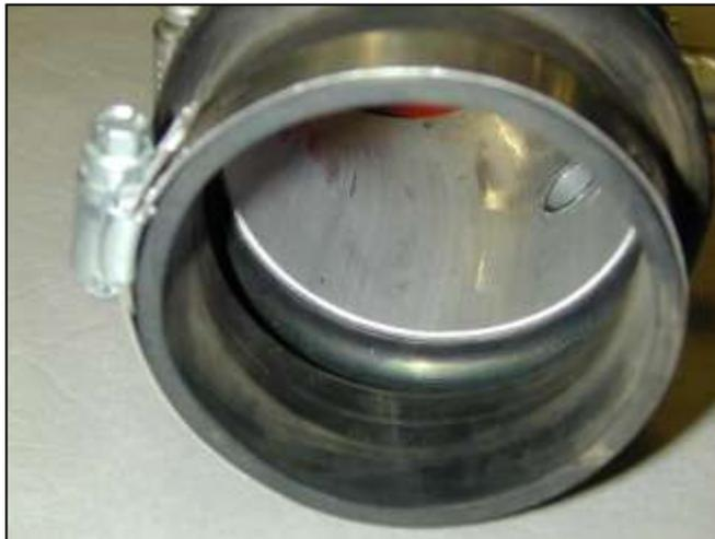
m. Push the hump hoses on only until the pipe reaches the hump as shown. Tighten the hose clamps around the 3" pipe.
