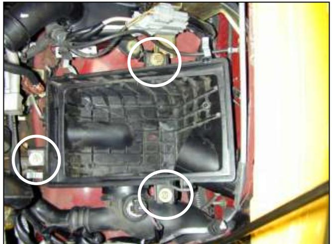
d. Remove the three bolts shown in the picture and remove the lower air box housing piece from the engine bay.
