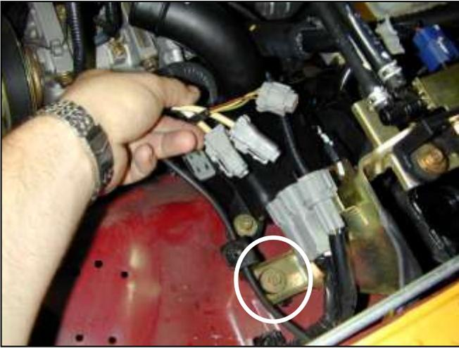
e. Remove the fastener circled in the picture. Unplug the three wiring connectors shown in the picture. This will allow easier access to the intake resonator chamber.
