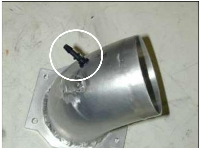
c. Insert the rubber grommet and vacuum hose connector into the small hole on the MAF sensor adaptor pipe. On vehicles not equipped with vacuum solenoid use vacuum cap to seal off vacuum hose connector first then install into grommet.
