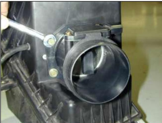
k. Remove the MAF sensor from the air box by removing the four mounting bolts.
