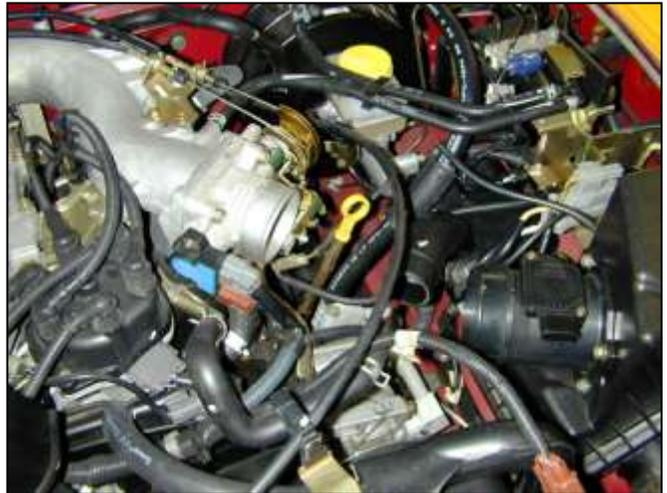
b. Remove the factory intake hose from the engine bay.
