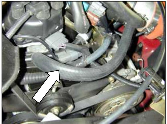
r. Use the included 5/8" ID hose and 1" hose clamps to connect the PCV tube to the lower nipple on the intake pipe.
