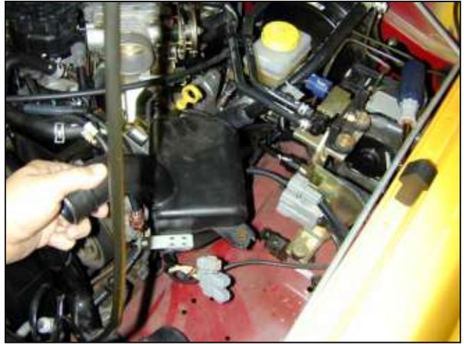
f. Remove any wiring harnesses attached to the resonator chamber and remove from the engine bay. PLUG IN THE WIRES that were unplugged in the previous step after the chamber was removed.
