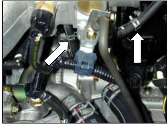
j. Closer view of tubing loom routing. Use pliers to slide the spring clamps over the breather and coolant hoses. A flat-head screwdriver may be needed to pry the hoses off the coolant line nipples.
