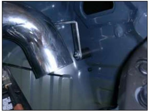
g. Guide the bracket on the intake pipe over the stud on the rubber mount. Once aligned, install the supplied washer and nylok nut onto the stud. Do not tighten until fitment is complete.
