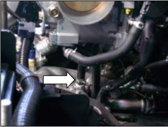
i. **CAUTION: Ensure the engine is completely cool before removing the coolant hose, or hot coolant will escape from the cooling system and cause injury or damage. Be sure to capture any lost coolant in a clean container.**
