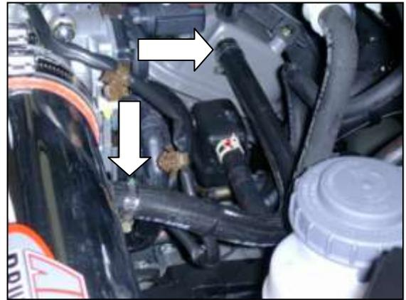
i. Install the supplied ½" breather hose between the intake pipe and the valve cover as shown. Use the supplied 1" hose clamps to secure. Secure the TBM wire harness to the valve cover breather hose using the supplied zip tie.
