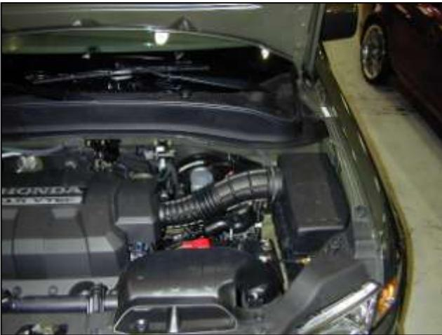
Stock air box system installed
