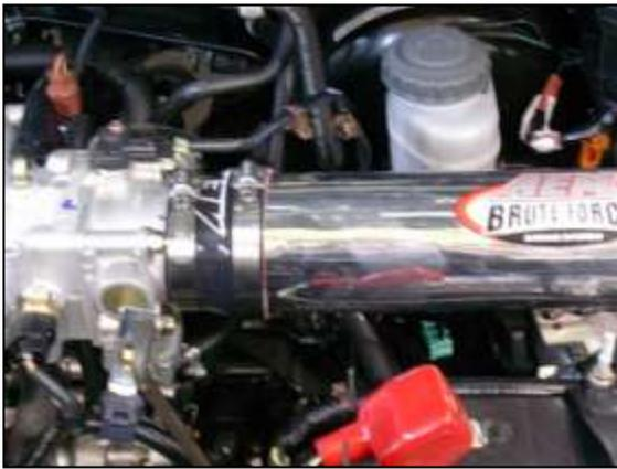
f. Install the AEM® intake pipe into the previously installed coupler.
