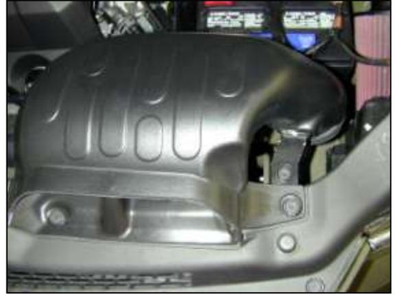
k. Install the stock air inlet duct using the three plastic connectors previously removed.
