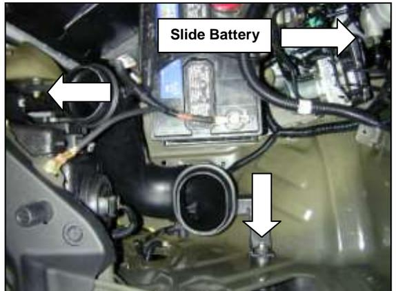
h. Remove the two bolts securing the lower inlet tube to the truck body. In order to remove the tube, loosen the battery hold down brackets and slide the battery forward for clearance. Once the inlet tube is removed, move the battery back to its original location and secure.
