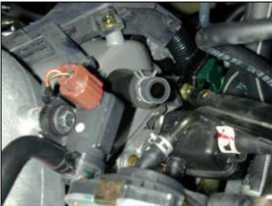
k. Remove the short rubber hose attached to the valve cover breather nipple.
