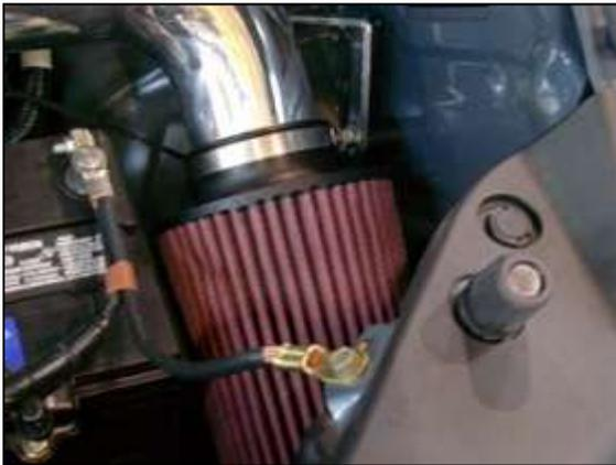
h. Install the AEM® air filter on to the end of the inlet tube. Push the air filter over the inlet pipe until the stop in the air filter is reached. Once proper fitment is achieved, install the supplied hose clamp to secure the filter onto the inlet pipe.
