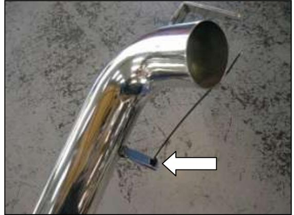
c. Check to see that the inside of the inlet pipe and air filter are clean and free from any foreign objects and/or obstructions. Install the supplied push in zip tie in the bracket as shown.
