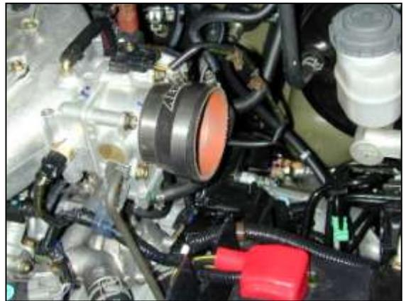
e. Install the silicone reinforced adapter over the throttle body and secure using a # 48 hose clamp.
