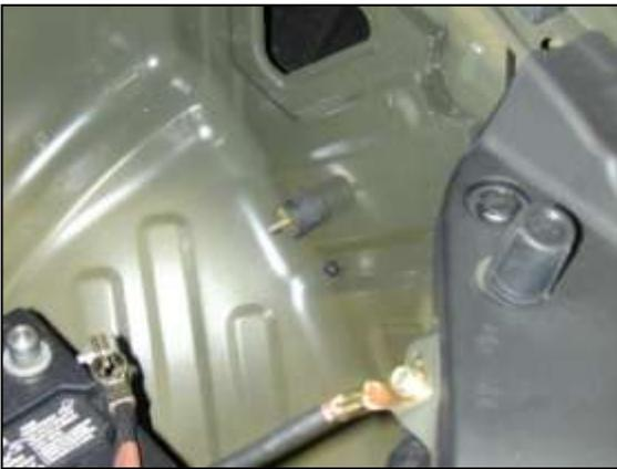
d. Install the rubber mount where the lower inlet tube was previously removed.
