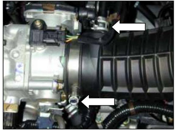
f. Loosen the hose clamp on the throttle body. Remove the valve cover breather hose from the air inlet pipe by compressing the flanges on the retaining clip and sliding the hose out.
