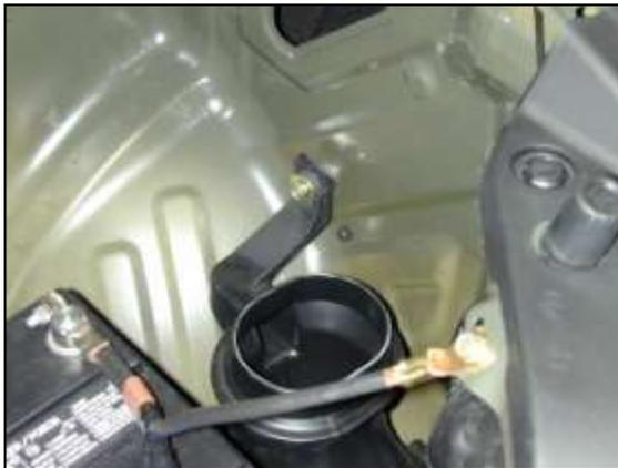
g. Remove the remaining bolt securing the air box to the chassis. Carefully remove the air box from the vehicle by lifting it straight up off the lower inlet tube.
