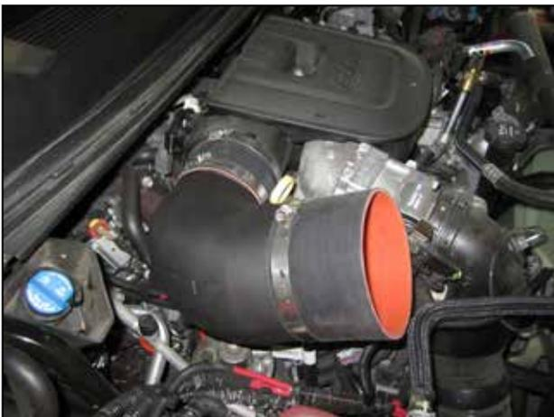
d. Loosely install another hose clamp (9472) over the outlet hose and install the intake elbow assembly onto the engine intake port as shown. Do not fully tighten the hose clamp yet.
