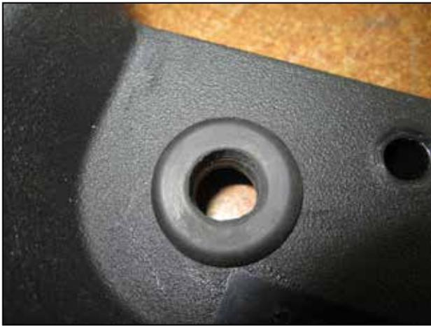
x. Install the grommet (784642) into the 0.75" hole in the corner of the air box lid (9-0411) as shown.
