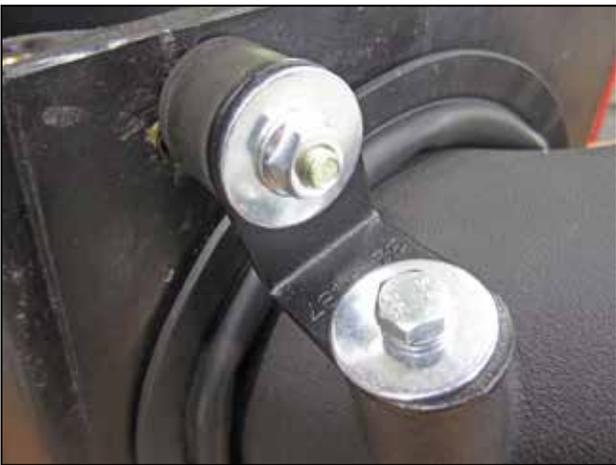
t. Install one flat washer (08160), one split washer (1-3025), and one M6 hex bolt (1-2065) through the "L" bracket slot and into the mounting boss in the lower intake tube (9-0405). Tighten the bolt and the hex nut with a 10mm socket.
