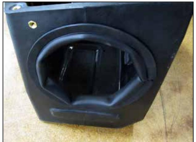
e. Install the bulb seal (102494) around the inside edge of the outlet hole of the air box (9-0406) as shown. Trim any excess bulb seal as needed.
