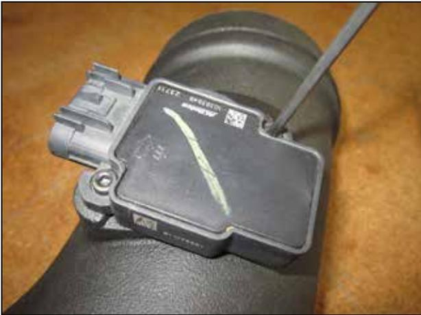
b. Install the MAF sensor onto the MAF pad on the lower intake tube (9-0405). Secure with the two 4mm Allen bolts provided. Tighten the bolts.
