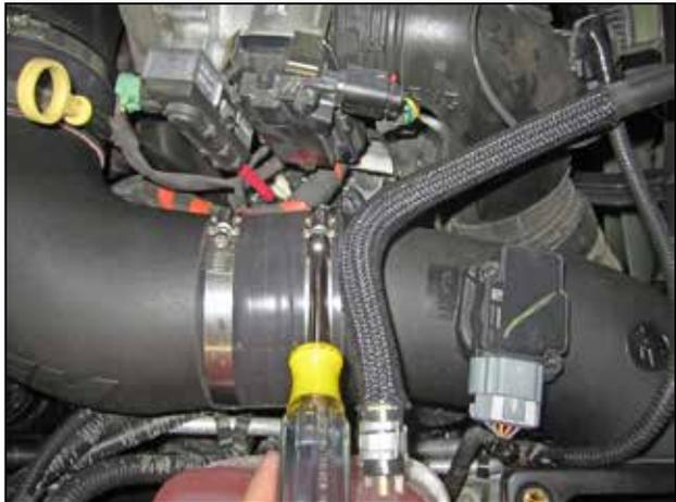
q. Install the fourth hose clamp (9472) on the open silicone hose already mounted on the intake elbow. Insert the outlet end of the lower intake tube (9-0405) into the silicone hose. Loosely secure the hose clamp so the intake tube can rotate inside the hose.
