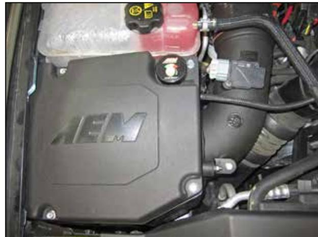
aa. Install the air box lid (9-0411) onto the air box (9-0406) as shown using the M6 hex/flare bolts (1-1016) provided. Start all 4 bolts by hand first and then tighten them with a 10mm socket to seal the air box.
