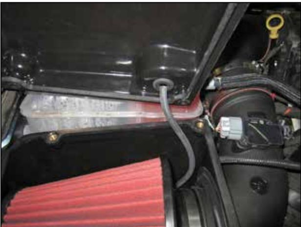
z. Guide the loose end of 5/32" air hose already attached to the filter cap onto the small port of the filter minder gauge through the air box lid as shown.
