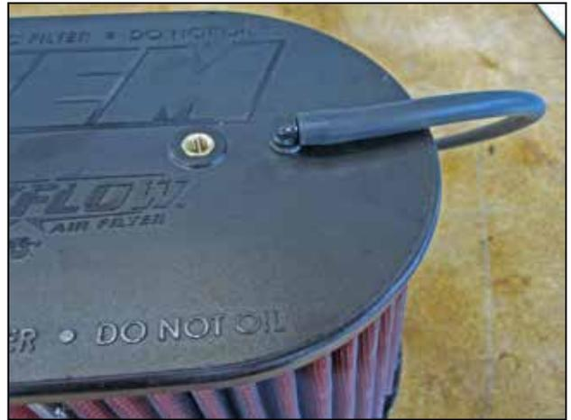
k. Install the small grommet (784631) into the drilled hole, and then install the 5/32" plastic elbow port (8-152) into the grommet. Install the 5/32" rubber air hose (5-3018) onto the elbow port as shown. This hose will be attached to the AEM® Filter Minder gauge at a later step.
