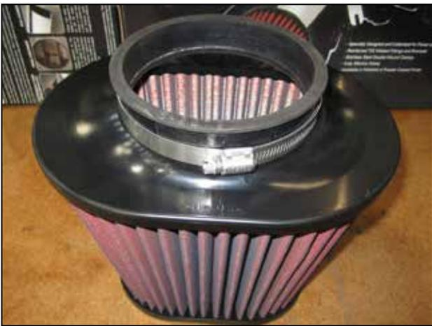
l. Install the filter insert (5-2279) into the outlet of the Dryflow™ air filter. Install the large hose clamp provided over the air filter outlet as shown.
