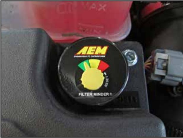
ab. Make sure the AEM® filter minder gauge needle is pointing to the green sector. Once your Dryflow filter is dirty and the pressure drop (restriction) across it reaches 20 inches (of H<sub>2</sub>O), the gauge needle will point to the red sector. This will mean it is time to wash your reusable AEM® Dryflow™ air filter.
