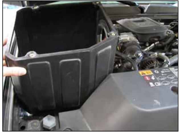
g. Place the air box into the engine bay where the stock air box was located as shown. Make sure the new left front mounting grommet is aligned with the threaded hole in the engine bay.
