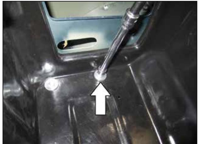
i. Install the third M6 bolt (1-2044) with a flat washer (08160) in the remaining mounting hole near the inlet window and tighten. Note that the large air inlet window is aligned with the smaller stock air inlet window in the vehicle fender.
