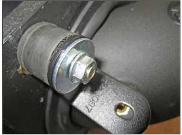
s. Loosely install the "L" bracket (32-3087), one flat washer (08160), and one M6 serrated nut (444.460.04) onto the rubber mount.
