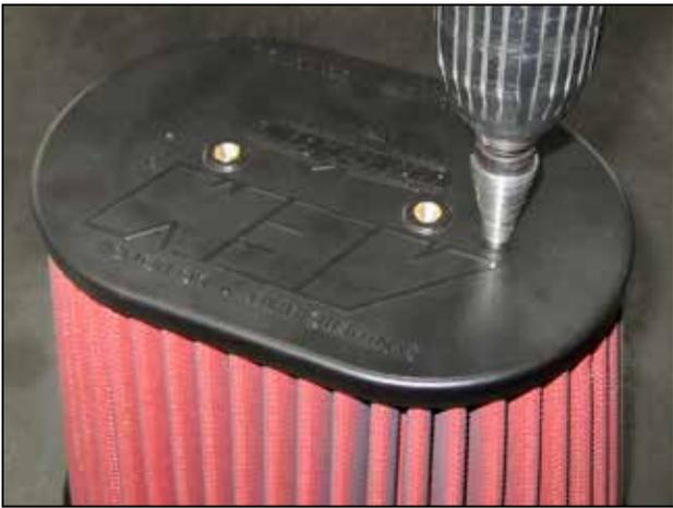
j. **Port Installation for AEM® filter minder gauge:** Drill a 1/4" diameter hole in the plastic cap of the Dryflow™ air filter at the dimpled location as shown. **Clean out all plastic shavings from the inside of the filter.**
