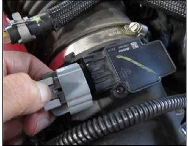
b. Depress the snap tab on the connector as shown and pull it to disconnect the harness from the MAF sensor.
