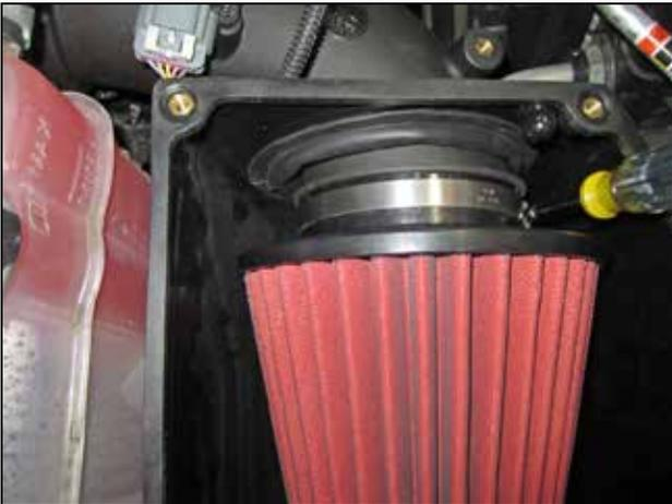
p. Fully seat the Dryflow air filter onto the lower intake tube inlet and align it inside the air box as shown. Tighten the large hose clamp at the filter base.
