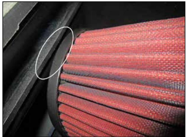
u. Rotate the lower intake tube and filter assembly until the edge of the filter cap lines up with the top edge of the air box opening near the fender as shown.
