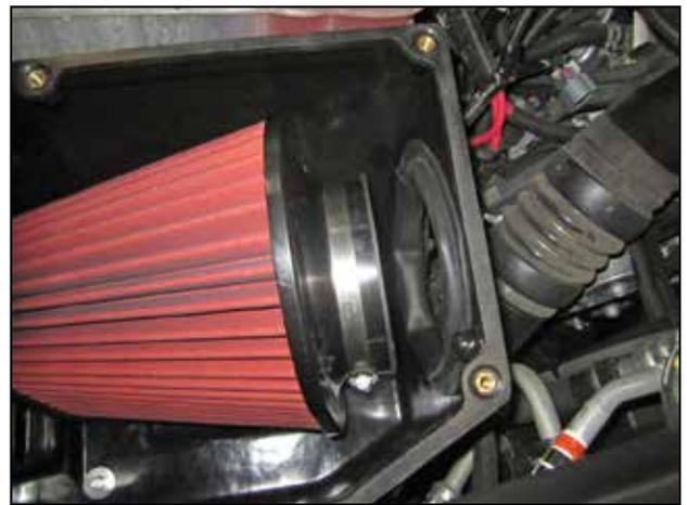
m. Insert the Dryflow™ air filter assembly into the air box as shown.
