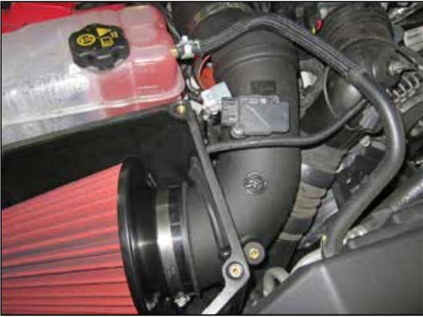
n. Loosely install the (9-0405) lower intake tube through the bulb sealed outlet hole in the air box and into the Dryflow air filter base adapter as shown.
