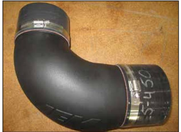
c. Install the silicone hose (5-1066) onto the outlet end of the intake elbow (9-0412), on the "A" side of the AEM® logo. Install the larger silicone hose (5-450) onto the inlet side of the intake elbow, the end closest to the "M" in the AEM® logo. Secure both couplers with (9472) hose clamps as shown.
