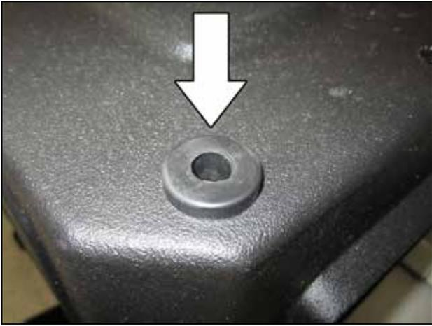
f. Install the foot grommet (784647) on the outside of the air box in the larger left front mounting hole as shown.
