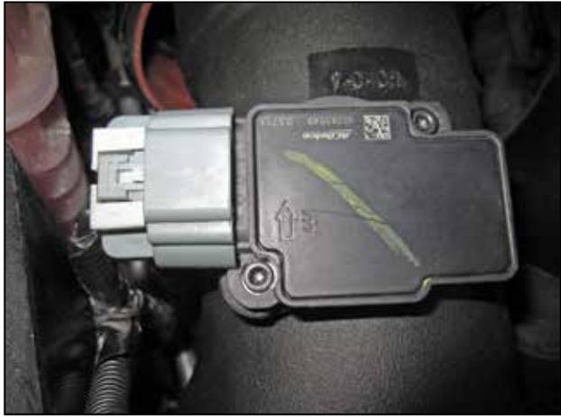
o. Connect the MAF harness to the MAF sensor and push the locking tab in to lock the connector.
