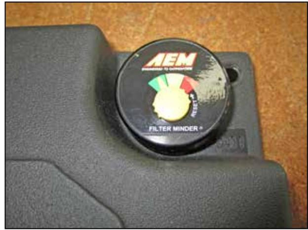
y. Install the filter minder gauge (35-80321) into the large grommet. Use glass cleaner to lubricate the hole in the grommet if needed.
