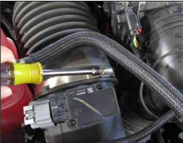
c. Loosen the 2 hose clamps retaining the stock intake tube.
