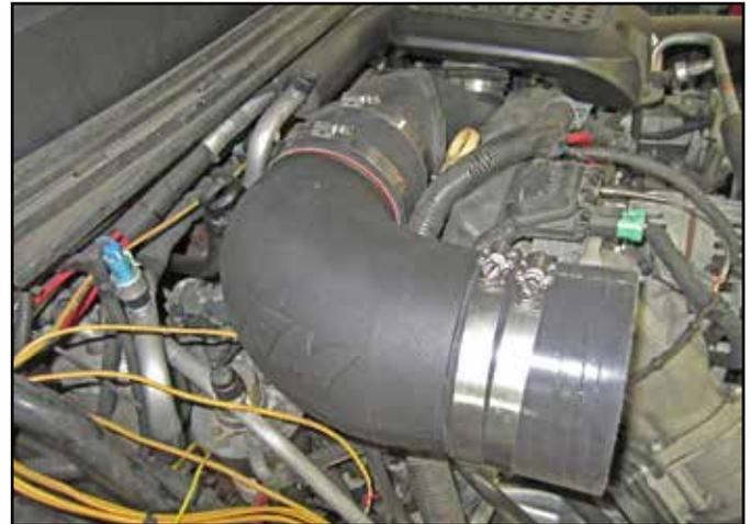
d. Install a #9472 hose clamp over the outlet hose and install the intake tube assembly onto the engine intake port as shown. Do not fully tighten the hose clamp.
