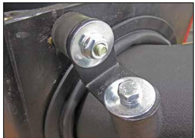
t. Install one flat washer, the split washer, and the M6 X 12mm hex bolt through the "L" bracket slot and into the mounting boss in the 9-0427 lower intake tube. Tighten the bolt and hex nut with a 10mm socket.
