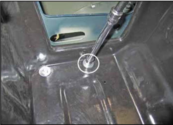
i. Install a M6 X 25mm bolt with a flat washer in the remaining mounting hole near the inlet window and tighten the bolt. Note that the large air inlet window is aligned with the smaller stock air inlet window in the vehicle fender.
