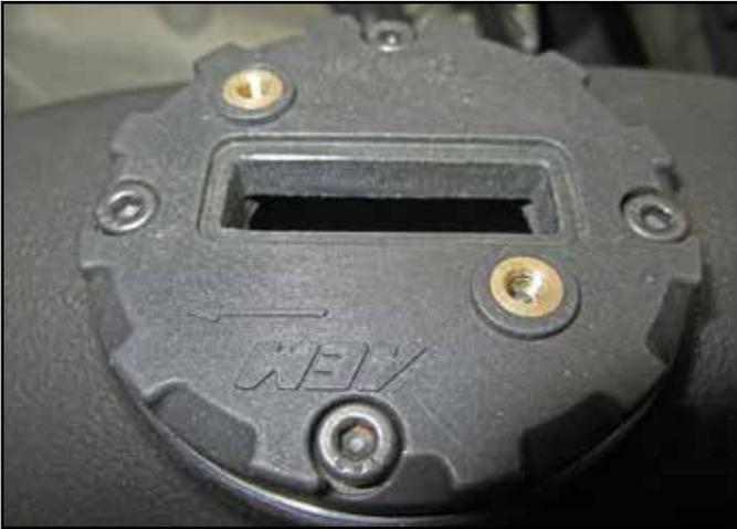
a. Install the mass air sensor adapter plate and O-ring seal in the 9-0427 lower intake tube using the four 4mm allen bolts provided.
