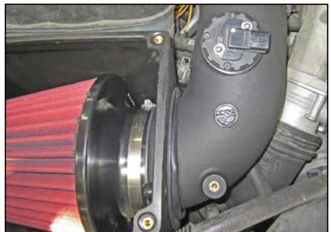
n. Loosely Install the 9-0427 lower intake tube through the bulb seal and into the air filter assembly as shown.
