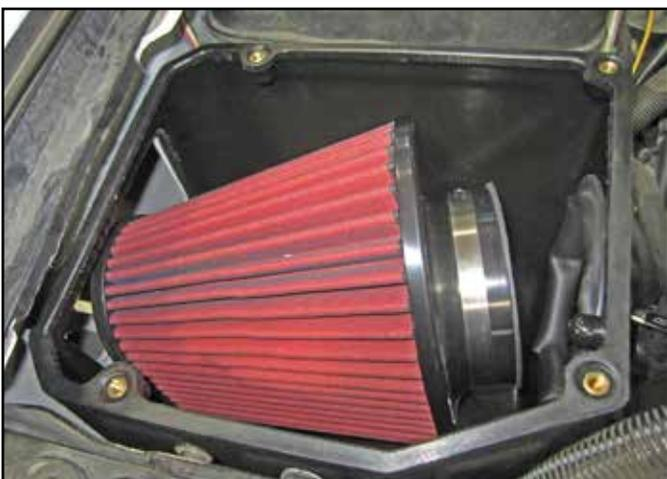
m. Place the AEM® Air Filter assembly into the air box as shown.
