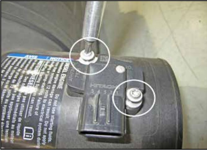
e. Using a T20 Torx bit, remove the two screws retaining the mass air sensor to the upper air box lid and remove the mass air sensor. Ensure the O-ring seal is still intact.
