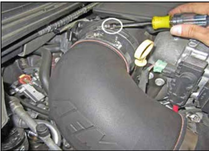
w. Fully seat the silicone hose at the engine intake port and tighten the hose clamp.
