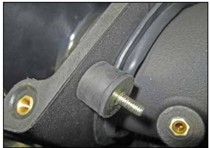
r. Install the 1228598 rubber isolator stud mount into the 6mm insert on the side of the airbox as shown. Tighten by hand.
