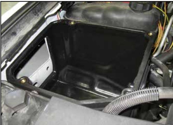
g. Place the air box into the engine bay into the stock location as shown. Ensure the new left front mounting grommet is lined up with the threaded hole in the engine bay.
