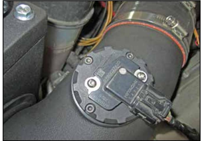
b. Install the mass air sensor on the mass air sensor adapter plate using the two buttonhead allen bolts provided.
