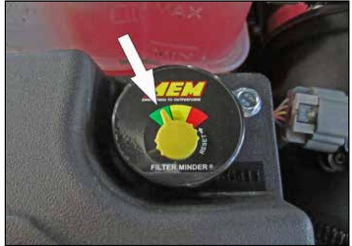
ab. Ensure the AEM® air filter minder gauge needle is pointing the green sector for the new AEM® Air Filter. Once the air filter is very dirty and the pressure drop (restriction) across it reaches 20 (inches of H<sub>2</sub>O) the gauge needle will point to the red sector. This will mean it is time to wash the re-usable AEM® air filter.
