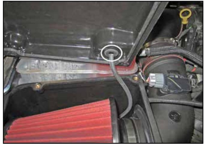
z. Mount the loose end of the 5/32" hose already attached to the air filter cap onto the small port on the air filter minder gauge under the air box lid as shown.
