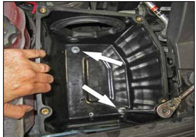
h. While pulling the air box toward the stock coolant reservoir to align the air box, install two M6 X 25mm bolts with two flat washers at the two mounting holes shown. Ensure the air box inlet window is aligned with the stock air inlet window in the sheet metal fender liner. Tighten the two bolts.
