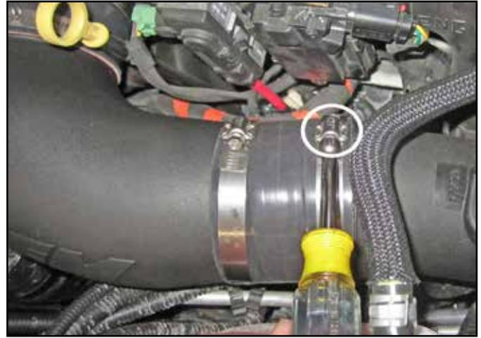
v. Tighten the hose clamp at the silicone hose connecting the upper and lower intake tubes.
