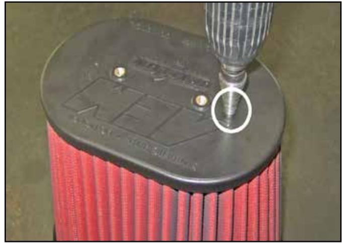
j. Drill a 1/4" diameter hole in the plastic cap of your new 21-2258DK AEM® Air Filter at the dimpled location as shown. **Clean out all plastic shavings from the inside of the air filter.**
