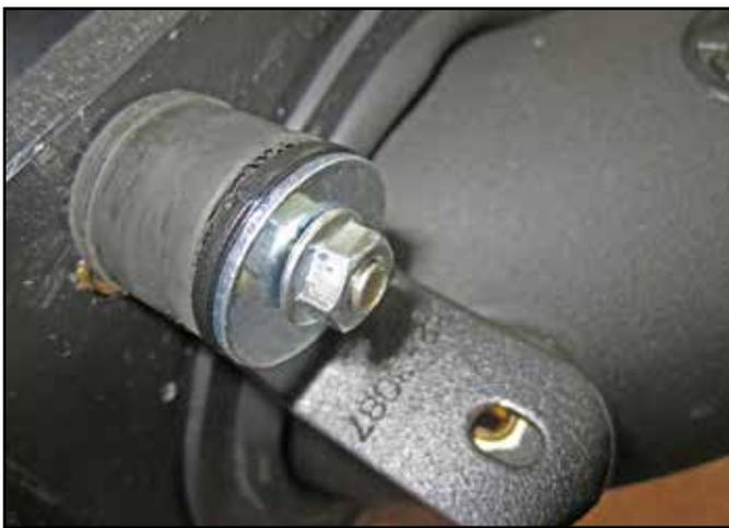
s. Loosely install the 32-3087 "L" bracket, one flat washer, and the 6mm serrated nut onto the isolator stud mount.
