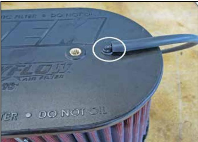
k. Install the 784631 grommet into the drilled hole, then install the 5/32" plastic elbow adapter into the grommet. Install the 5/32" rubber hose into the elbow adapter as shown. This hose will attach to the AEM® air filter minder gauge in a later step.
