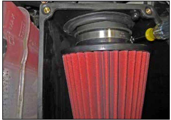
p. Fully seat the AEM® air filter onto the lower intake tube inlet and align it vertically as shown. Tighten the hose clamp at the air filter base.
