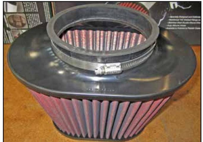
l. Install the large hose clamp provided onto the 21-2258DK AEM® DRYFLOW® Air Filter; then, Install the 5-2279 air filter base adapter into the outlet of the AEM® DRYFLOW® Air Filter.
