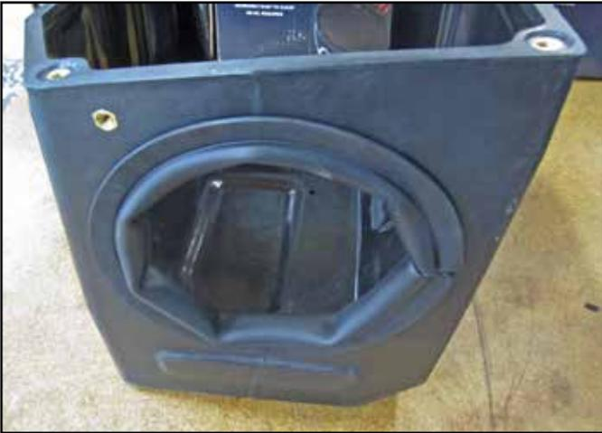
e. Install the bulb seal around the inside of the outlet hole on the 9-0406 air box as shown. Trim excess as needed.
