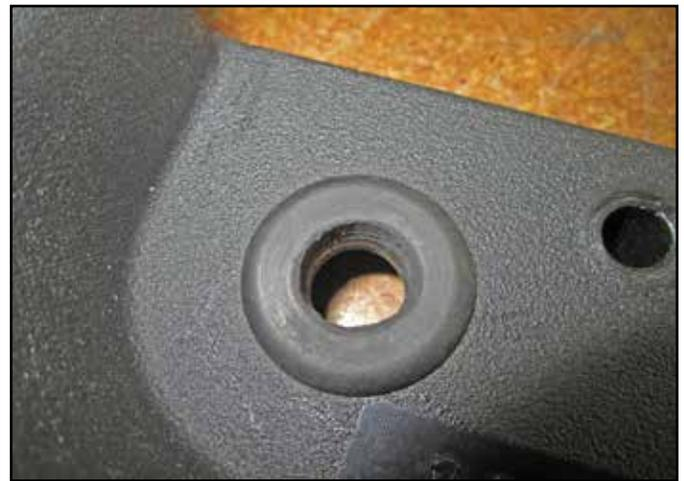
x. Install the 784642 grommet into the 3/4" hole in the corner of the 9-0411 air box lid as shown.
