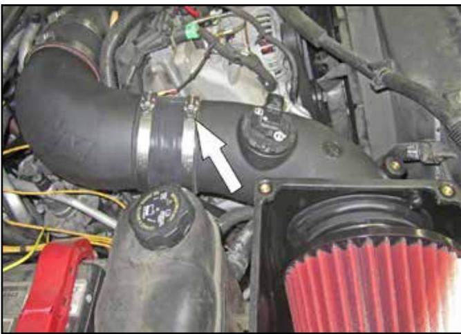
q. Install a #9472 hose clamp on the silicone hose already mounted on the intake tube elbow. Install the 9-0427 lower intake tube into the silicone hose. Do not fully tighten the hose clamp.
