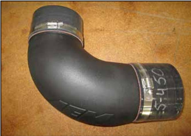
c. Install the 4.25 X 2.5" silicone hose onto the outlet of the 9-0412 intake tube, on the "A" side of the AEM® logo. Install the 4.5 X 3" silicone hose onto the inlet side of the intake tube, on the "M" side of the AEM® logo. Secure both silicone hoses with the #9472 hose clamps as shown.
