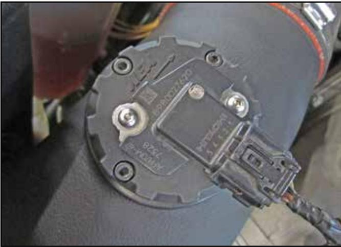
o. Re-connect the mass air sensor, fully seating the connector to lock it.
