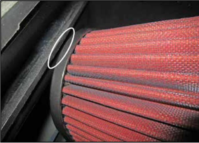
u. Rotate the lower intake tube and air filter assembly until the edge of the air filter cap lines up with the top edge of the air box opening near the fender as shown.
