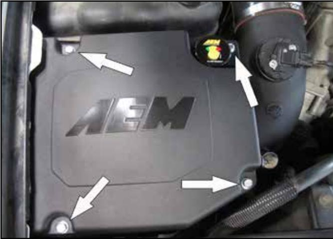
aa. install the 9-0411 air box lid onto the 9-0406 air box using the provided 6mm hex bolts. Tighten all bolts by hand first, then tighten with a 10mm socket to seal the air box.
