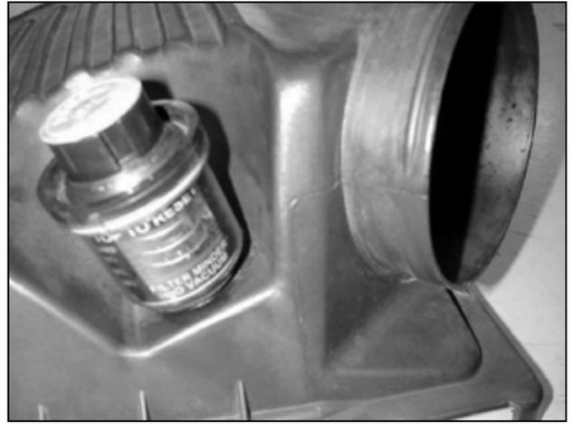
f. Remove the factory air filter restriction gauge from the stock air filter housing lid. Set aside for use during the AEM® intake kit installation.
