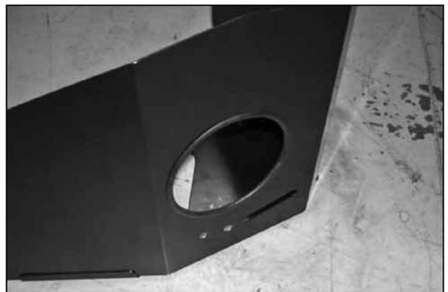
f. Install the supplied rubber edge trim to the hole on the heat shield. Trim to fit.
