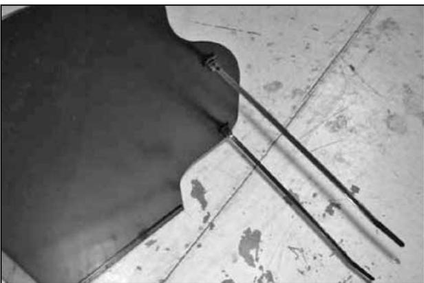
e. Install the two supplied tree mount zip-ties into the two holes on heat shield as shown.
