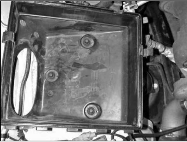
e. Loosen the three plastic nuts securing the lower air filter housing to the vehicle. Remove the housing by gently lifting up.
