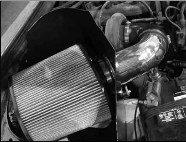
s. Slide the hose clamp onto the air filter's neck and attach the air filter assembly onto the filter adapter. Ensure the air filter is completely seated onto the adapter and the hose clamp is aligned with the filter adapter's lip. Once the hose clamp is properly aligned, secure the hose clamp, ensuring the filter neck's tabs compress and engage the filter adapter. Ensure the air filter does not make contact with any part of the vehicle and has adequate clearance.
