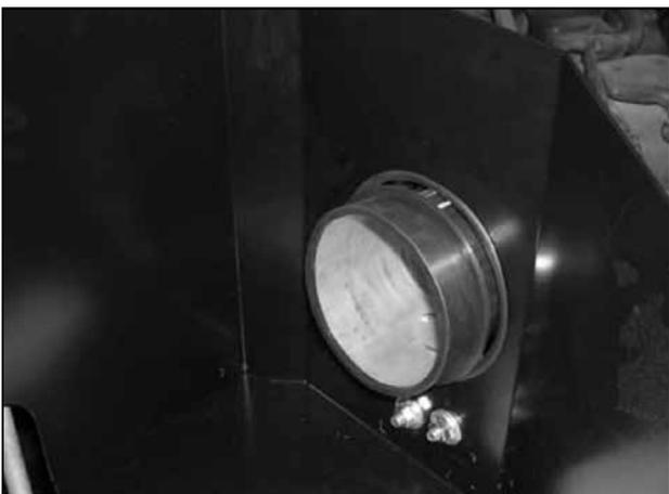
q. Install the supplied air filter adapter by stretching it over the end of the intake pipe.
