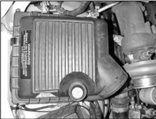
c. Release the four retaining clips securing the air filter housing lid to the lower housing. Remove the lid.
