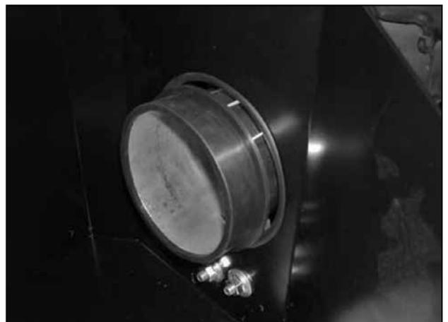
r. Ensure the intake pipe is centered in the heat shield hole. Once properly aligned, completely tighten the nuts on the intake pipe bracket and the hose clamps securing the intake pipe.
