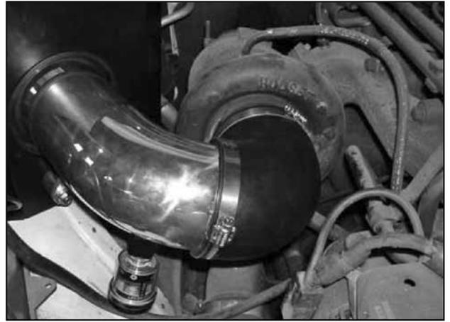
n. Install the intake pipe by sliding the long end of the coupler over the turbo inlet while aligning the mounting bracket of the intake pipe with the two rubber mounts attached to the heat shield.
