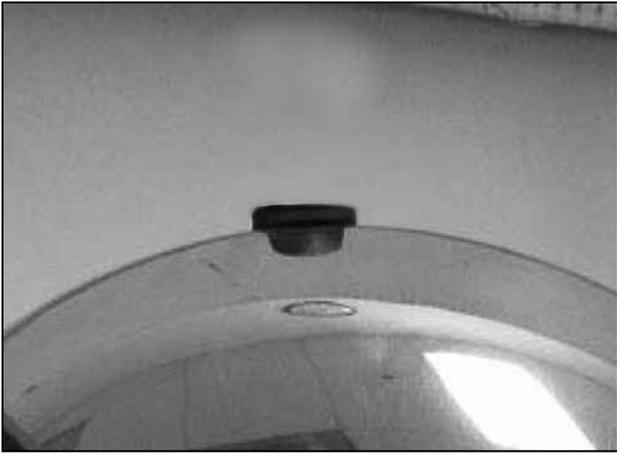
m. Install the grommet (784646) onto the intake pipe (use soapy water to aid installation). Place the grommet into the pipe at an angle and rotate it until the groove engages the pipe. Insert the filter minder gauge into the grommet.
