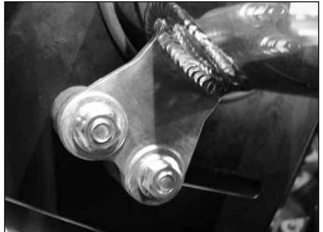
p. Secure the intake pipe mounting bracket to the heat shield using the supplied M8 washers and nuts.
