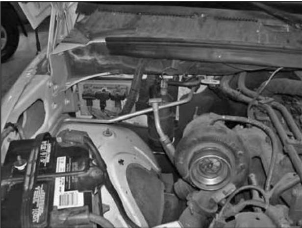
c. Stock air box system removed.
