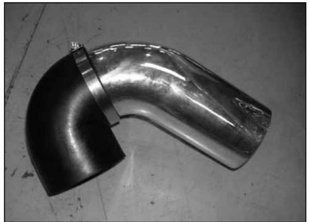
l. Loosely install the 90° coupler onto the short end of the intake pipe as shown. Attach a #64 hose clamp, but do not tighten the hose clamp.
