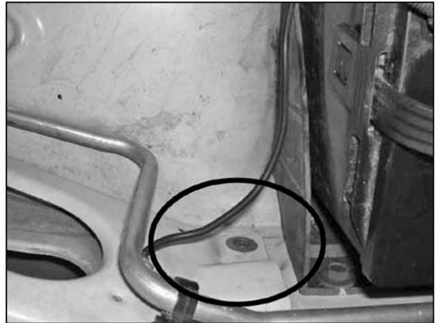
d. Remove the 13mm bolt from the inner fender behind the passenger side battery as shown.
