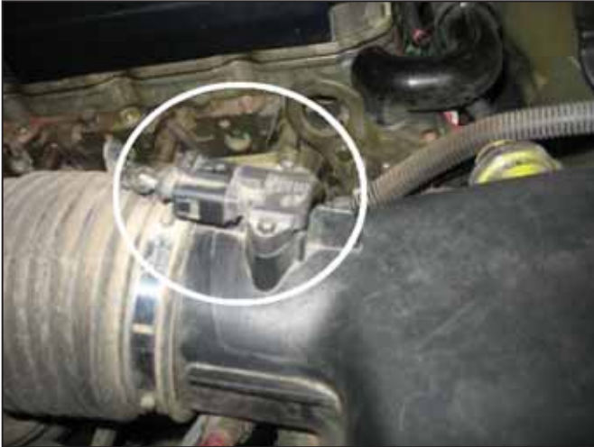
a. Stock airbox system installed. Unplug the wiring harness from the inlet air temperature (IAT) sensor.
