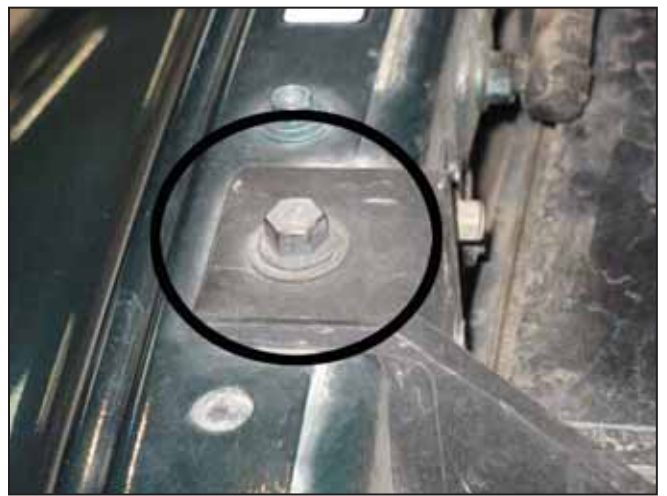
d. Remove the grommets from the plastic battery-tray. Remove the bolt securing the battery tray to the fender.
