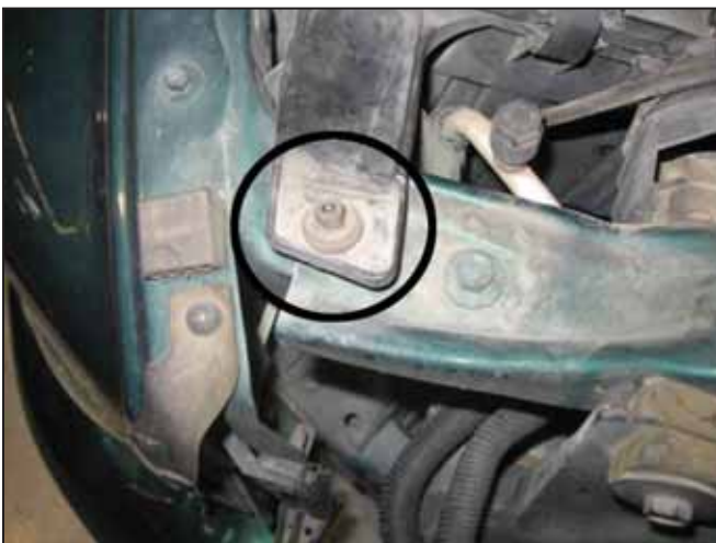
c. Remove the nut securing the front of the air filter housing to the chassis. Lift up on the air filter housing and remove it from the engine bay.
