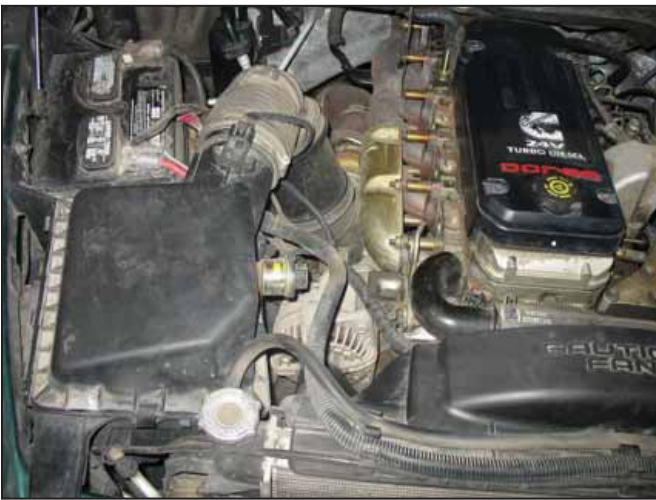
Factory airbox system installed
