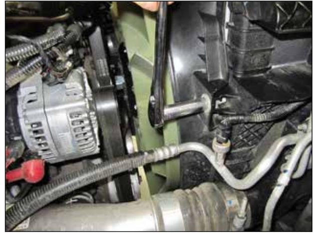
f. Remove the 13mm bolt on the fan shroud.
