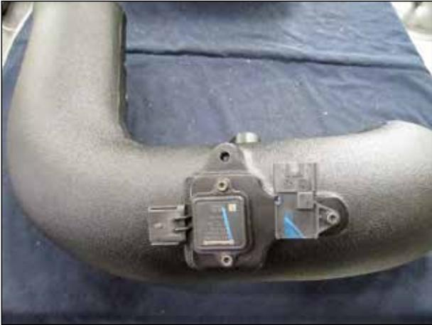
b. Using the bolts(1-2097), secure the MAF and IAT sensors(1-2109) to the AEM intake tube as shown.
