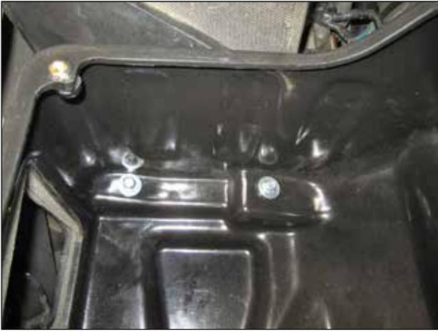
n. Install the other 6mm bolt(1-2038) with the 6mm washer(08160).
