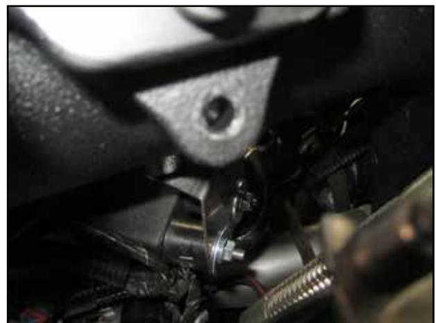
s. Now install the 6mm nuts(444-460-04) and 6mm washers (08160) on the rubber mounts holding the intake bracket to the air box.
