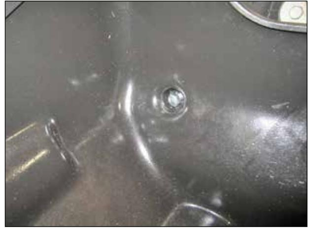
o. Install the 8mm bolt(1-2080) through the front of the air box into the radiator support; you may need to adjust the fan shroud to get the bolt in.
