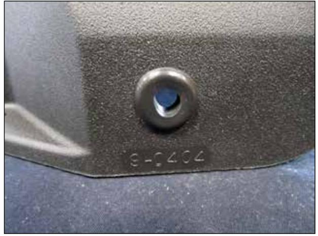
u. Install the rubber grommet(784642) into air box lid(9-0404).
