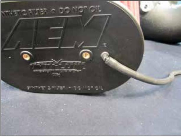
h. Install the hose(5-3015) on the 90 Degree fitting.
