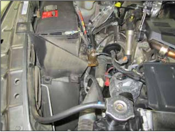
e. Lift up on the air box and remove the intake system from the vehicle.
