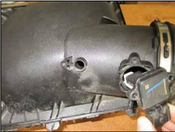
g. Remove the MAF sensor and IAT sensor from the OEM intake system.
