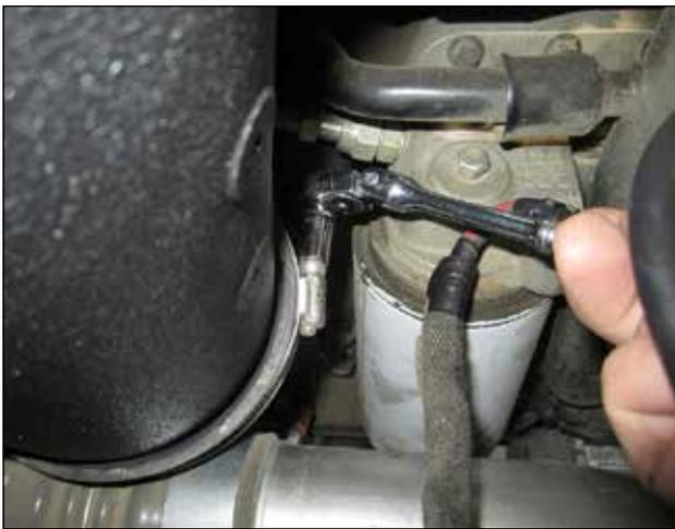
bb. Adjust the intake tube for maximum clearance and tighten the hose clamp on the turbo coupler to the AEM intake tube.
