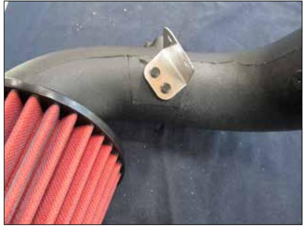
i. Install the intake tube bracket(32-3057) on the AEM intake tube(9-82211) as shown using the provided 6mm bolts(1-2110).
