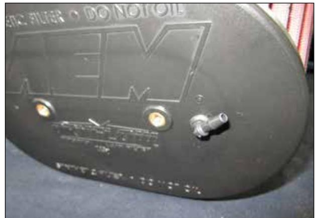
e. Install the 90 degree fitting(8-152) into the grommet on the filter.
