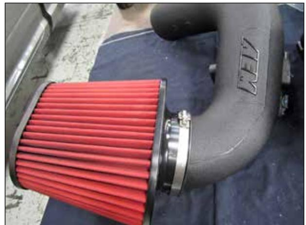
g. Now install the AEM filter and hose clamp (103-BLO-8020N) on the intake tube as shown.
