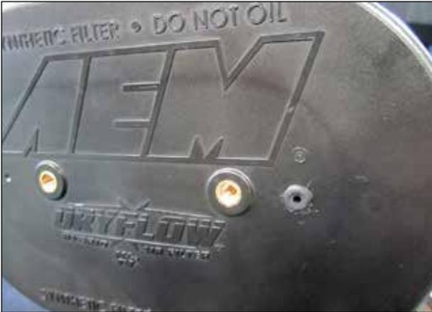
d. Install the rubber grommet(784631) in the ¼ diameter hole.
