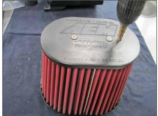
c. Drill a ¼ diameter hole in the plastic cap of the AEM filter at the dimpled location as shown, Clean out all plastic shavings from inside the filter.
