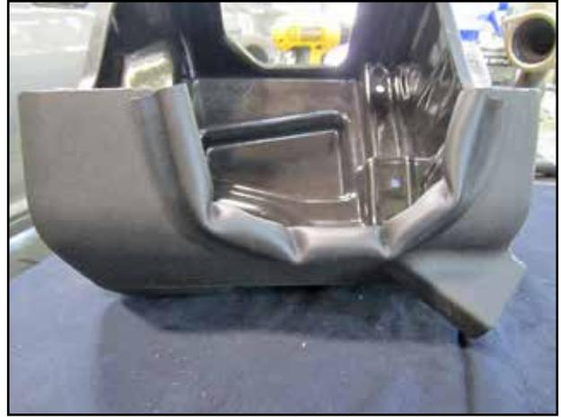
k. Install the rubber edge trim(8-4012) on the lower air box.
