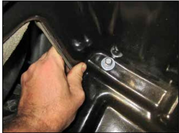
m. Set the lower AEM air box(9-0418) in place and squeeze the OEM foam as shown, to allow for the air box to sit in place. Install the 6mm bolt(1-2038) and 6mm washer(08160).
