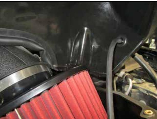
x. Install the filter minder hose on filter minder from step (h)
