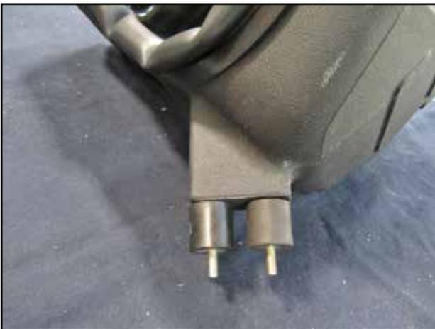
l. Install the 2 rubber mounts(1228599) on lower air box(9-0418).
