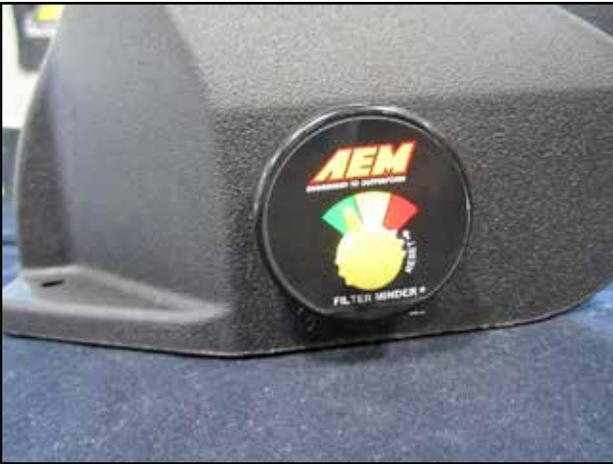
v. Now install the AEM filter minder(35-80321) into the grommet installed in step (u).
