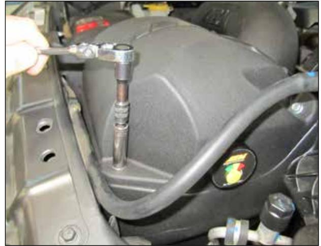
aa. Install and tighten the four 6mm bolts(1-2038) for the air box lid.
