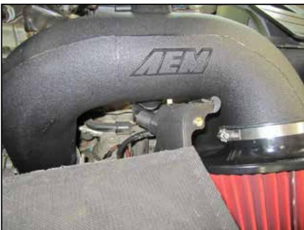
r. Install the AEM Intake tube in the turbo coupler and air box. Plug in MAF and IAT sensors.
