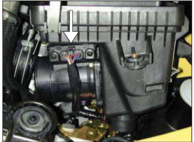
f. Disconnect the MAF sensor harness from the bottom portion of the air box. Carefully remove the bottom portion of the air box. The honeycombs in the MAF sensor are sensitive, take note not to damage during removal.
