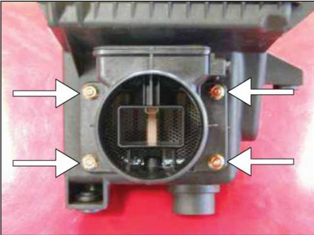
g. Carefully remove the 4 bolts holding the MAF sensor to the bottom portion of the air box. Check the MAF sensor gasket for tears or cracks. Replace as necessary.
