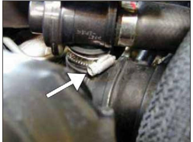
h. Loosen the hose clamp connecting the blow off valve to the turbo inlet hose. Disconnect the blow off valve from the inlet hose. Remove hose clamp from the inlet hose.
