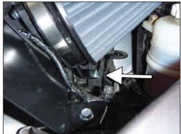
o. Attach the air filter and MAF sensor assembly to the inlet pipe. Line up the bracket to the rubber mount. Refer to the diagram on the next page.
