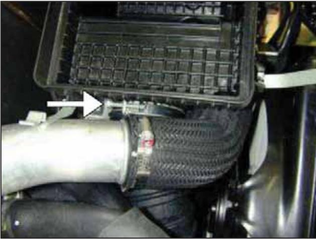
e. Loosen the hose clamp connected to the bottom portion of the air box.
