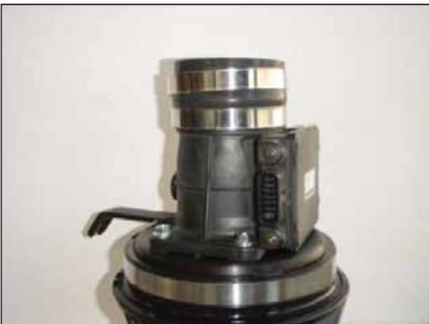
n. Attach the coupler to the MAF sensor. Attach the provided hose clamps to the coupler as shown. Do not fully tighten. You may need to add a very small amount of lubricant to slide the coupler over the sensor for easier installation.
