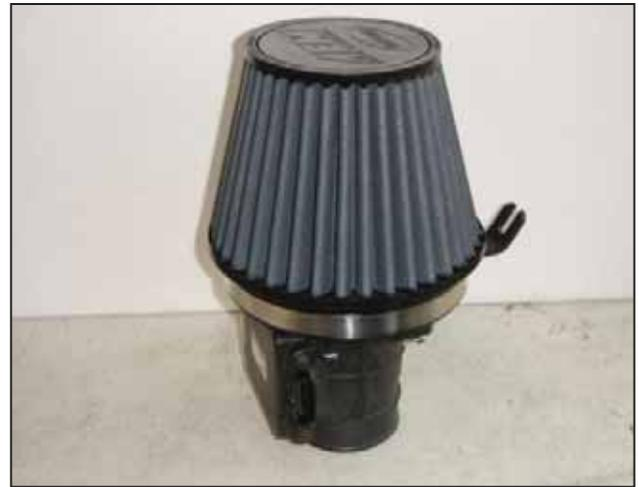
m. Attach the filter element to the MAF sensor and secure with provided hose clamp.
