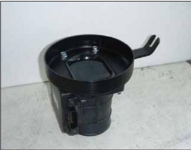
l. Assemble the MAF sensor adapter to the MAF sensor with the provided M6 nuts and M6 bolts.
