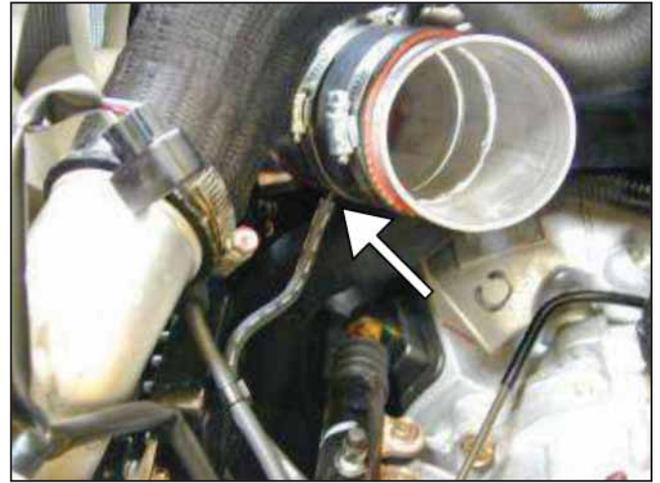
k. Attach vacuum line from the boost solenoid to the vacuum nipple underside of the pipe.
