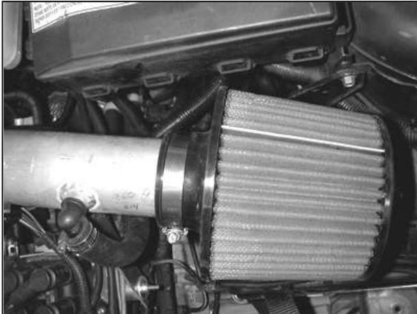
i. Install the AEM<sup>®</sup> air filter onto the intake pipe and secure with the supplied hose clamp.
