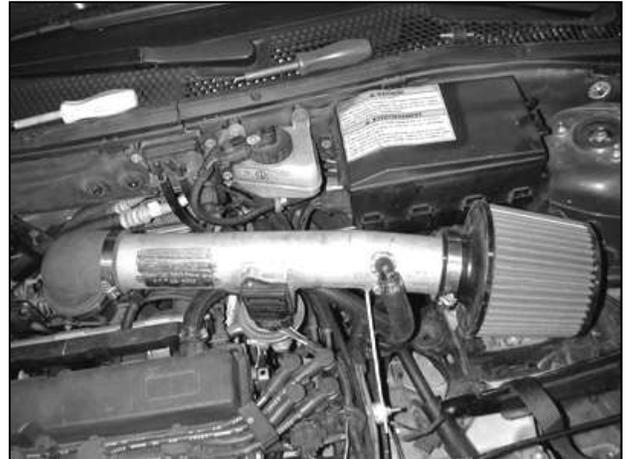
AEM<sup>®</sup> intake system installed
