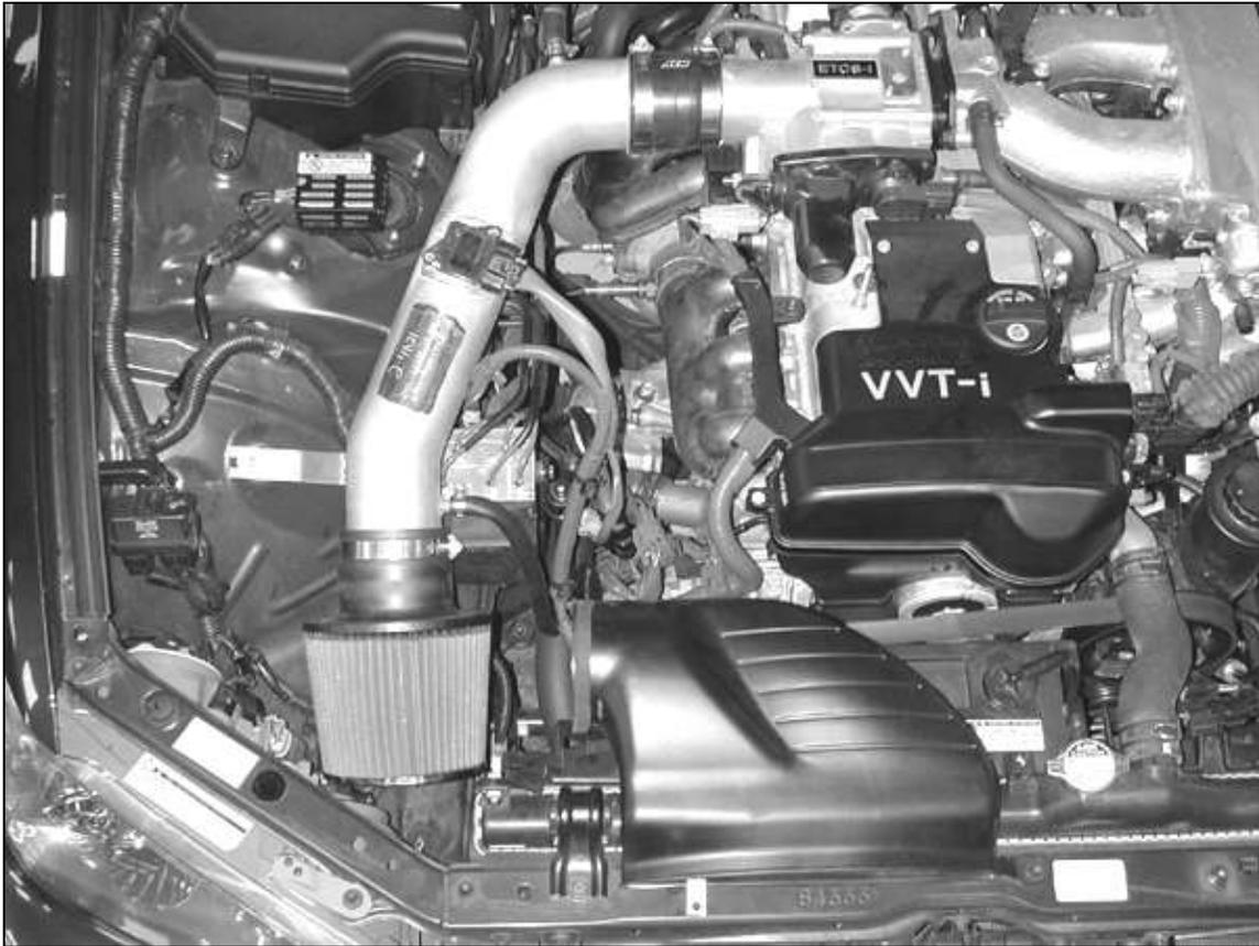
AEM® intake system installed
