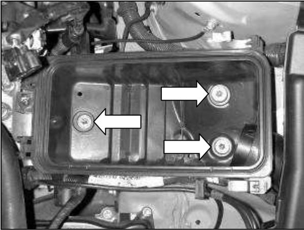
l. Remove the three bolts retaining the lower air box. Remove the lower air box from the vehicle.
