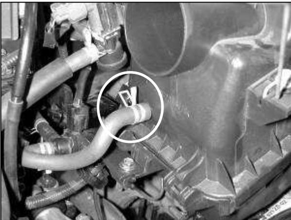
f. Remove the large vacuum line from the engine side of the air box lid.
