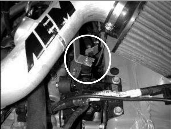
k. Install the AEM® intake pipe into the engine bay with the air filter already installed. The intake bracket should line up with the rubber mount. Loosely secure the bracket to the rubber mount with the supplied M6 washer and lock nut. Refer to the diagram above for proper rubber mount installation.
