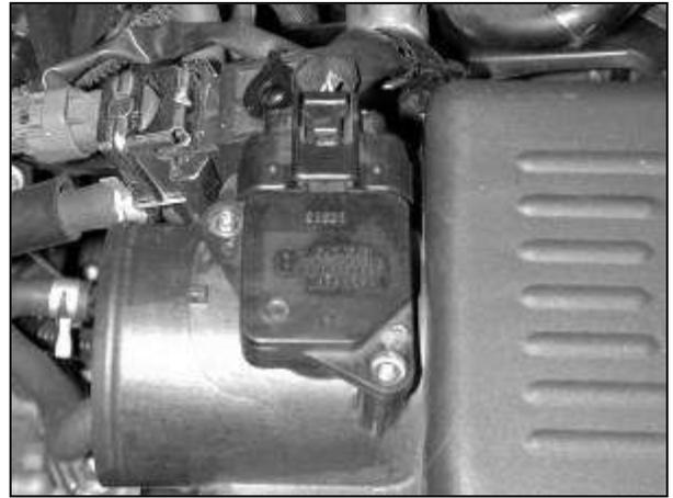
e. Remove the air flow meter connector from the sensor. Remove the two small screws and remove the sensor from the air box. Use care when removing this component, as it can be easily damaged. Set the air flow meter aside in a safe place.
