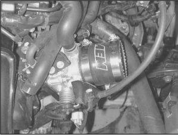
i. Place the supplied silicone hose on the throttle body. Loosely secure the hose with the two supplied 2.75" hose clamps.
