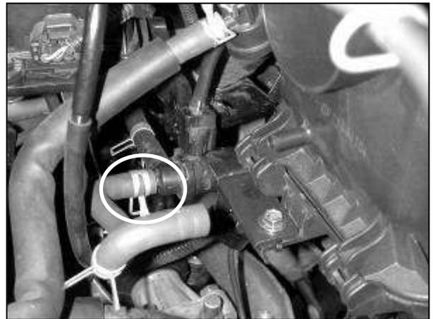
g. Remove the other side of the large vacuum line from the VSV mounted to the air box. Keep both vacuum line spring clamps; they will be reused with the AEM<sup>®</sup> intake system.
