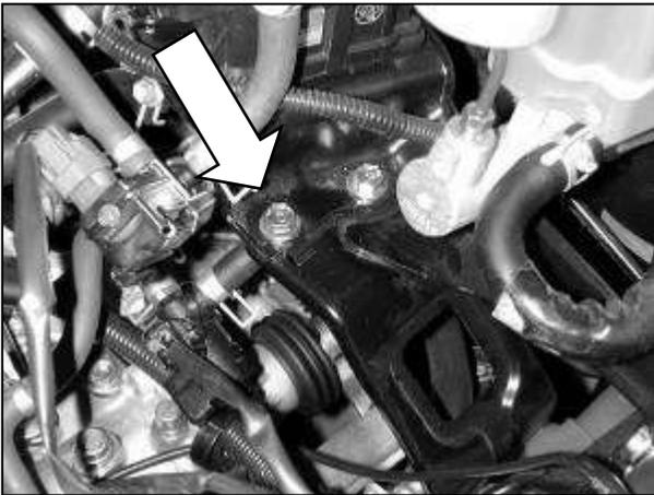
c. Remove the forward-most M8 bolt from the black bracket under the brake master cylinder.
