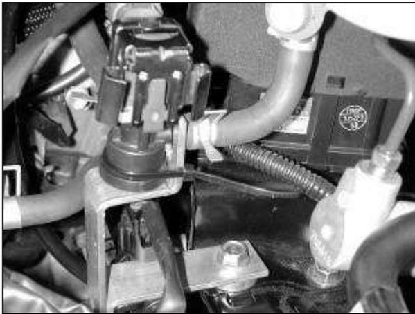
g. Use one of the supplied zip ties to secure the upper VSV to the bracket. Make sure the zip tie rests in the notches in the bracket to ensure that it does not slide off.
