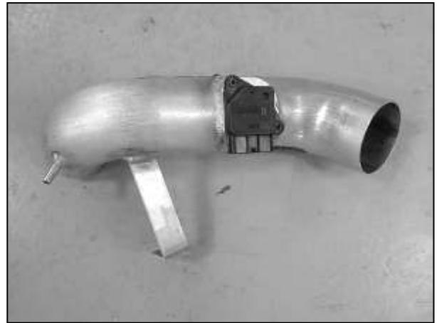
h. Mount the MAF sensor to the adaptor on the underside of the AEM® intake pipe using the two supplied 8-32 cap screws.
