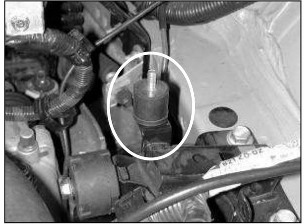
j. Install the supplied rubber mount onto the metal lower air box bracket. See diagram below for proper rubber mount installation.
