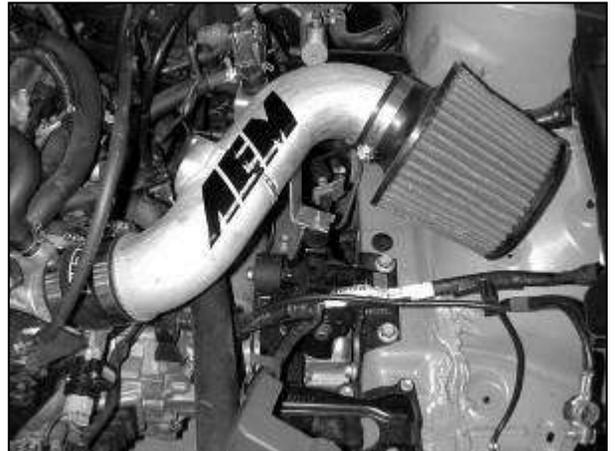
l. Install the throttle body end of the pipe into the silicone coupler. Plug in the MAF sensor on the back side of the pipe.
