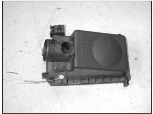
i. Remove the air box lid from the vehicle.
