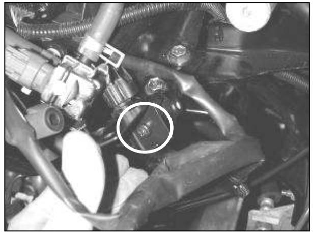
k. Remove the phillips head screw that secures the metal bracket to the VSV. This bracket will not be reused with the AEM<sup>®</sup> intake system.
