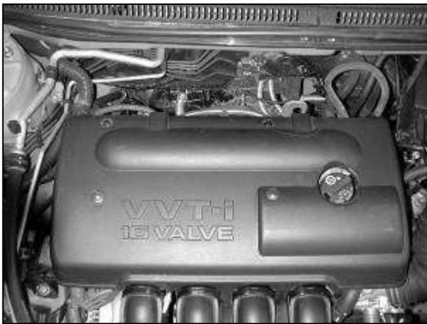
b. Remove the two nuts and two plastic rivets that hold the plastic engine cover on. The plastic rivets may be gently lifted with a small screwdriver. Remove the engine cover.
