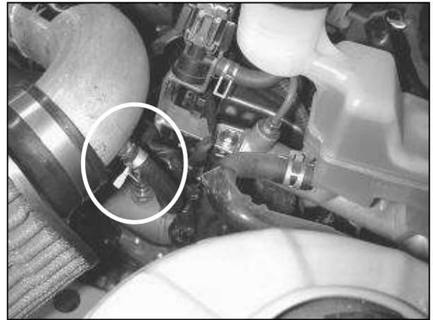
n. Use the other stock spring clamp on the intake pipe side of the 5/16" vacuum hose. Route the hose carefully to avoid kinks.
