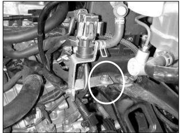
f. Use the supplied M8 bolt to secure the assembly to the bracket beneath the master cylinder. Be sure that the spacer remains in place. Rest the upper VSV on the bracket as shown. The rear vacuum line may need to be pulled back slightly to clear the bracket.
