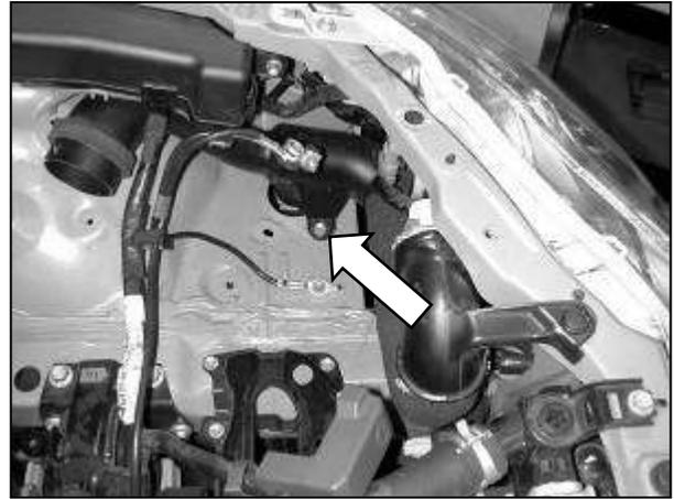
m. Remove the stock intake air duct from the engine bay. The duct is retained by one bolt and one plastic rivet. Pry the center of the plastic rivet up with a small screwdriver; the entire rivet should pull out.
