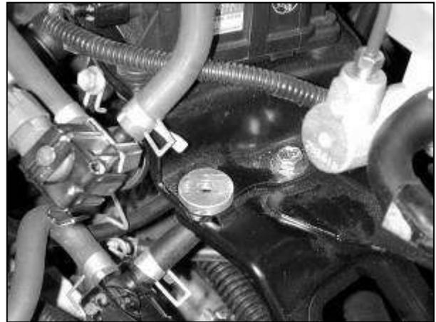
d. Place the supplied VSV bracket spacer in-line with the hole exposed in the previous step.
