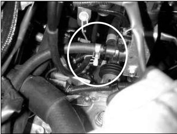
m. Replace the vacuum line removed in step 2g with the supplied length of 5/16" vacuum hose. Reuse the stock spring clamp.
