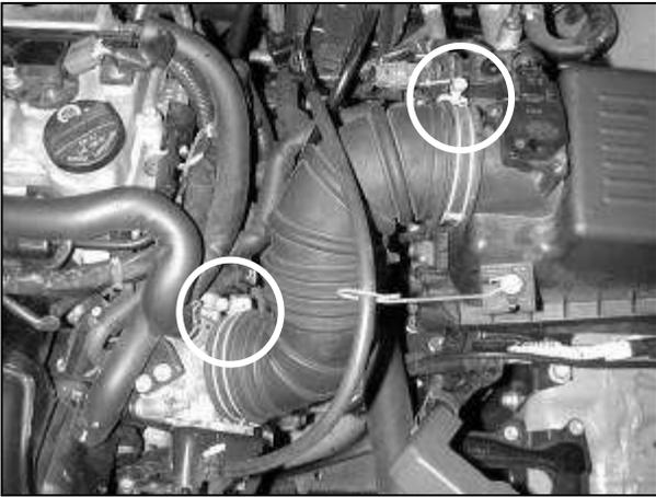
d. Loosen the two 10mm hose clamps at the throttle body and air box. Remove the stock rubber intake hose from the engine bay.
