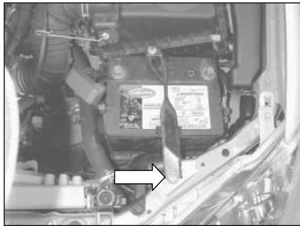
c. Disconnect the positive battery terminal. Remove the bolt on the radiator support that secures the battery bracket. Unhook the rod at the rear of the battery bracket. Remove the battery from the vehicle.
