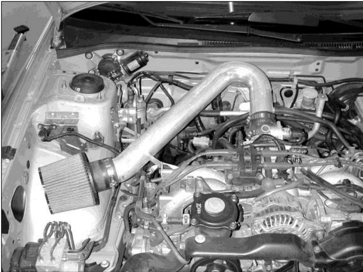
AEM® intake system installed
