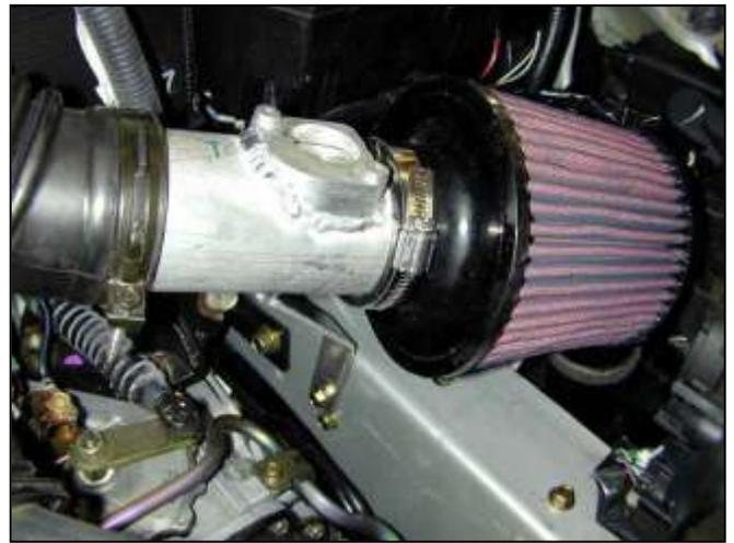
g. Insert other end of pipe into the stock inlet hose. Place mounting tab under the bolt in the frame rail.
