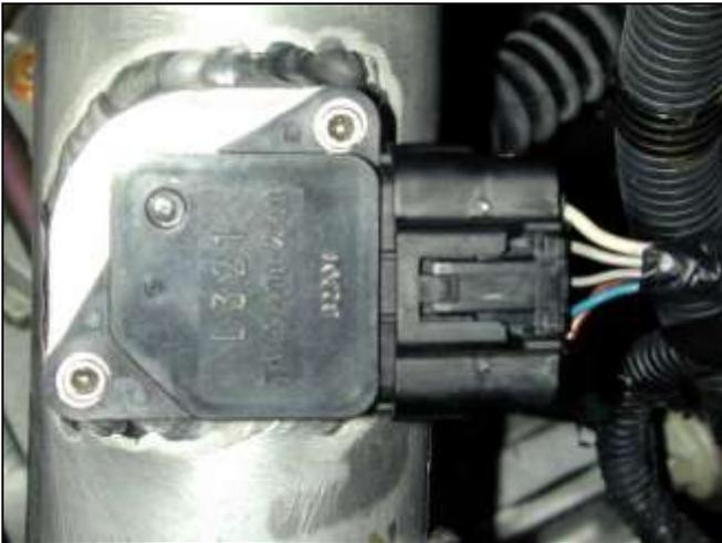
h. Install the air flow sensor into the inlet pipe utilizing the supplied screws. Plug in the air flow sensor.
