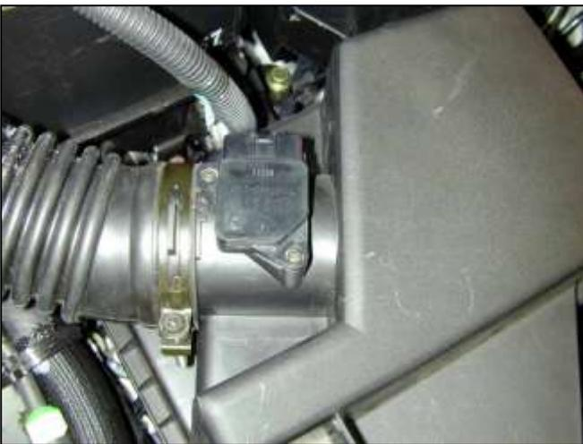
c. Release all clips and remove upper air box from vehicle. Loosen the two screws securing the MAF sensor and remove it from the air box.
