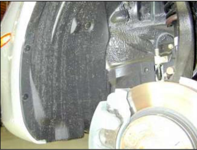
i. Raise the front of the vehicle with a jack. Refer to your owner's manual for proper jack and jack stand placement to properly support vehicle. Support your vehicle using properly rated jack stands before wheel removal or while working under the vehicle. **NEVER WORK UNDER A VEHICLE WITHOUT USING JACK STANDS.** Remove the driver side wheel. Release the plastic clips inside the fender well securing the liner.
