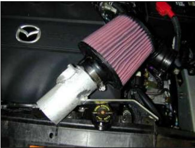
f. Install the air filter onto the end of the pipe as shown.
