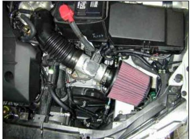
i. Check the clearance of the air filter with respect to the surrounding surfaces. Tighten the hose clamp on the inlet hose and the frame bolt.
