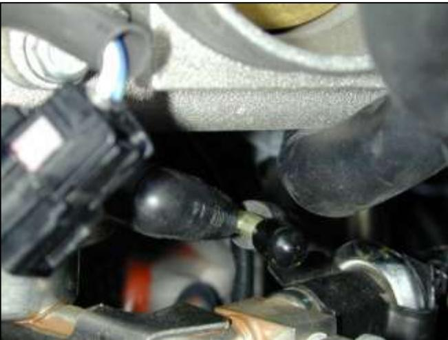
d. Install the supplied vacuum cap onto the open port on the 'T' fitting.
