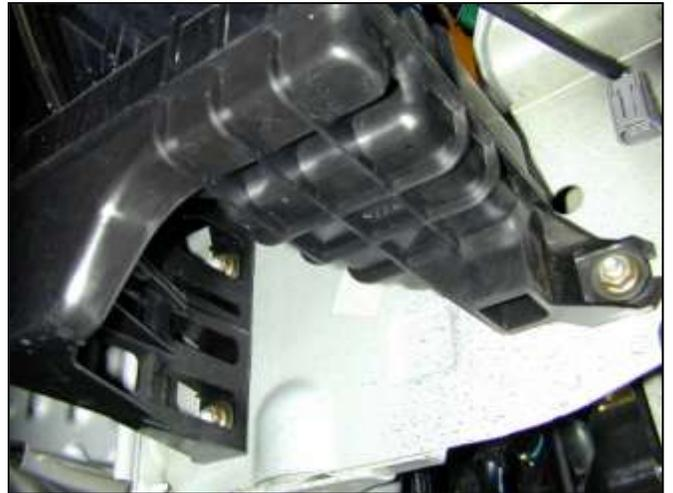
l. Release the three nuts securing the resonator box. Remove the resonator box from the vehicle.
