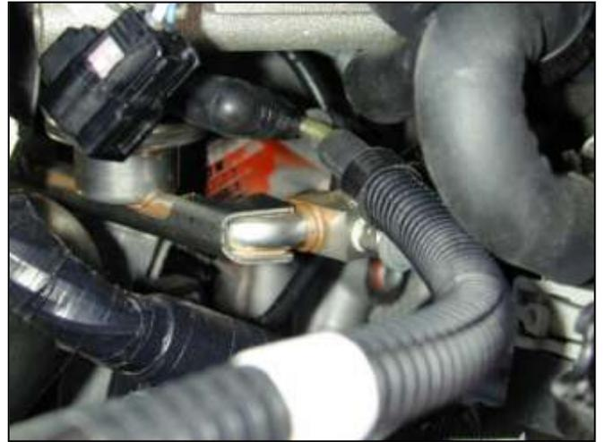
c. Follow the vacuum hose up to the 'T' fitting. Pull the vacuum hose off of the 'T' fitting. Remove the hose from the vehicle.
