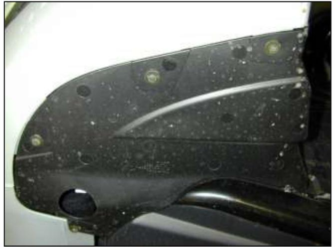
j. Remove the four screws on the bottom of the fender liner.
